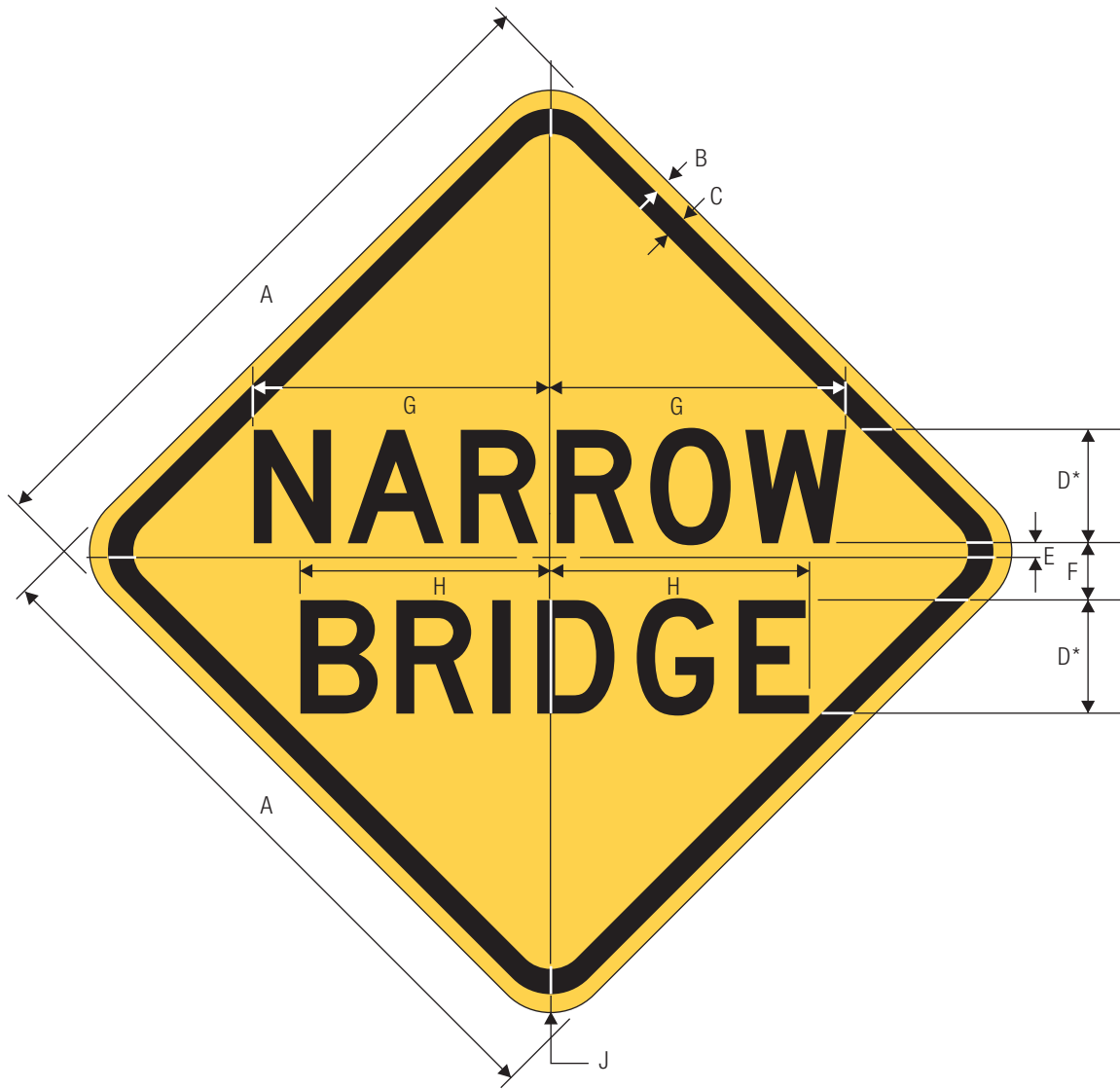
W5-2 NARROW BRIDGE
