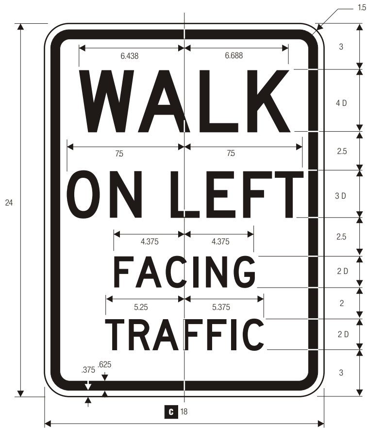
R9-1 WALK ON LEFT FACING TRAFFIC
