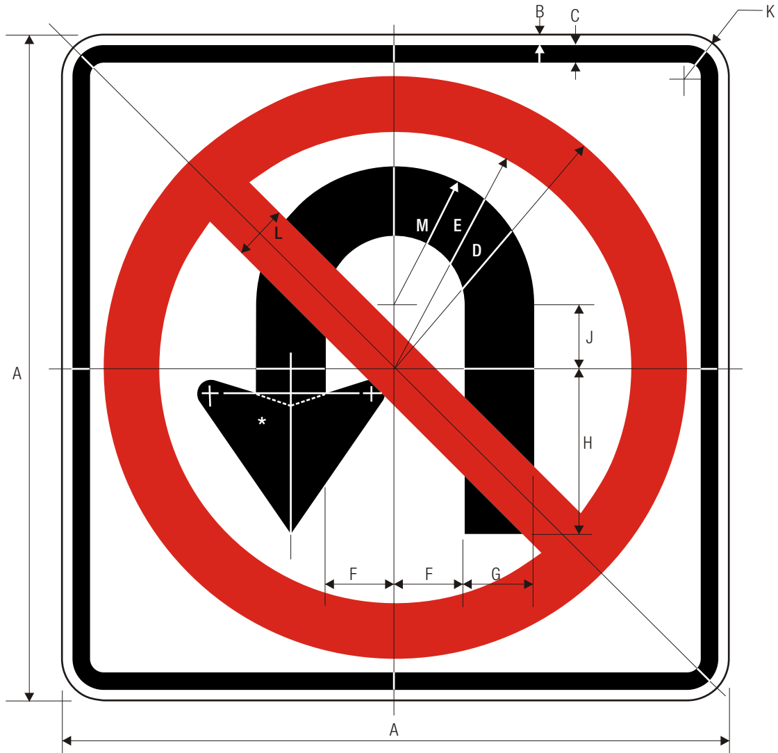
R3-4 U-TURN PROHIBITED
