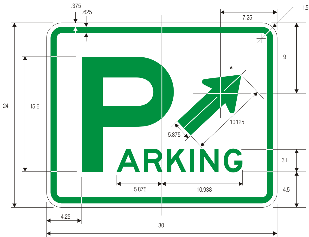
D4-1 PARKING AREA
