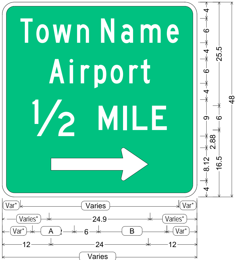
D1-103a; 3.00" Radius, 1.00" Border, White on Green; "TownName" C; "Airport" C; "1/2" D; "MILE" D; Arrow 6" Type D4 - 0°;
