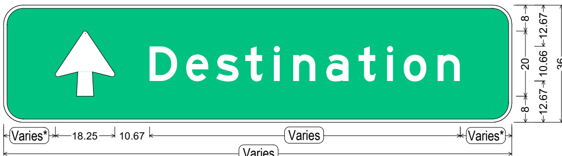
D1-1 (expressway); 6.00" Radius, 1.00" Border, White on Green; Arrow 10-13.33 Type B - 90°; "Destination" E;
