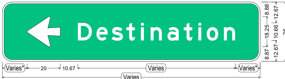
D1-1 (expressway); 6.00" Radius, 1.00" Border, White on Green; Arrow 10-13.33 Type B - 180°; "Destination" E;
