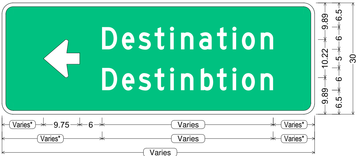
D1-1 (conventional road - 2 line); 3.00" Radius, 1.00" Border, White on Green; Arrow 6" Type D3 - 180°; "Destination" D; "Destinbtion" D;
