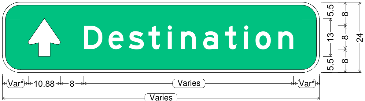
D1-1 (ramp - crossroad); 6.00" Radius, 1.00" Border, White on Green; Arrow 8" Type D1 - 90°; "Destination" E;
