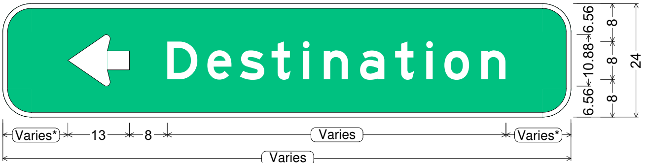
D1-1 (ramp - crossroad); 6.00" Radius, 1.00" Border, White on Green; Arrow 8" Type D1 - 180°; "Destination" E;
