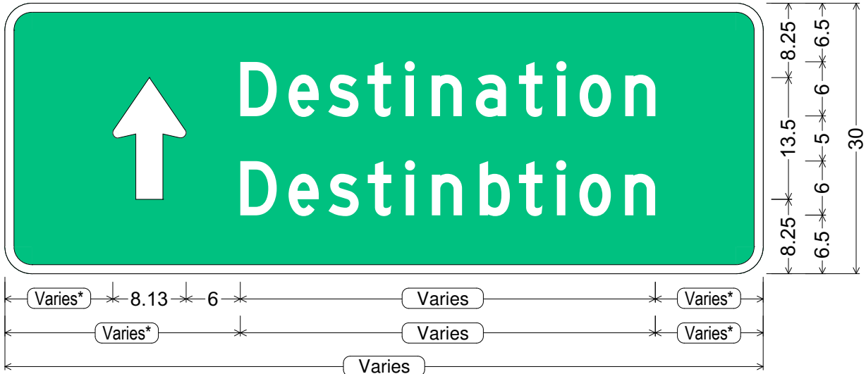
D1-1 (conventional road - 2 line); 3.00" Radius, 1.00" Border, White on Green; Arrow 6" Type D2 - 90°; "Destination" D; "Destinbtion" D;
