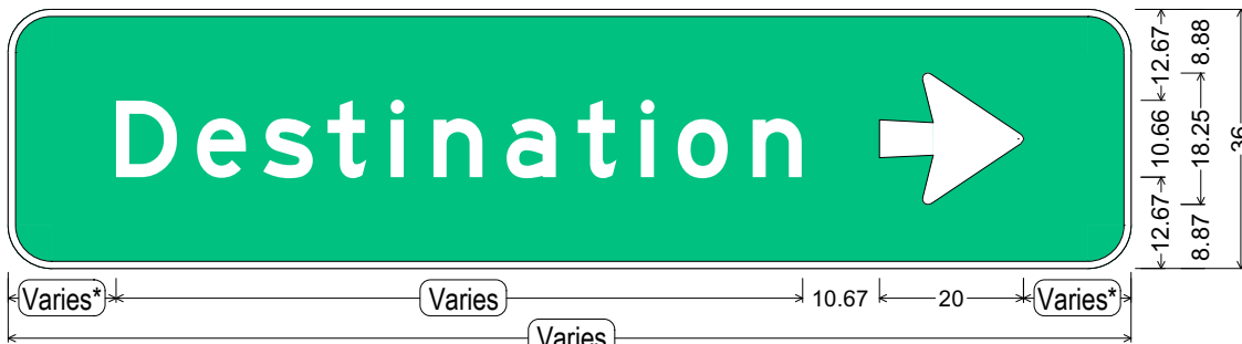
D1-1 (expressway); 6.00" Radius, 1.00" Border, White on Green; "Destination" E; Arrow 10-13.33 Type B - 0°;
