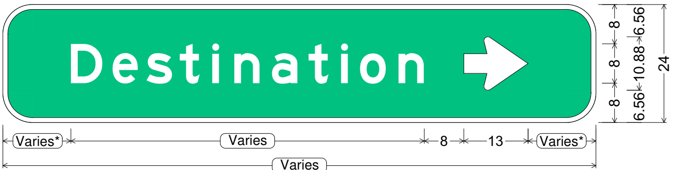
D1-1 (ramp - crossroad); 6.00" Radius, 1.00" Border, White on Green; "Destination" E; Arrow 8" Type D1 - 0°;
