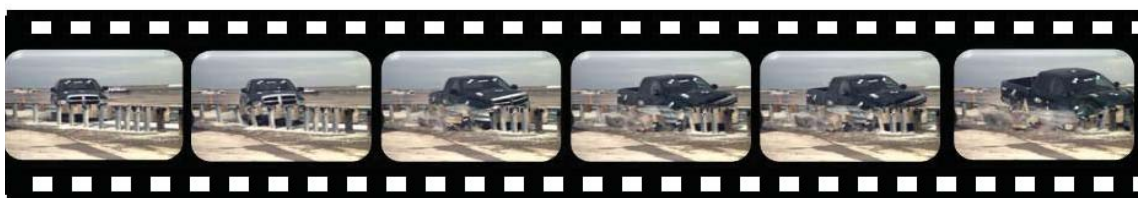
MASH TL-3 Test of MGS Transition to Thrie-beam
