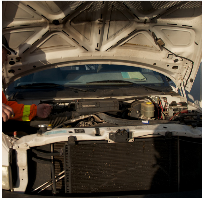
Use drip pans or absorbent pads under equipment during staging and maintenance that involves fluids.
