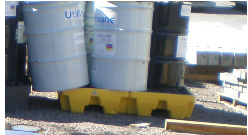
Drums and materials on containment pallets (designed for 40 CFR compliance) are only useful when materials are centered and the capacity is not exceeded.
