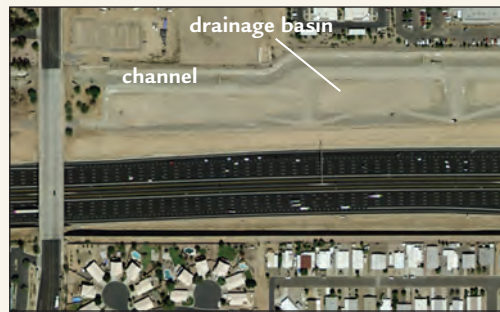
Narrow parallel retention basin
