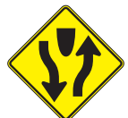
Start of Divided Highway
