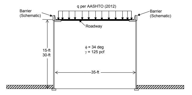
Note: Incorporate the presence of barriers in the design in terms of impact loading. Use ADOT 42inch barrier detail as shown in ADOT Standard Drawing No. SD-1.02. Use Test Level-5 (TL-5) loading as per Table A13.2-1 in AASHTO (2012).
