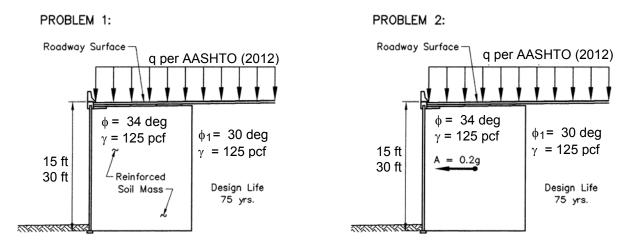
Note: For Problems 1 and 2, incorporate the presence of barriers in the design in terms of impact loading. Use ADOT 42-inch barrier detail as shown in ADOT Standard Drawing No. SD-1.02. Use Test Level-5 (TL-5) loading as per Table A13.2-1 in AASHTO (2012).
