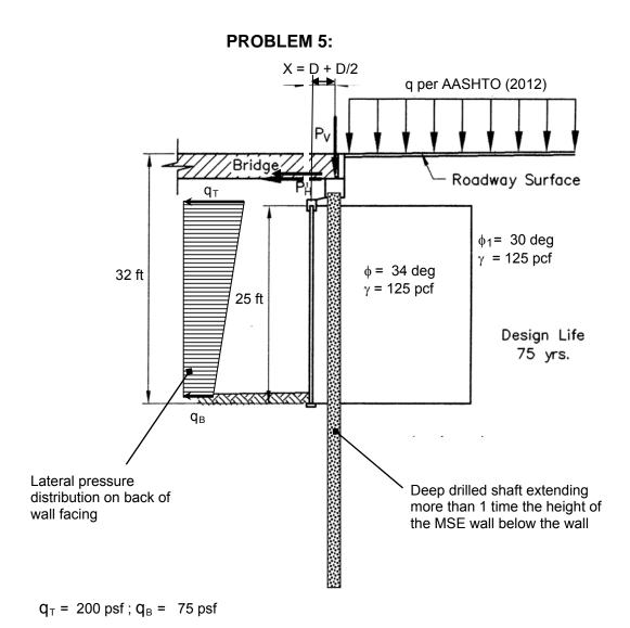
Note: X is measured from the back-face of the facing unit to the center of the drilled shaft.
