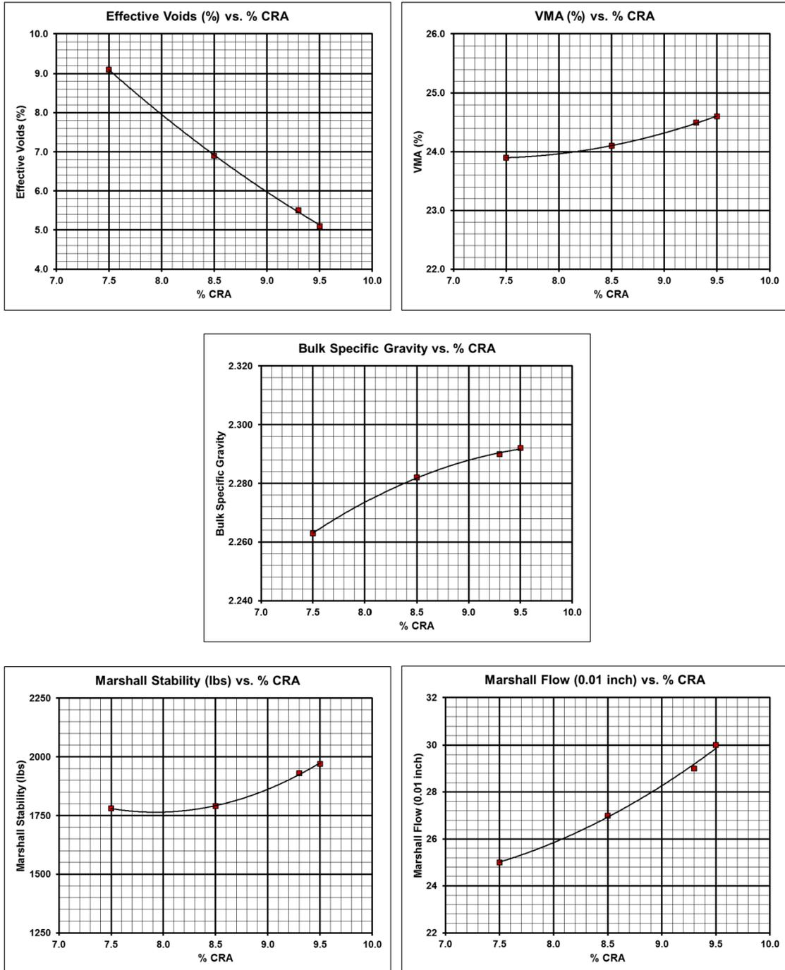
The above graphs are for illustrative purposes only. Straight-line interpolation, as specified in Subsections 11.3 and 11.3.1, is used for mix design calculations.
