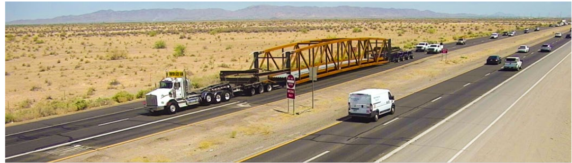
Traveling from Coolidge to San Francisco, this bridge section cargo on State Route 347 was more than 221 feet long and 18 feet wide, and categorized as a "super load" by the statewide permits office.
