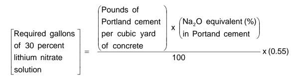
(e) The coarse aggregate and the fine aggregate shall be tested separately in accordance with ASTM C 1260 to determine the potential for alkali silica reaction (ASR). When aggregates show the potential for ASR, as indicated by expansions of 0.10% or greater at 16 days after casting, sufficient mitigation for the expansion shall be determined in accordance with ASTM C 1567. The use of fly ash or natural pozzolan may exceed 25 percent, by weight of the cementitious material.
