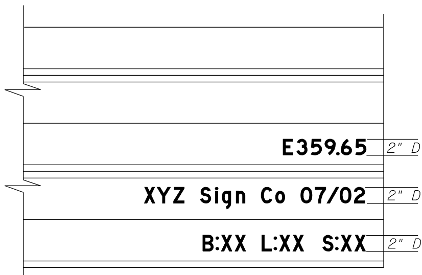
LETTERING FOR BACK OF EXTRUDED AND FLAT SHEET GUIDE SIGN PANELS (BLACK)
