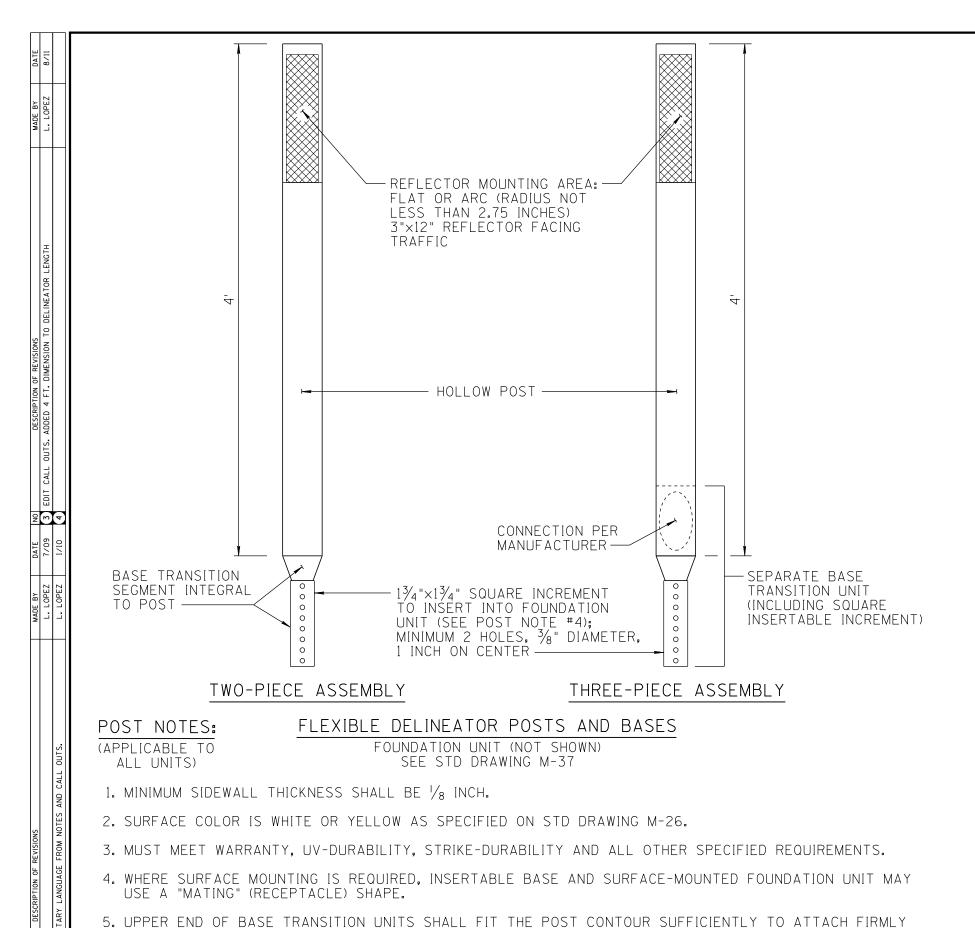
6. LOWER END OF BASE TRANSITION SEGMENTS AND BASE TRANSITION UNITS SHALL BE SHAPED AND SIZED
