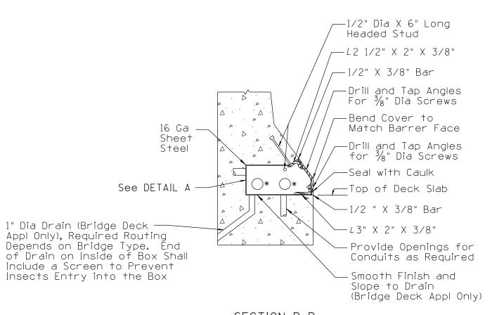
SECTION B-B \* Conduit Placement As Needed
