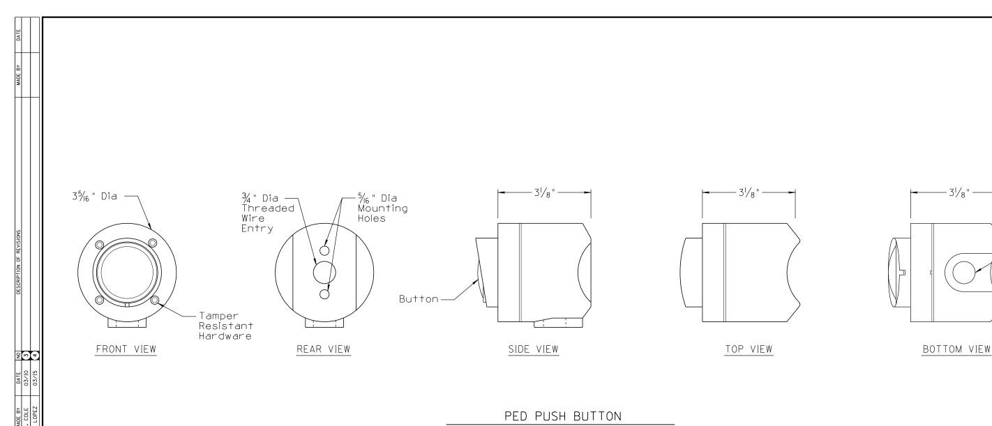
(Note: Push Button shall conform to all applicable requirements of T.S. 11-1. The exact configuration can vary as long as the same function is achieved.)
