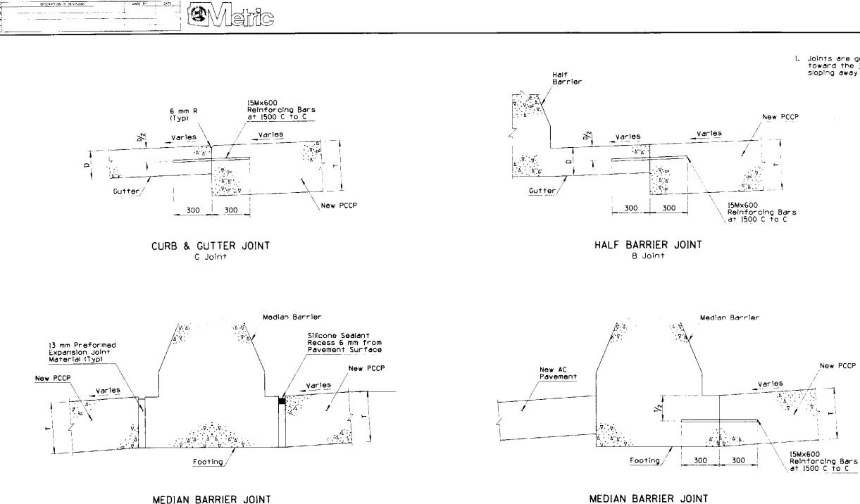
B Joint PCCP On Both Sides of Barrier
