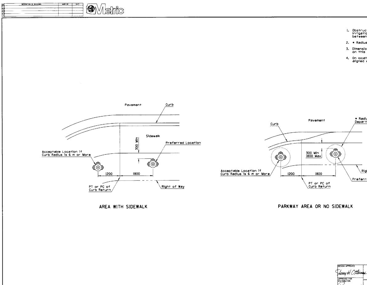
Obstructions such as utility poles, street signs, irrigation boxes, fences, etc., must not be placed between curb and hydrant.
