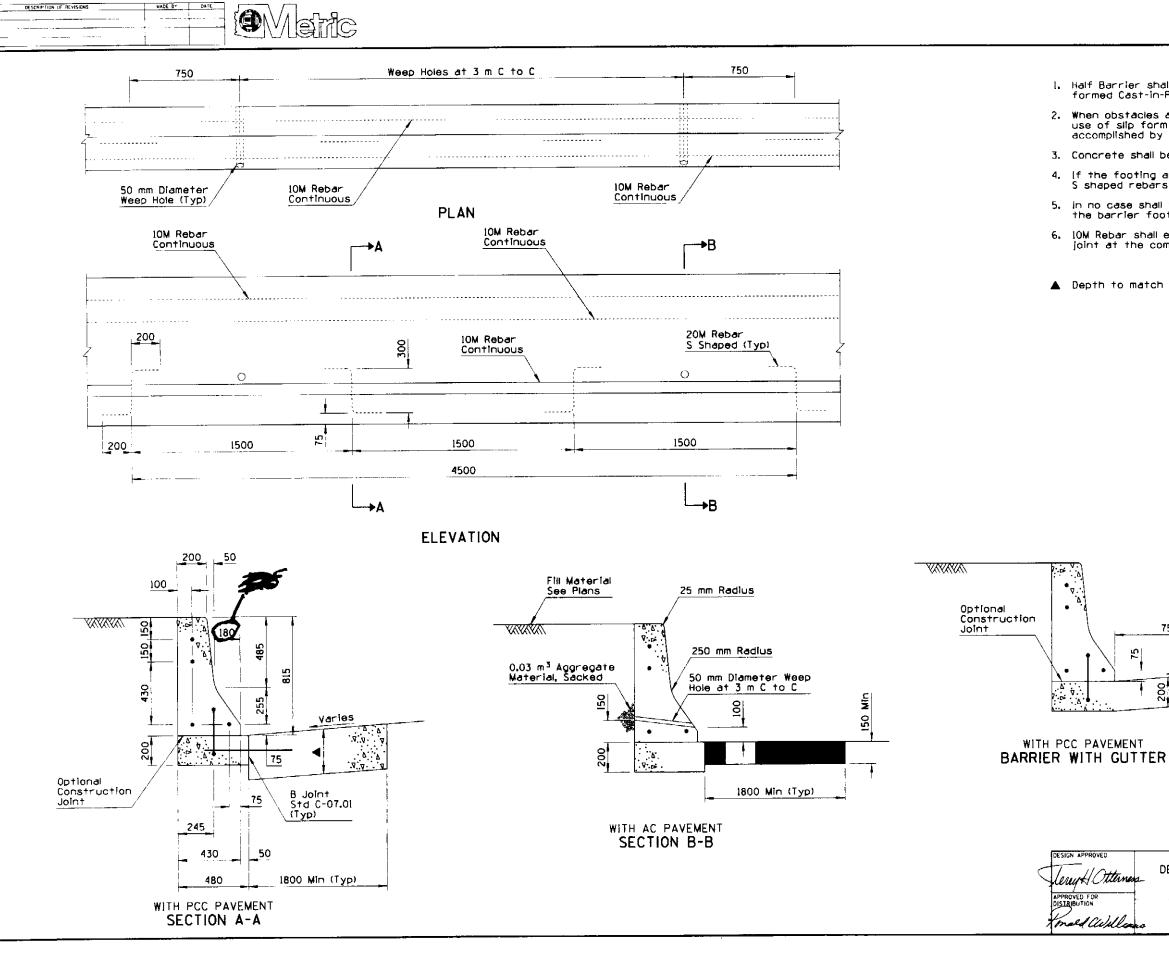
Half Barrier shall be constructed by the slip form or formed Cast-in-Place method.
