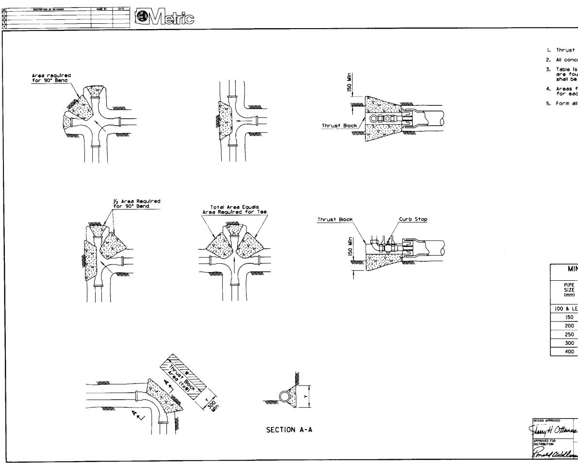
1. Thrust blocks are to extend to undisturbed ground.
