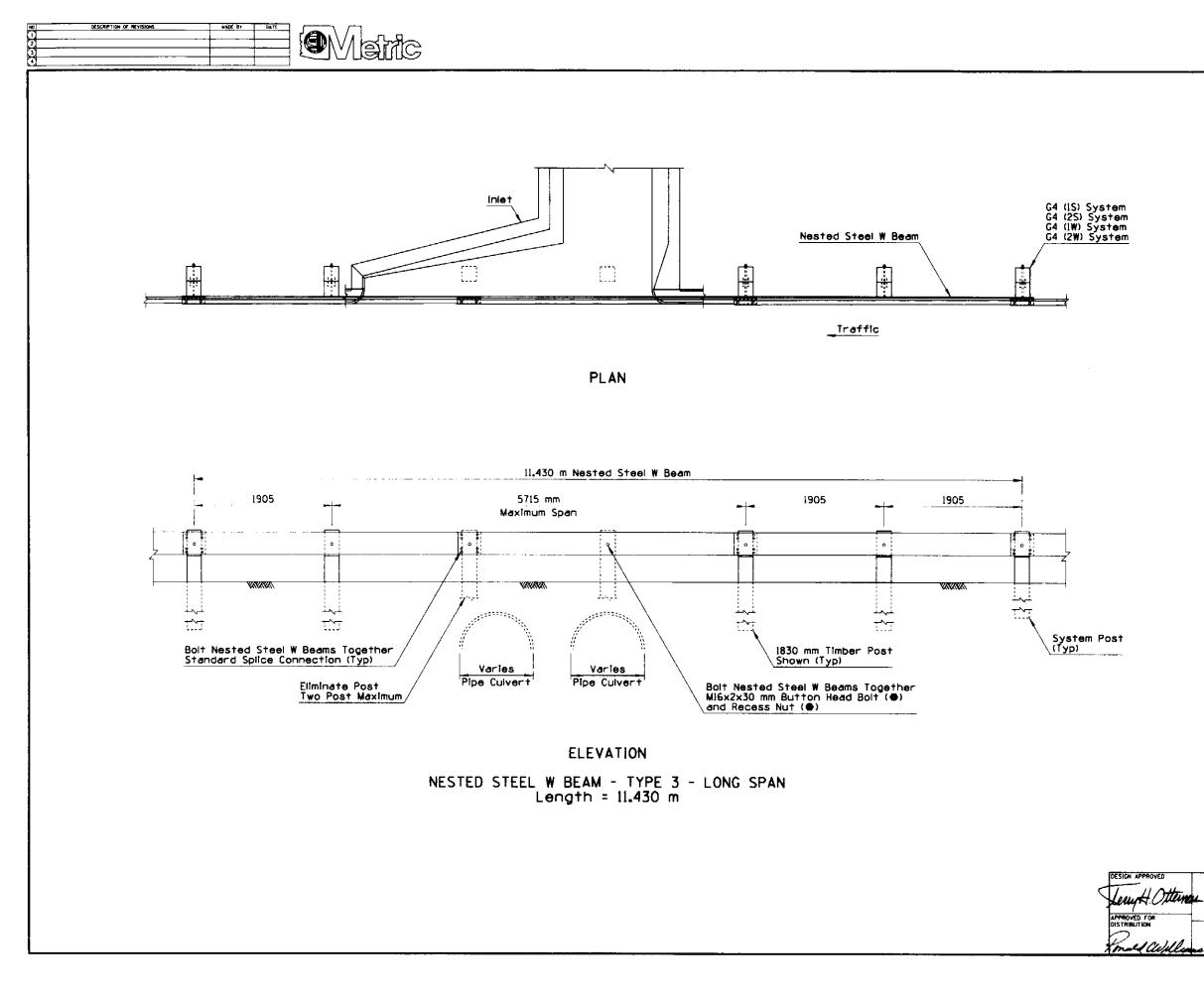
Use Type 3 Nested Steel W Beam to span downdrain or spillway inlets as shown in the plan view.
