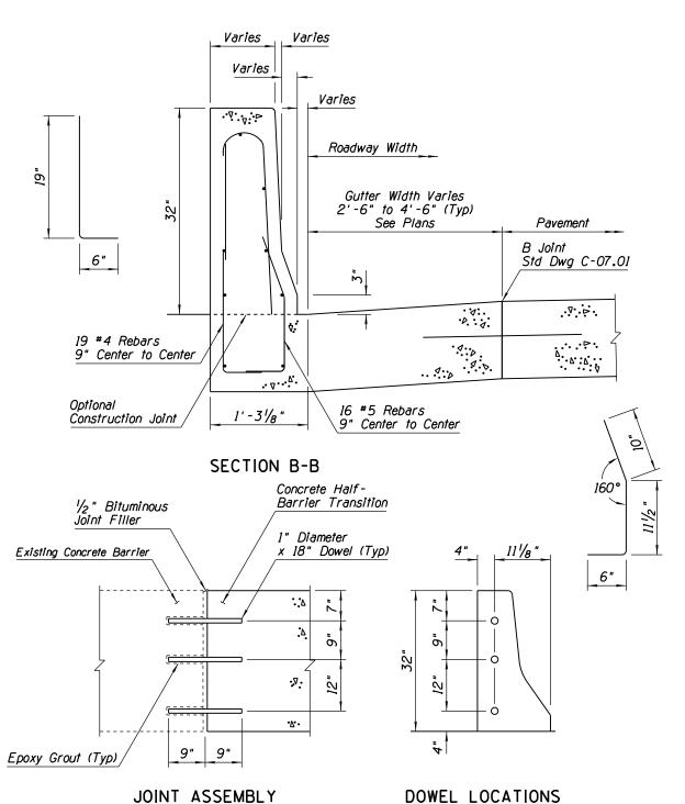
CONSTRUCTION JOINT DETAIL (OPTIONAL)
