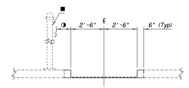
**ELEVATION** DEPRESSED CURB AT SIDEWALK RAMP
