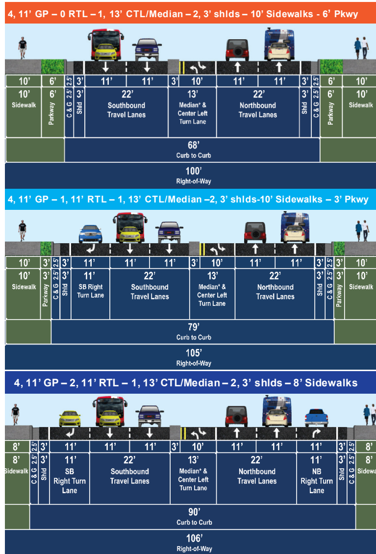
Figure 4-2: Short-Term Recommended Cross Section: Forest Meadows Street to Route 66
