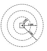
typically consists of two or more layers of air space and is designed to contain all published instrument approach procedures to the airport. An air traffic control clearance is required for all aircraft to operate in the area.
