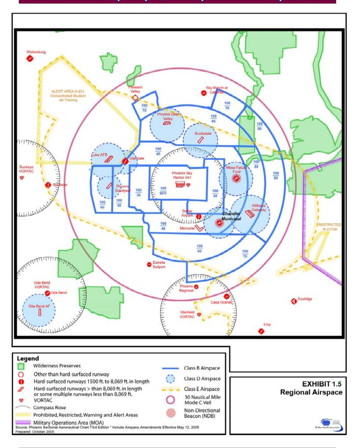
Through Federal Aviation Regulations (FARs), airspace classifications have been developed to promote the safe and efficient movement and control of aircraft during flight and approach/departure procedures. Airspace classifications are identified on sectional aeronautical charts published by the FAA's National Aeronautical Charting Office. FAR Part 71 and FAR Part 73 establish classifications of airspace with the following characteristics:
