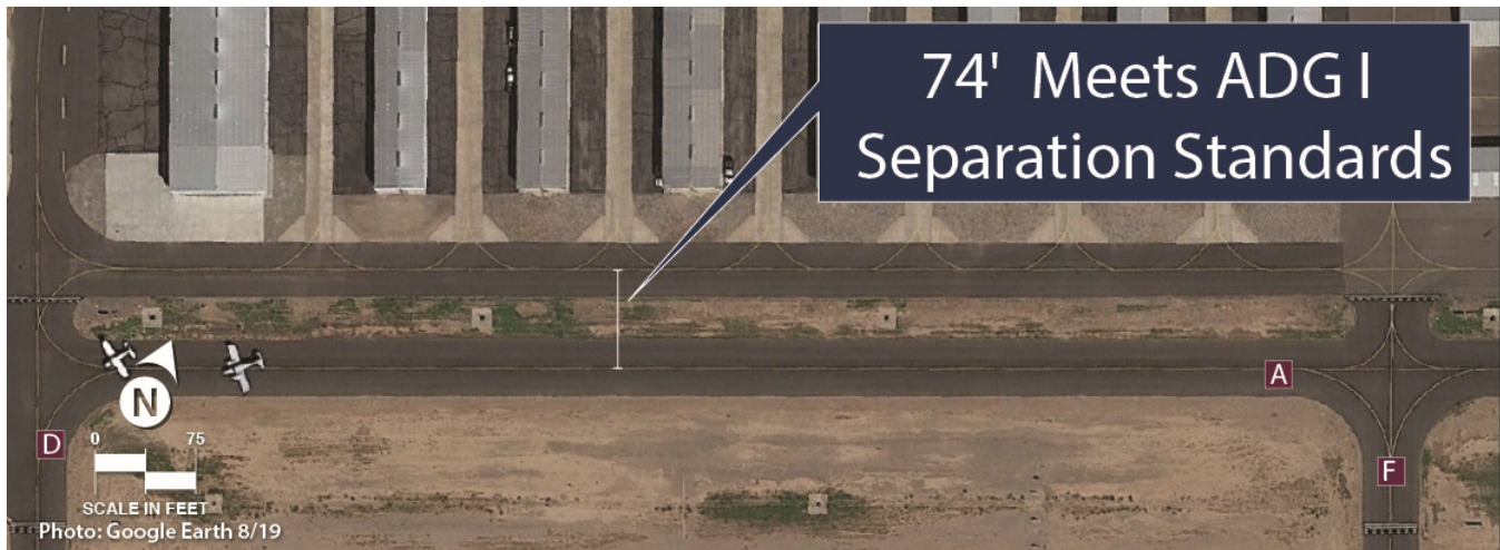
FIGURE 3A – ADG I TAXIWAY CENTERLINE SEPARATION AREA
