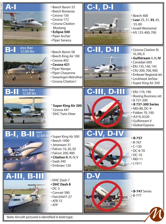
Exhibit 2D AIRPORT REFERENCE CODES In the long range, the forecast traffic will warrant the development of a parallel runway. The separation between the centerlines of the two paved runways should be at least 700 feet. The parallel runway should be of sufficient design to accommodate on the order of 90 percent of the aircraft types using the airport. As a result, it should ultimately be planned to ARC B-II.
