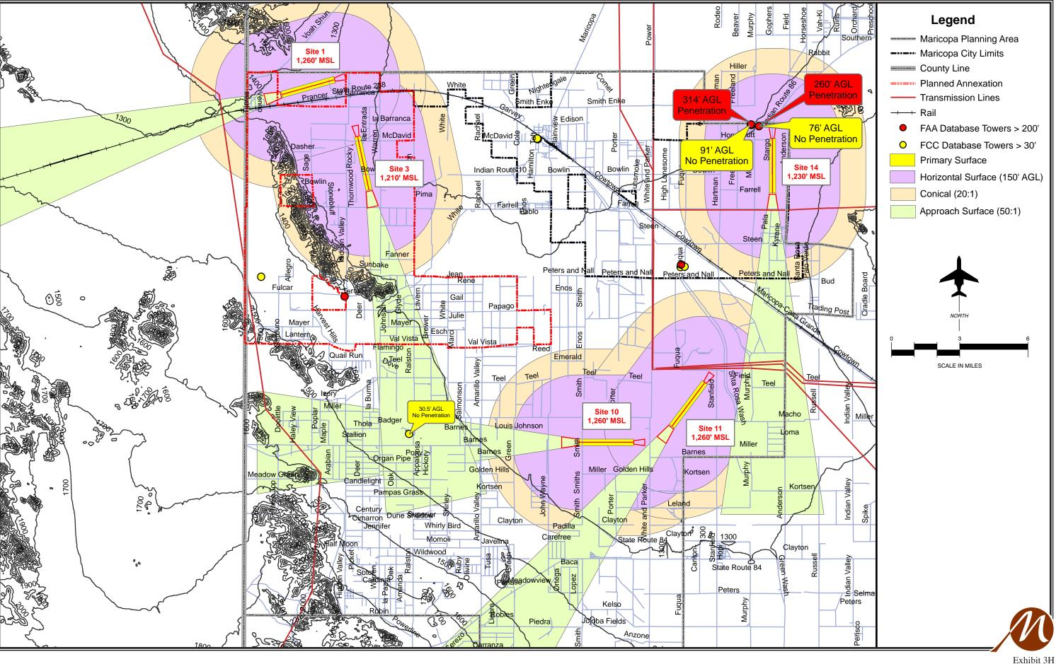
OBSTRUCTION CONSIDERATION CANDIDATE SITES clear of obstruction. Site 3 would have a terrain penetration to CAT I approach slope from the south. This would potentially raise the instrument approach minimums for the airport.
