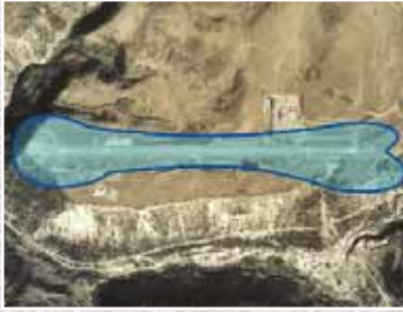
The 65 DNL contour defines a noise impact envelope which encompasses all of the area within which significant sleep disturbance may be expected.
