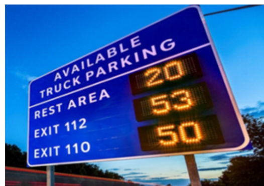
Figure 9: Example Dynamic Parking Capacity Sign
