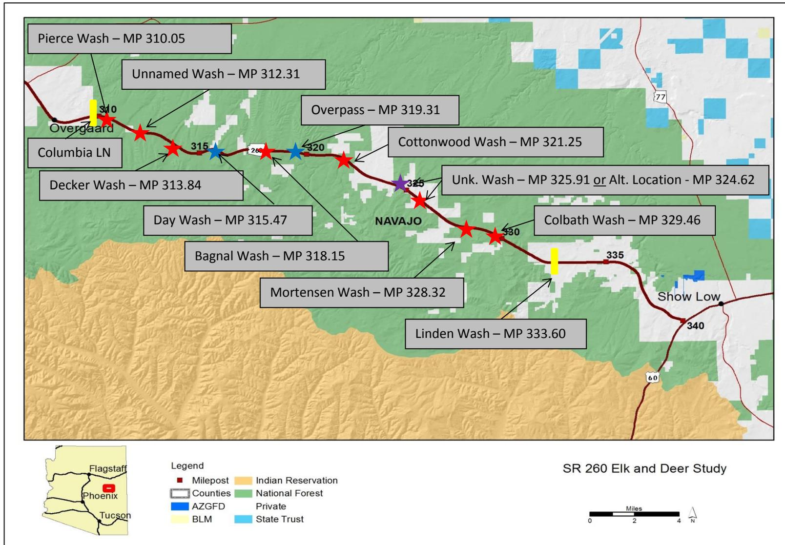
**Figure 49. Recommended Specific Locations of Wildlife Crossings and Fencing from Overgaard to U.S. 60. Red and Blue Stars Mark Underpass, Overpass, and Alternate Locations, Respectively, and Yellow Bars Mark Proposed Fence Ends**
