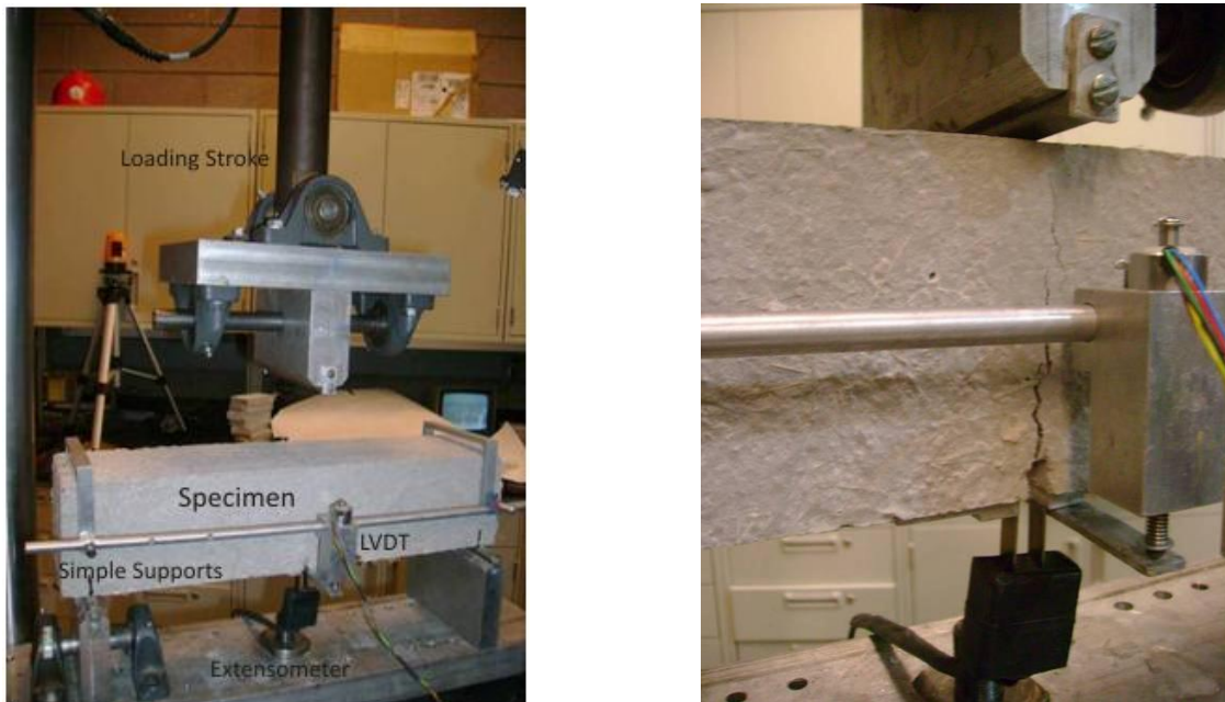
Figure 6. a) Closed-Loop Flexural Test Setup, b) Measuring CMOD at the Notch by Extensometer and Displacement at Mid-span by the LVDT.
