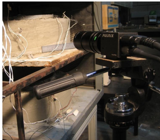
Figure 49. Digital Camera Used for Crack Investigations and Crack Width Measurement.
