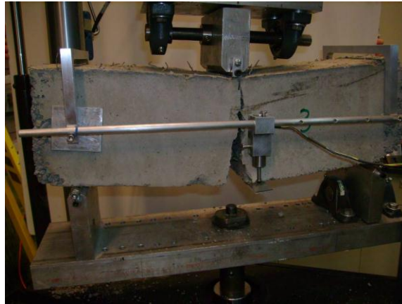
Figure 7. Crack Growth in FRC Samples under a Three-point Bending Test.
