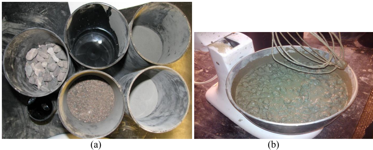
Figure 24. Casting Concrete with Lightweight Aggregate: a) Materials before Pouring into Mixer and b) Materials after Mixing.
