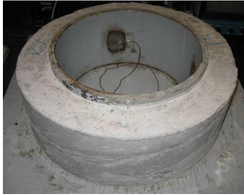
Figure 42. Examination of HVFA Concrete Specimens after Exposure to the Shrinkage Chamber.
