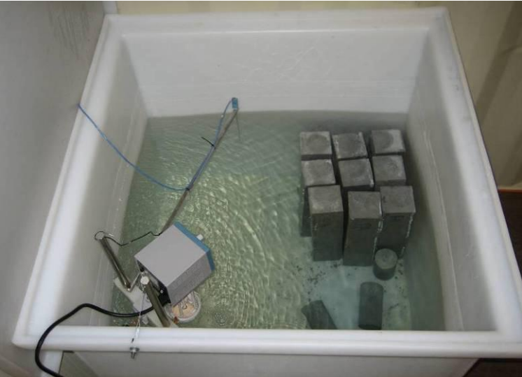
Figure 34. Curing of Specimens in the Water Tank at a Constant Temperature of 70° F.
