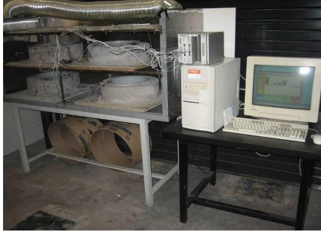
Figure 40. Shrinkage Chamber (with Cover Door Removed) Designed to Subject Restrained Concrete Ring Samples to Low Humidity Conditions.
