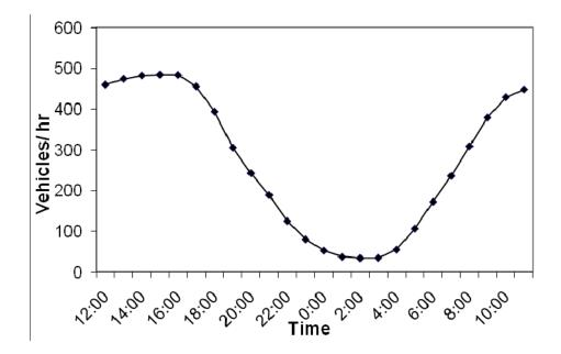
*Figure 4*. Hourly traffic volume (vehicles/hr) by hour along US 89, Arizona from 2007 to 2008, determined by an automatic traffic recorder installed in 2007.
