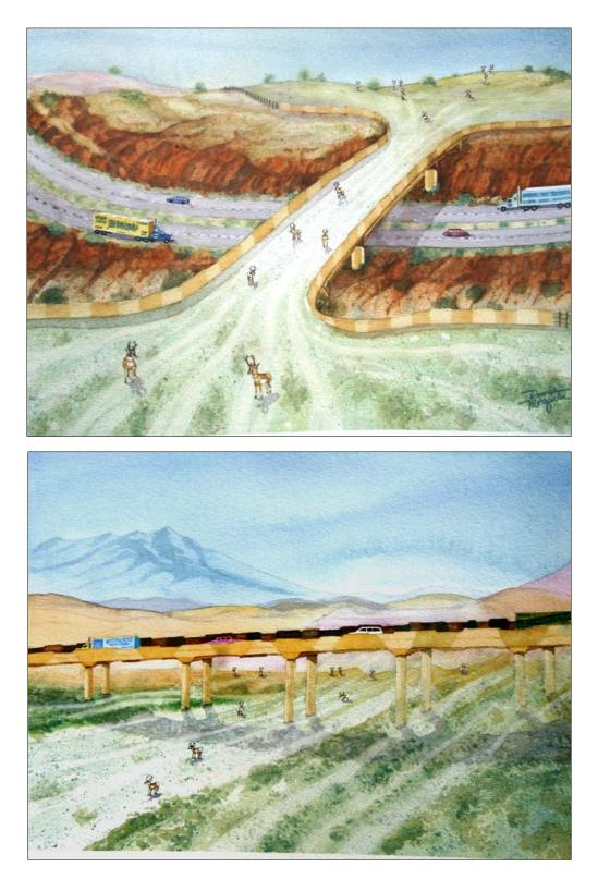
*Figure 16.* Renderings of potential pronghorn passage structures that emphasize openness and unobstructed views for crossing pronghorn, including an overpass capitalizing on existing terrain (top) and an elevated roadway/viaduct over gentle terrain (bottom).
