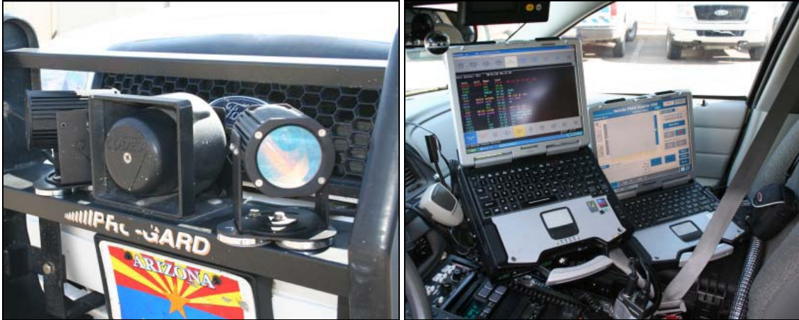
Figure 14. LPR Technology Installation for DPS Vehicles
