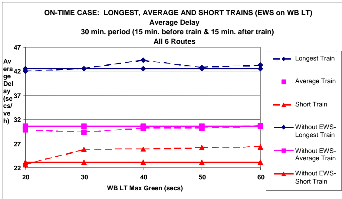
Figure 13: Delay for Different Gates Down Durations Using EWS on WB LT
