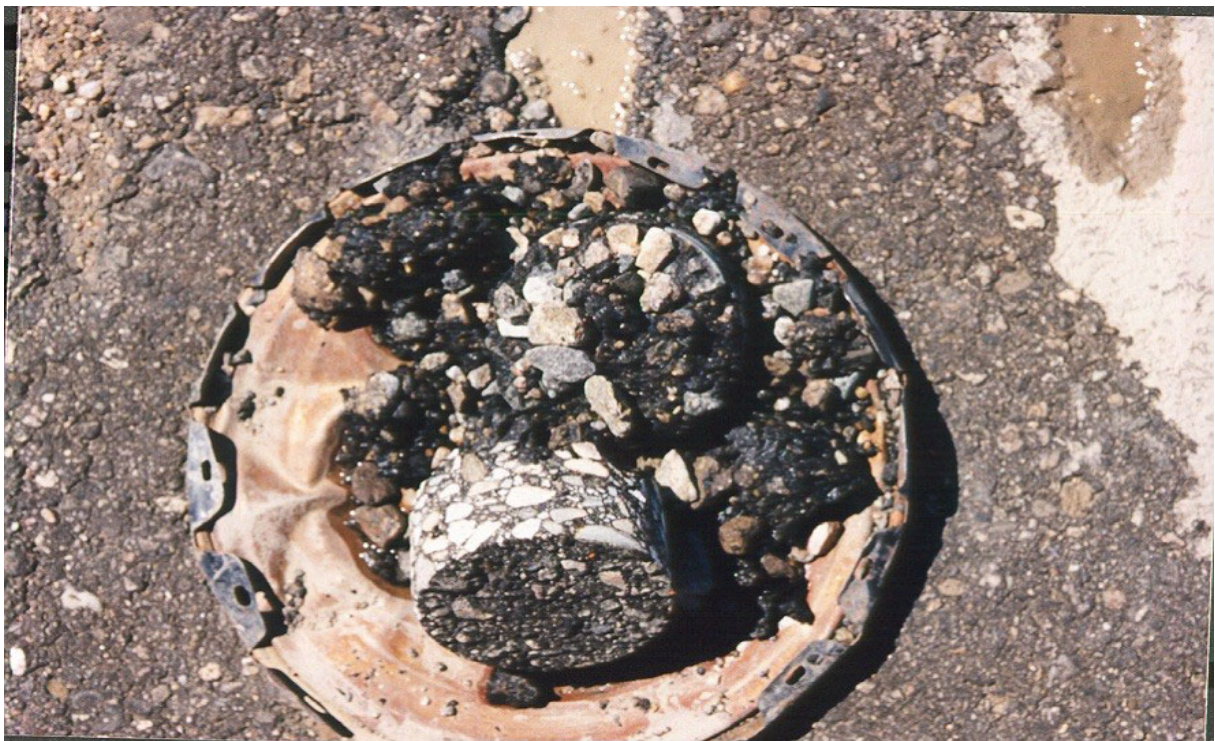
Photo No. 6 Severe Stripping Evident in Core Retrieval Remains
