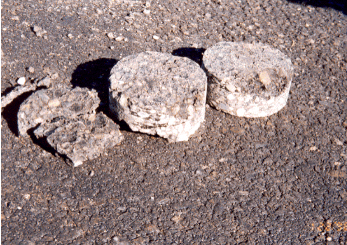
Photo No. 3 Remains of Core Attempt of \frac{3}{4} " Superpave Section (040902)
