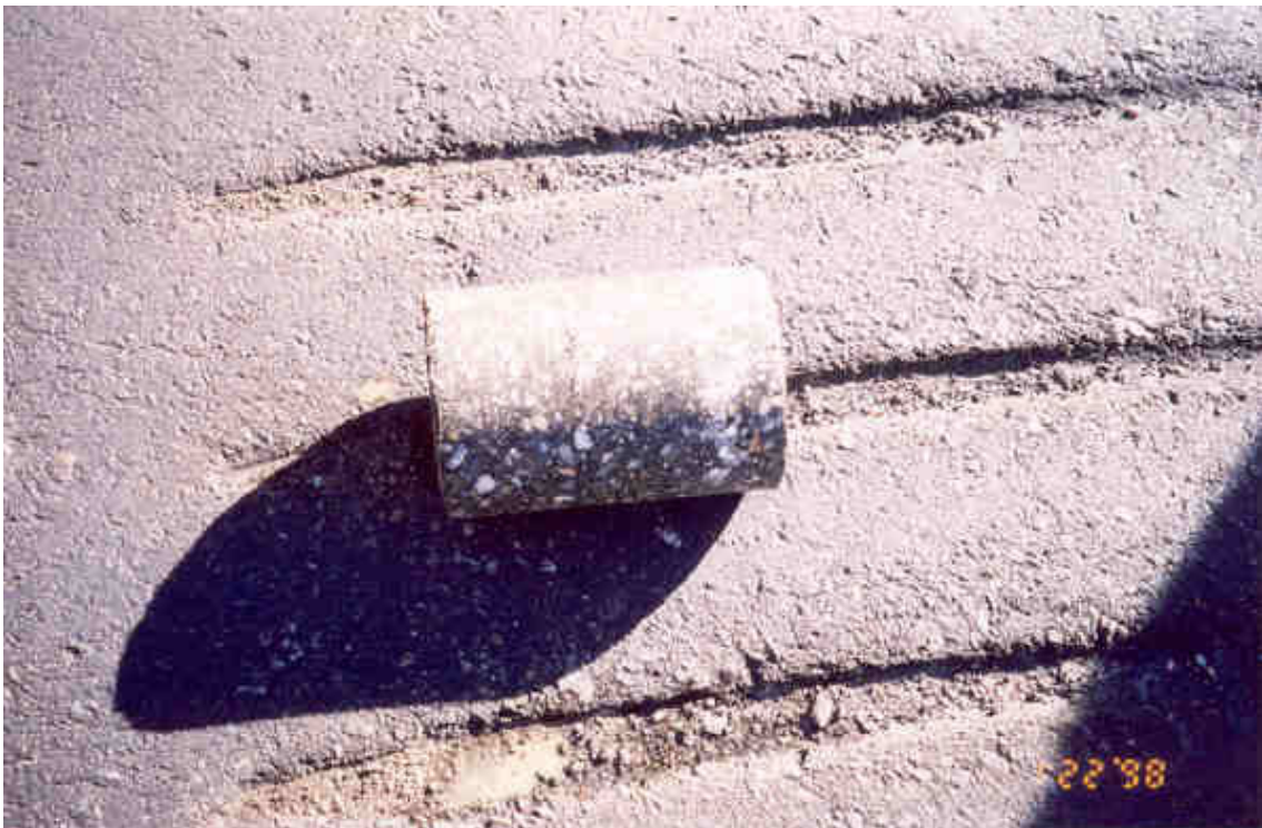
Photo No. 4 Intact Core of ADOT Base Mix Retrieved (040162)
