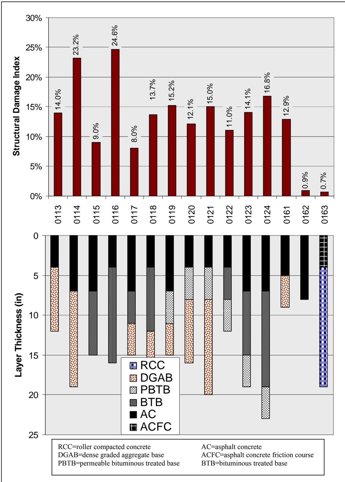
Figure 15. Structural Damage Index and pavement structure summary.
