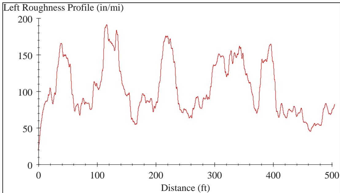
Figure 41. Roughness profile of section 0160, 25-ft base length.
