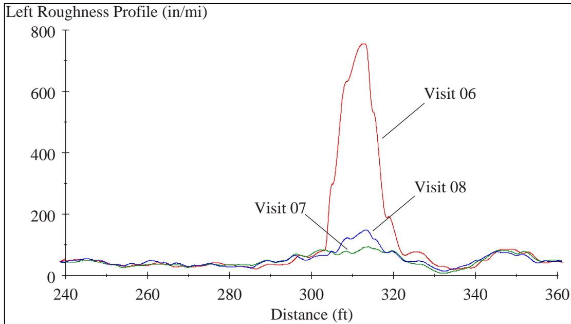
Figure 42. Roughness profile of section 0122, 10-ft base length.
