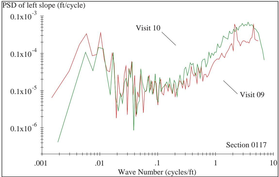
Figure 37. PSD plot of section 0117 profile, left side.
