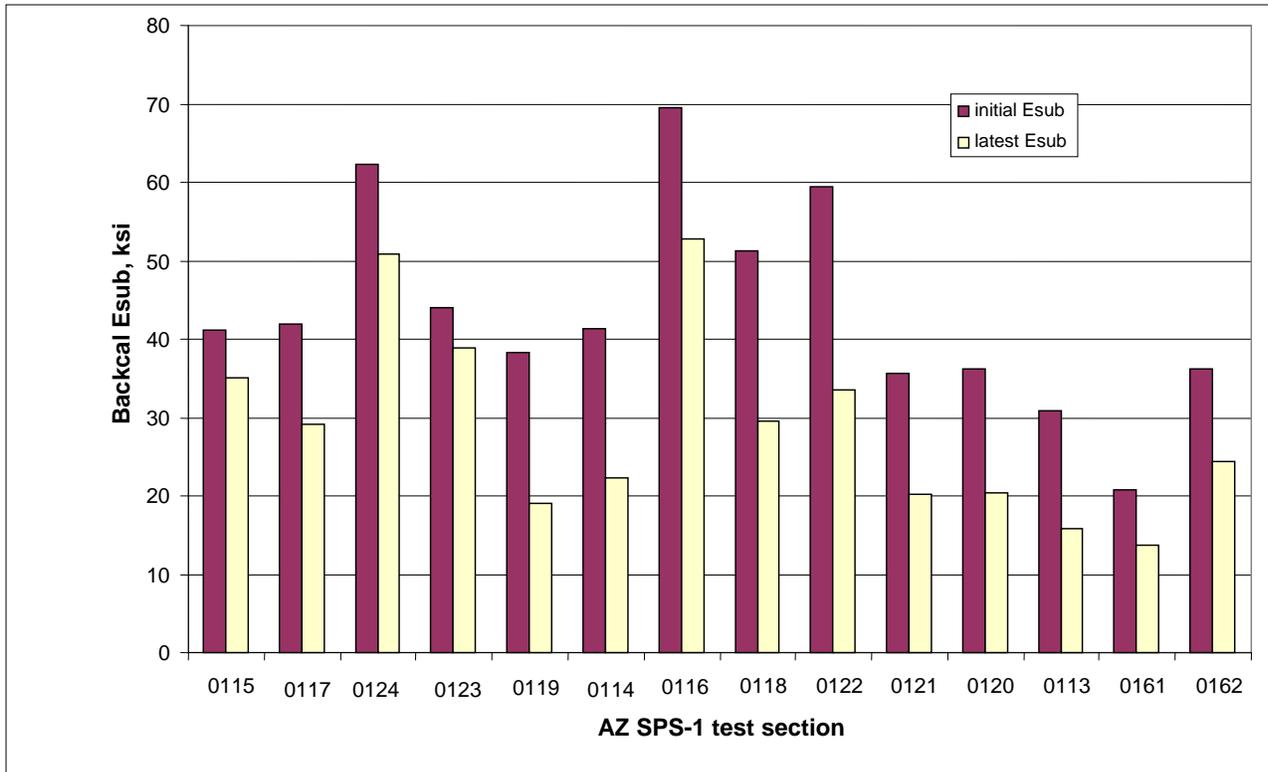
Figure 4. 1994 and 2004 backcalculated subgrade modulus by test section.
