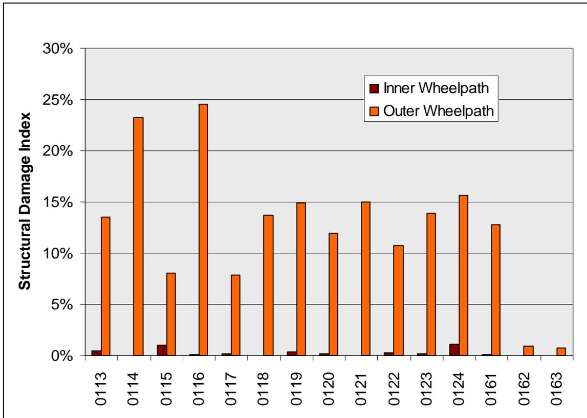
Figure 18. Structural Damage Index separated by wheel path.
