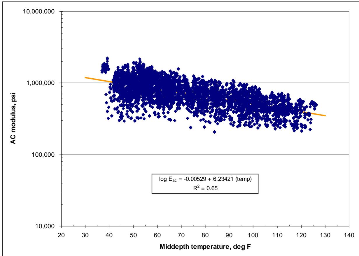
Figure 9. Backcalculated AC modulus versus temperature.
