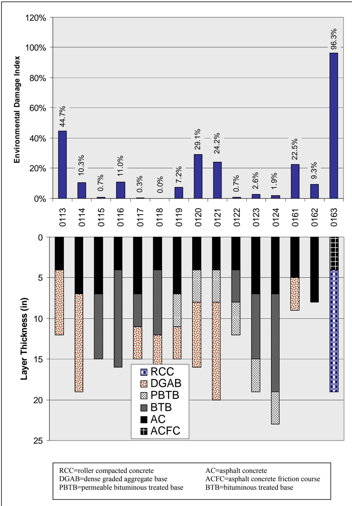
Figure 16. Environmental Damage Index and pavement structure summary.
