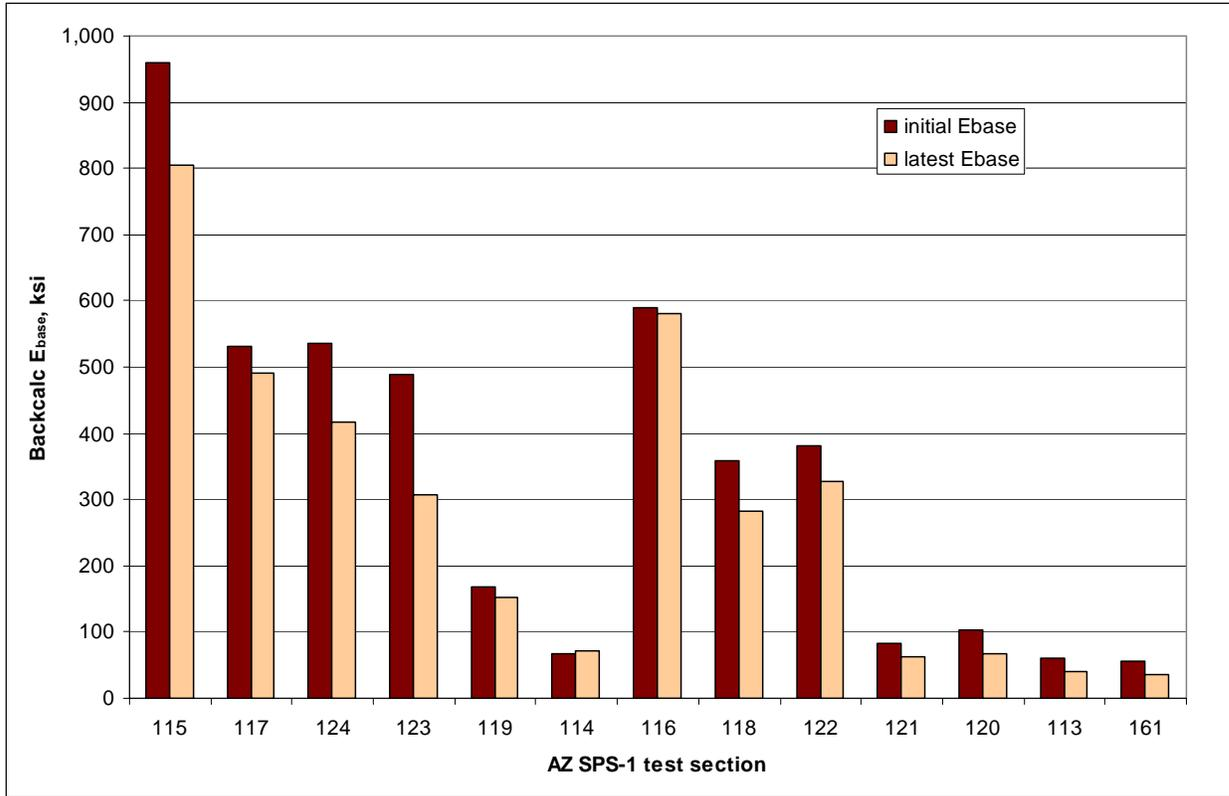
Figure 7. 1994 and 2004 backcalculated base modulus by test section.
