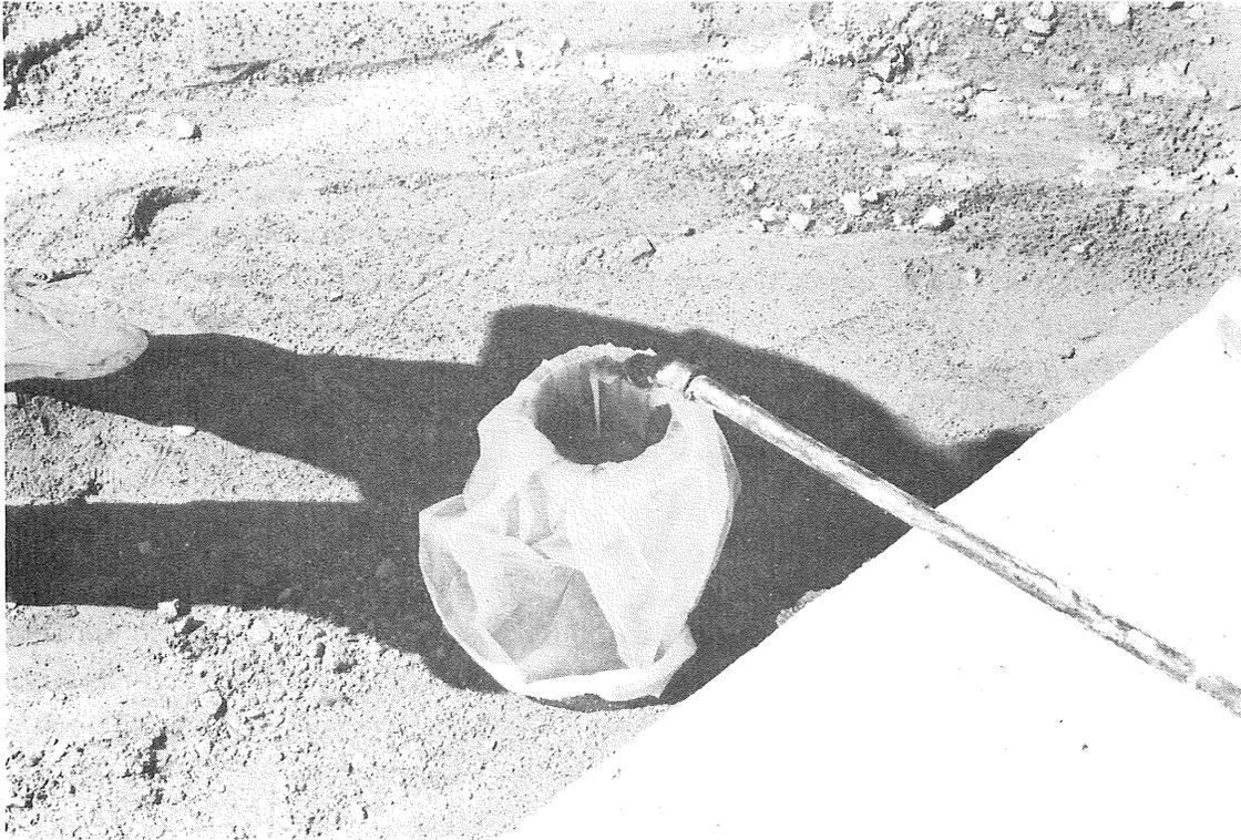
Figure 20 - Typical Sampling of Self Leveling Joint Sealants
