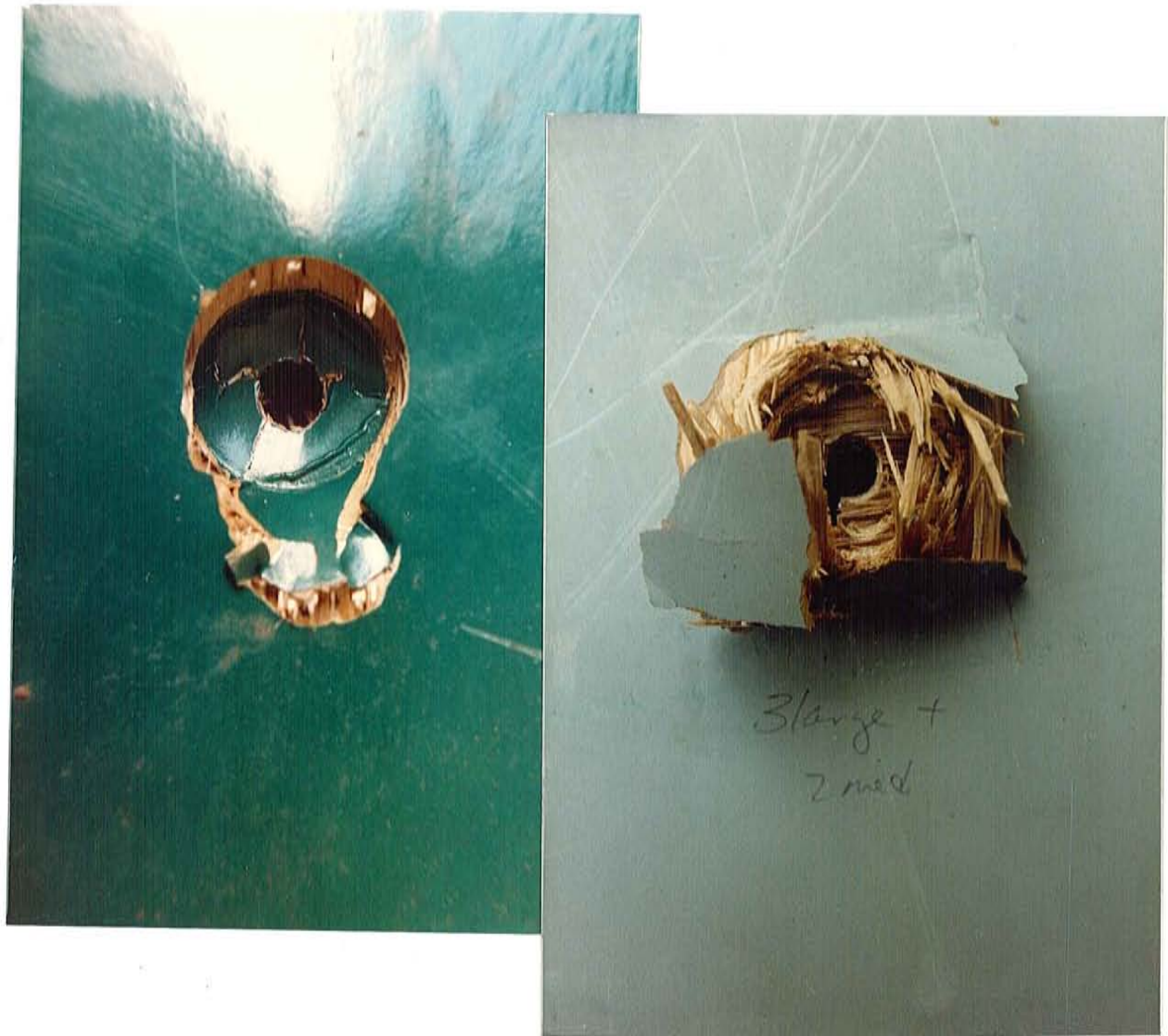
Figure X.11. Photograph of Typical Plywood Punching Shear Failure
