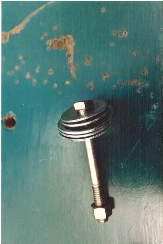
Figure X.10. Photograph of Stacked Fender Washers Following Pullout Test
