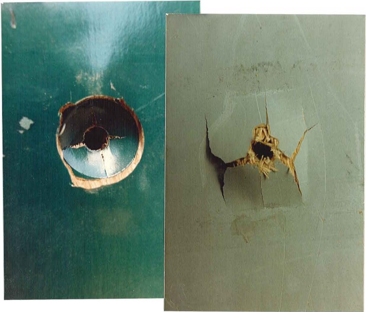
Figure X.9. Photograph of Plywood Following Large Fender Pullout Test
