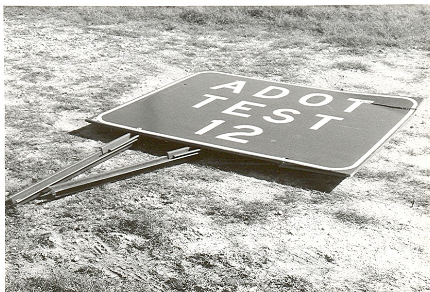
FIGURE A-90. SIGN INSTALLATION AFTER TEST 12.
