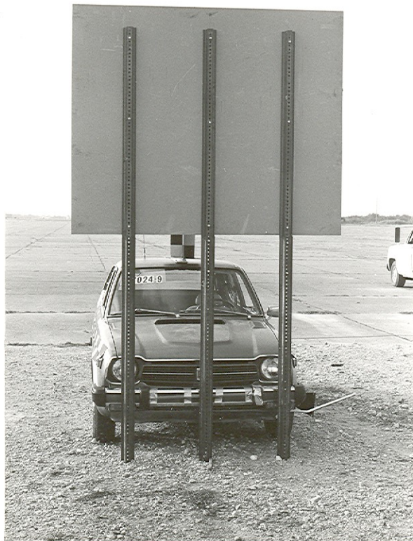
FIGURE A-73. RELATIVE POSITIONS OF TEST VEHICLE AND SIGN INSTALLATION FOR TEST 9.
