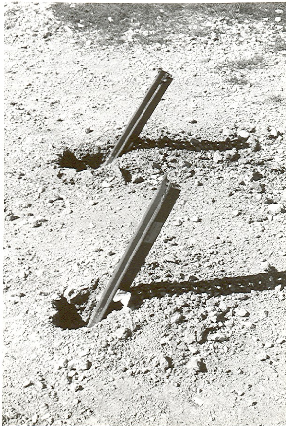
FIGURE A-85. SIGN INSTALLATION AFTER TEST 11.
