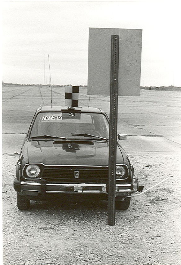
FIGURE A-94. RELATIVE POSITIONS OF SIGN INSTALLATION AND TEST VEHICLE FOR TEST 13.
