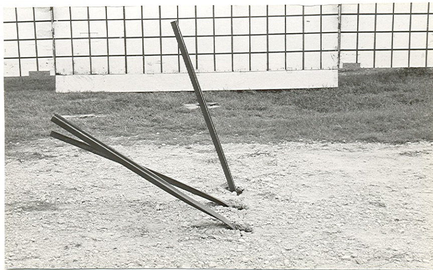
FIGURE A-79. SIGN INSTALLATION AFTER TEST 10.
