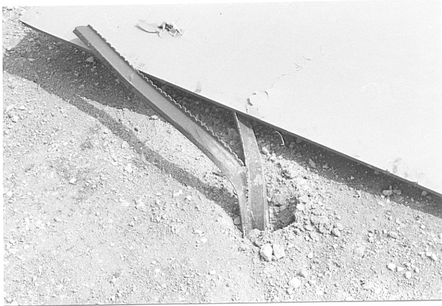
FIGURE A-147. SIGN INSTALLATION AFTER TEST 23.
