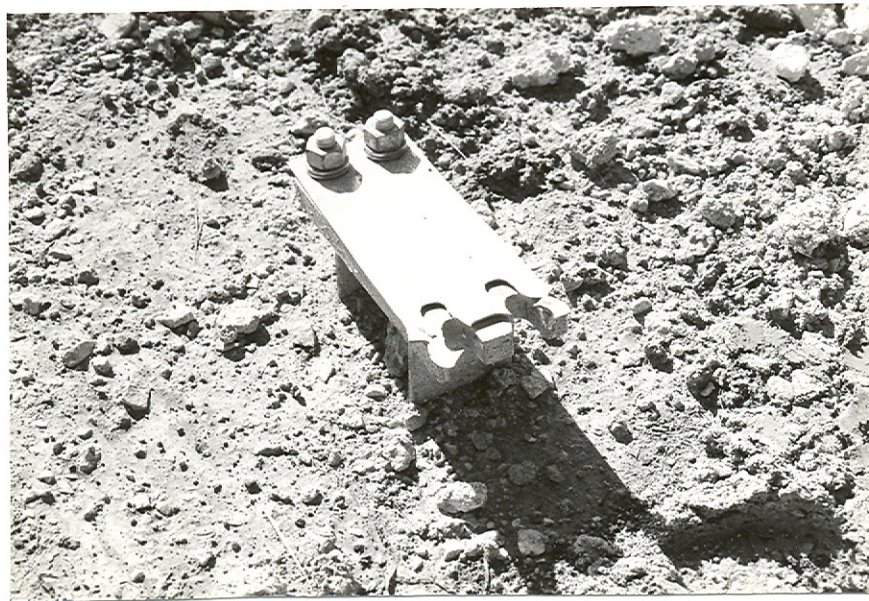
FIGURE A-31. BREAKAWAY BASE AFTER TEST 2.24-2.
