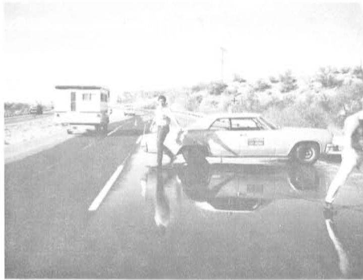
(A) Car skids at 40 MPH and rotates 90° clockwise
