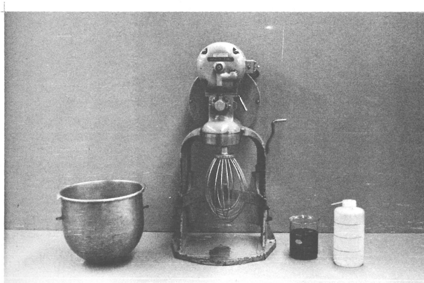
FIGURE 8 Photograph of the Hobart Mixing Equipment Used for Blend Soil, Water, and Emulsion
