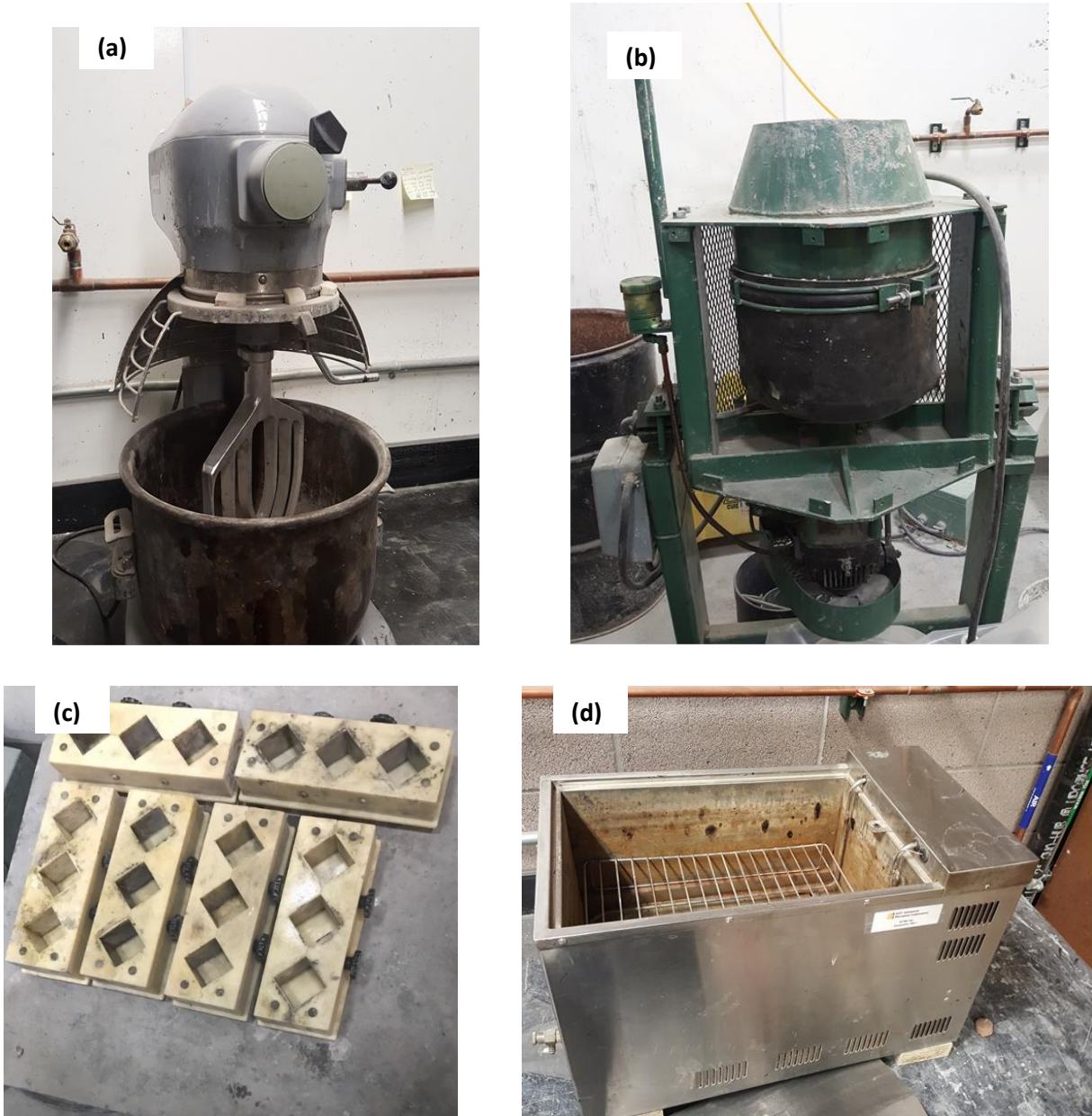
Figure 23. (a) Hobart mixer, (b) Omni high shear mixer, (c) cubical molds used for casting, and (d) water bath
