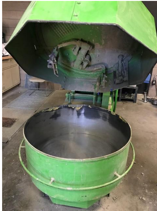
Figure 57. Croker RP150XD rotating pan mixer
