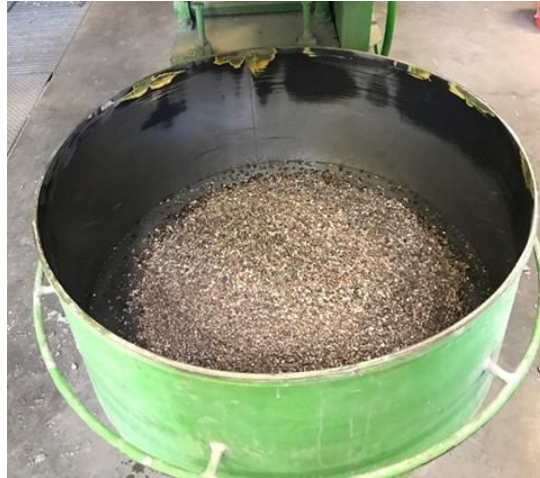
Figure 59. Coarse aggregates (#4, #8 and #10) added to the mixer
