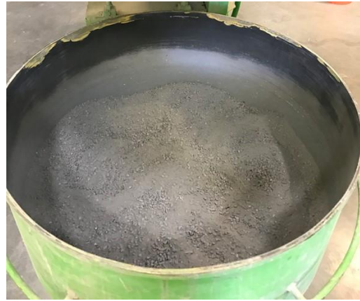
b) Blending the micro-silica and aggregates
