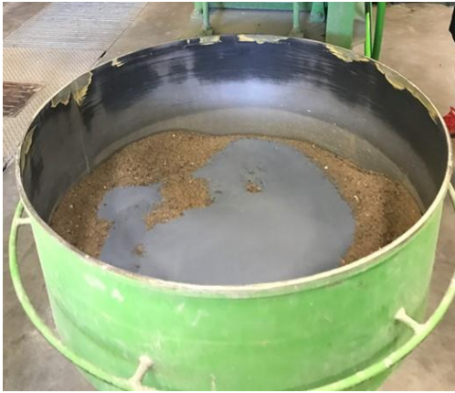
a) Addition of micro-silica to aggregate mixture
