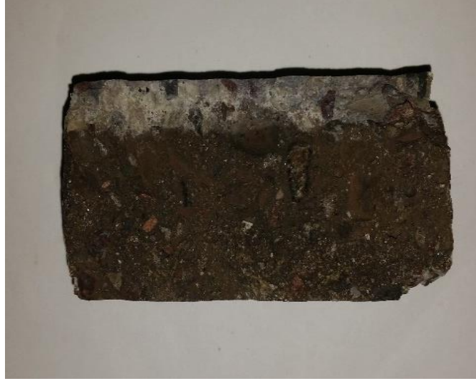
Figure 153. Axially split specimen tested under NSSM showing chloride penetration
