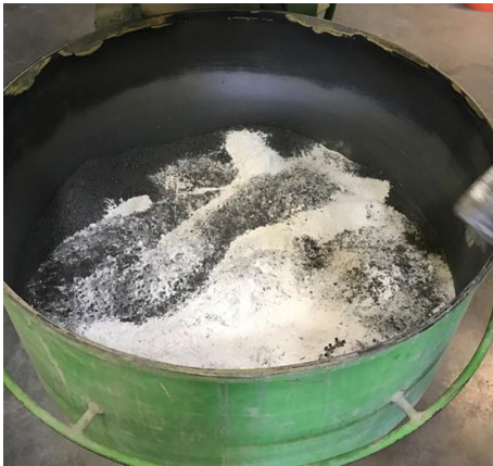
c) Addition of limestone to the aggregate blend
