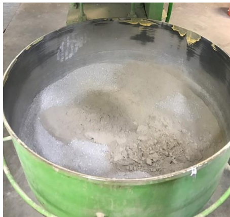
e) Addition of fly ash to the blend
