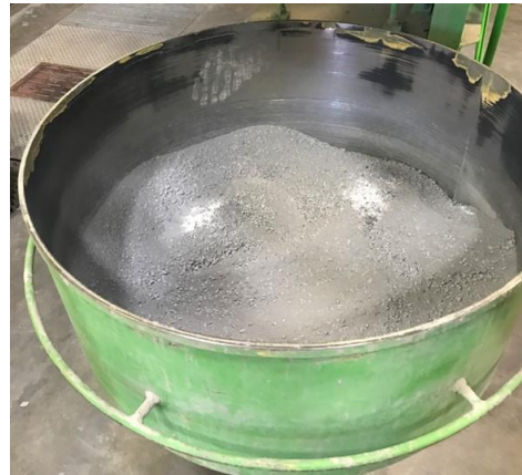
d) blending of limestone and aggregate blend
