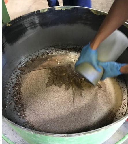
Figure 61. Mixing water added to the aggregate to attain SSD condition
