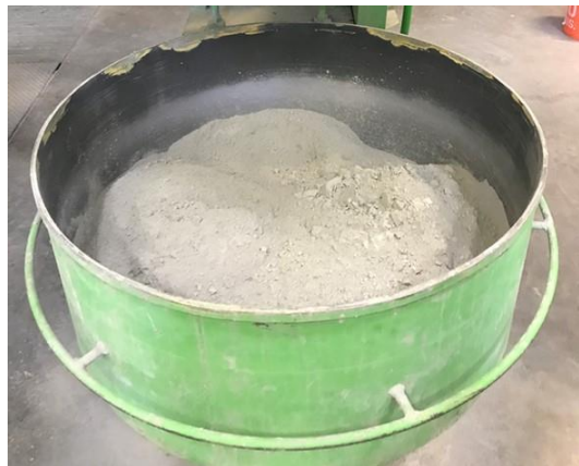
f) Addition of cement to the final blend
