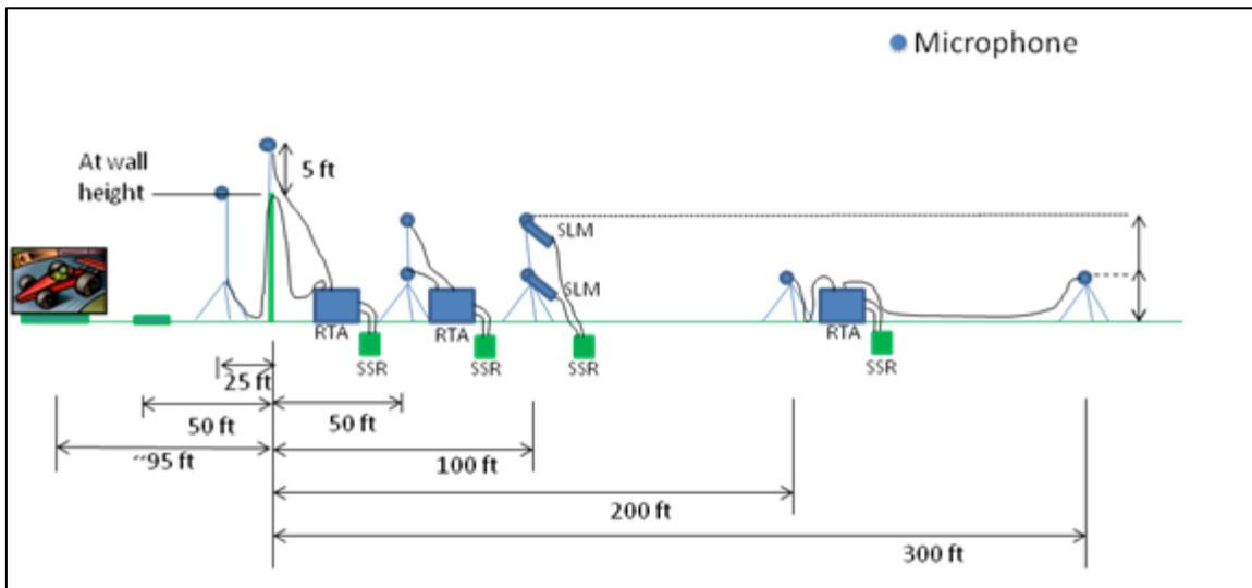
**Figure 3: Acoustic Measurement Site Diagram**
