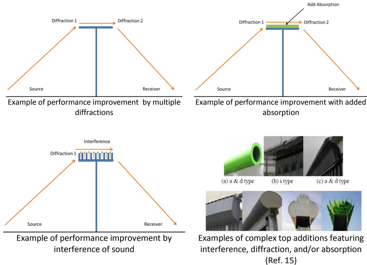
**Figure 1. Different Types of Barrier Top Treatments**
