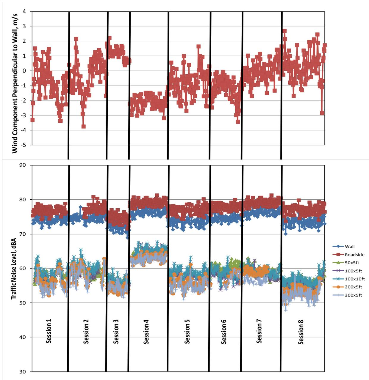
**Figure 28: Measured Wind Component and Sound Pressure Levels, All Sessions**
