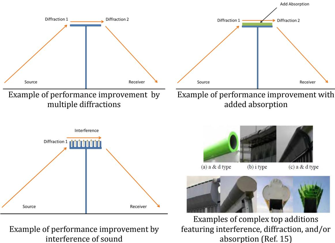
**Figure 1: Different types of barrier top treatments**
