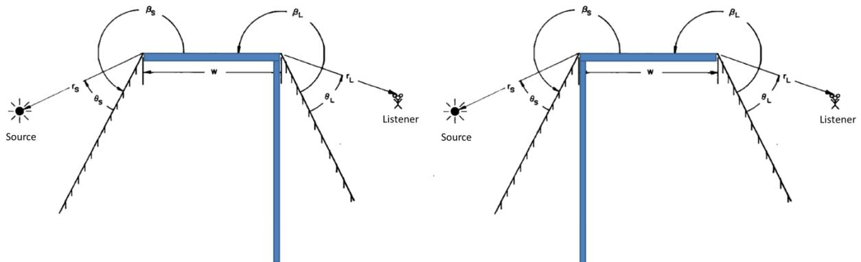
Figure 25. Representation of a L-Top barriers LU (left) and LD (right) using wide barrier theory from Pierce
