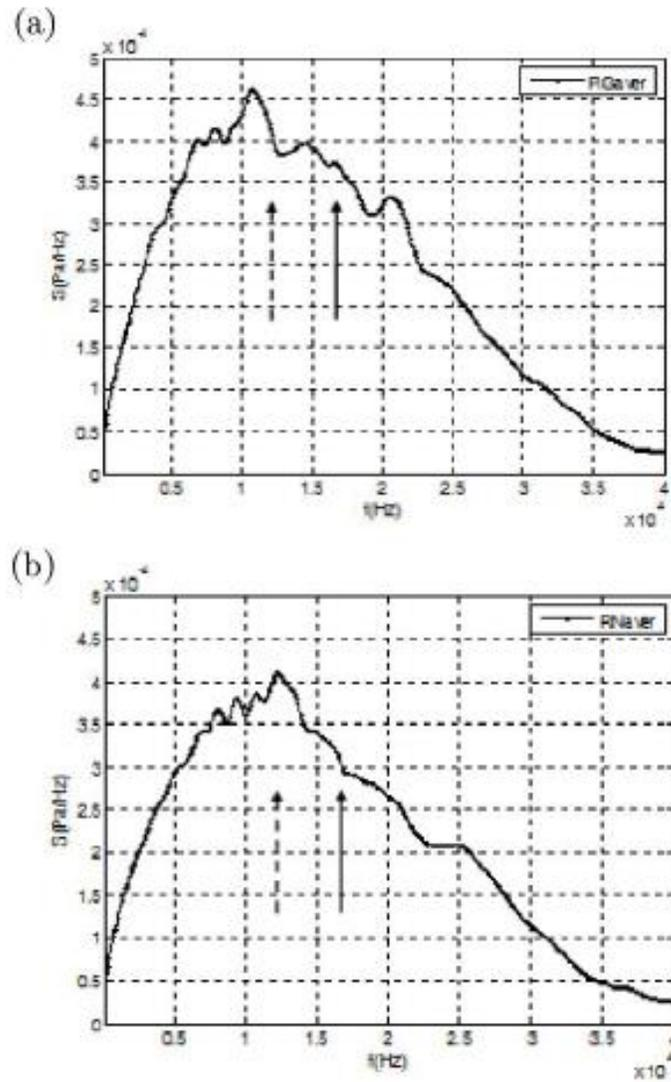
Figure 8: Spectrum density amplitudes for the mean diffracted pressure signal for (a) the RG jagged regular barrier top and (b) the RN jagged random barrier top. The mean is based on 17 measurements at different lateral positions as described in the text. The solid arrow shows the estimated characteristic frequency of the free (F) signal and the dash arrow shows the approximate position of the spectral maximum in each case.
