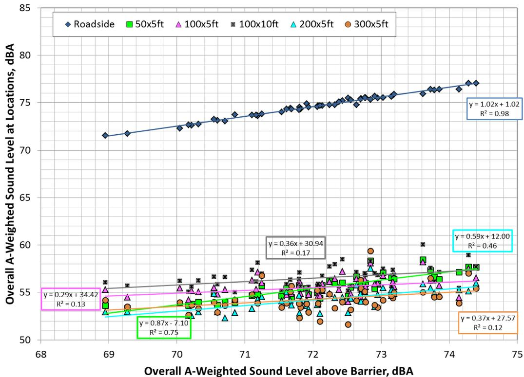
**Figure 11. Sound Pressure Levels from the Roadside and behind the Sound Wall Plotted Versus Levels above the Sound Wall for Measurement Session 3**
