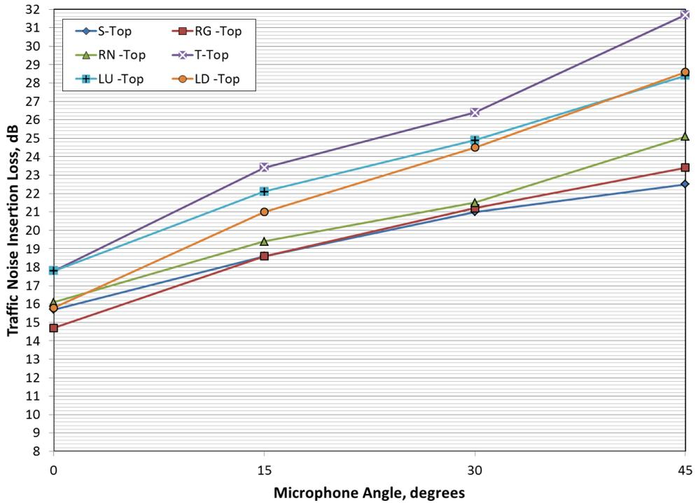
Figure 23. Traffic Noise Insertion Loss Based on Acoustic Scale Modeling Results for a Source Angle of 30° and a Full-Size R distance of 14.8ft (4.5m)
