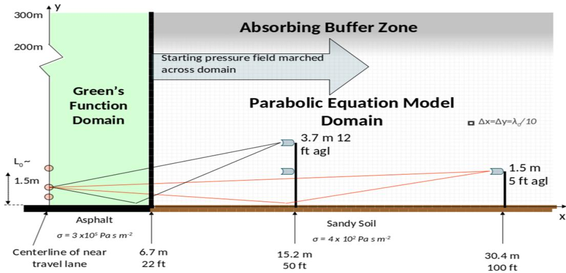
Figure 29. Geometry and calculation domains used model highway noise propagation in ADOT Project SPR-605
