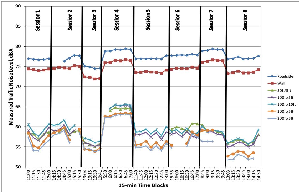
**Figure 25: Measured Traffic Noise Levels, 15-Minute Averages**
