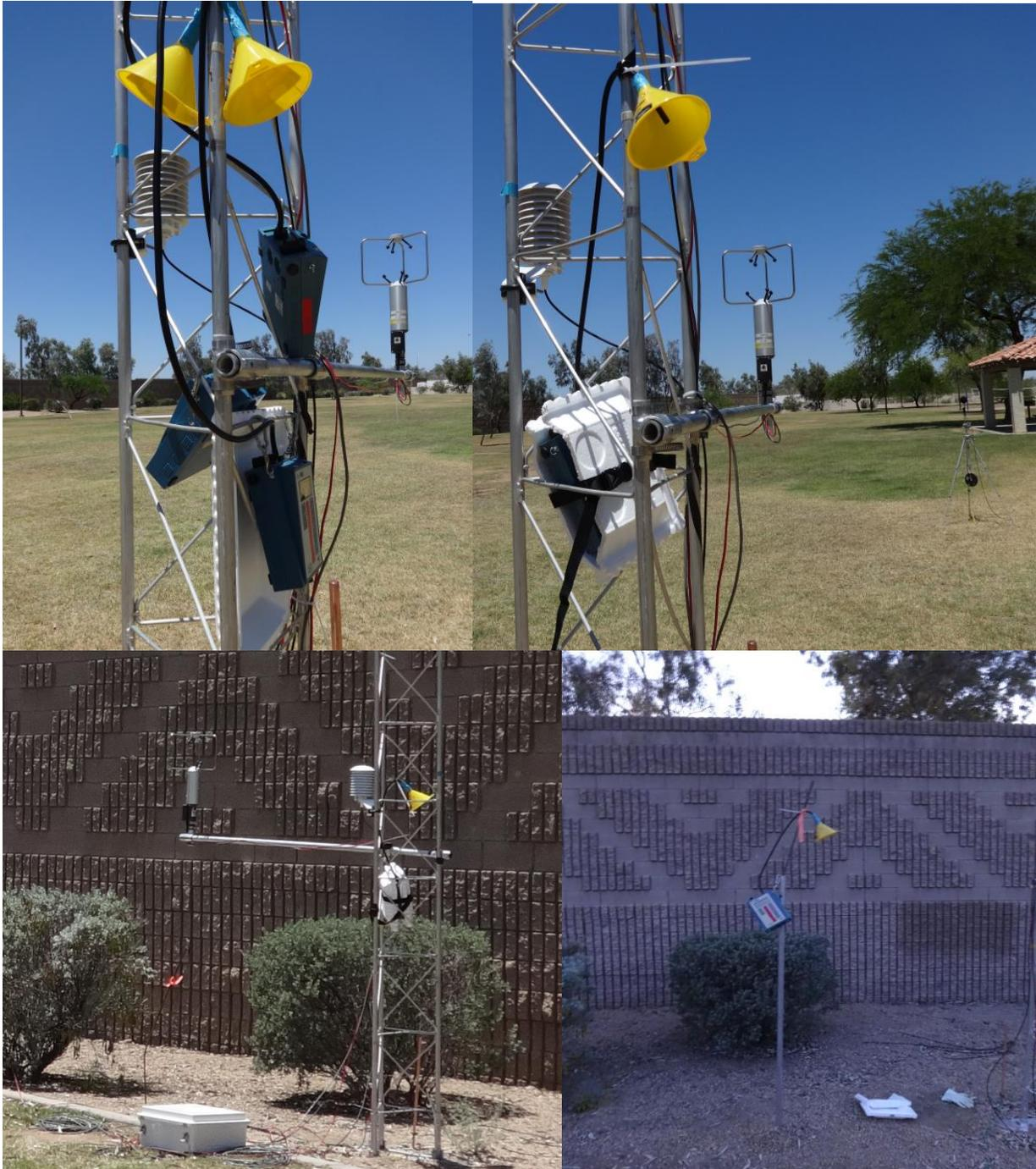
Figure 26. Images of DustTRAK configuration 1 field tower (top left), and configuration 2 for the: field tower (top right) wall tower (bottom left) and wall tower during disassembly of wall tower (bottom right).
