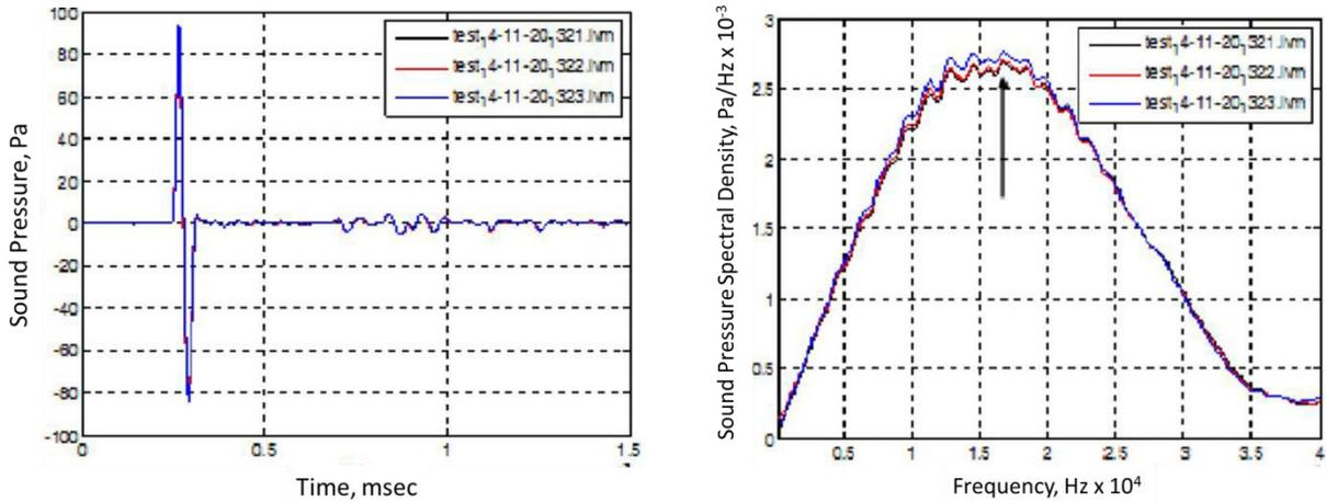
**Figure 12. Spark Source Time Trace (a) and Spectrum (b)**
