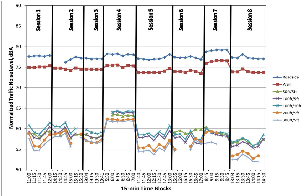
**Figure 26: TNM Normalized Traffic Noise Levels, 15-Minute Averages**
