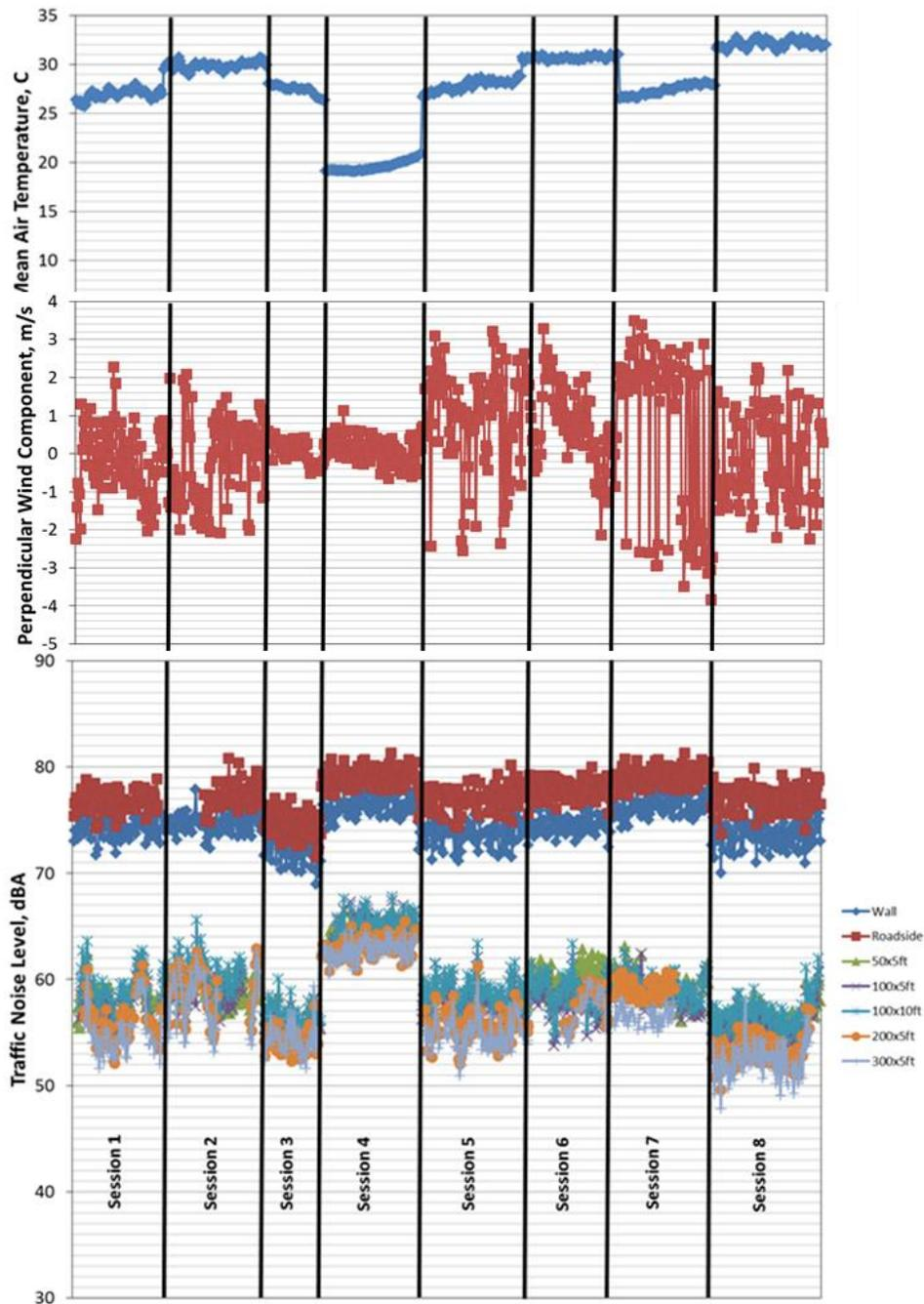
**Figure 10. Measured Wind Component, Air Temperature, and Sound Pressure Levels, All Sessions**
