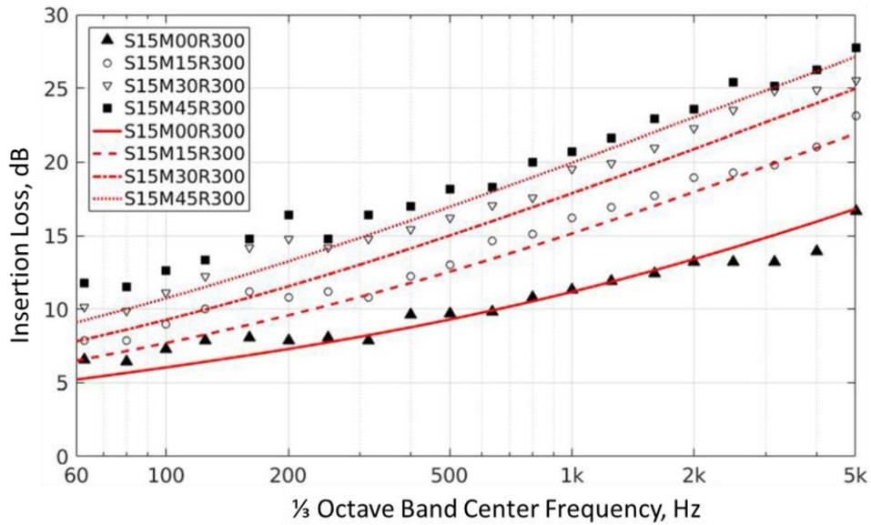
**Figure 18. Comparison of Experimental and Theoretical Results (from Eqn 8) for Straight (S) Top Source at 15° and Microphone at 0°, 15°, 30°, and 45° and a distance of 30cm**
