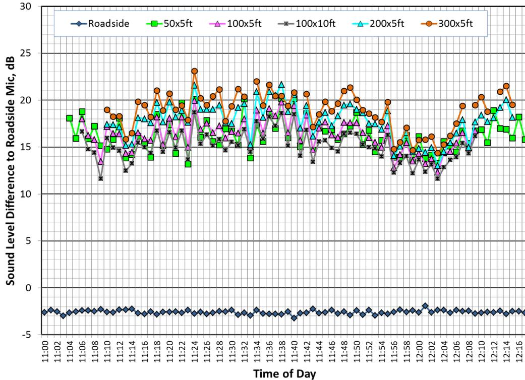
**Figure 7. One-Minute Average Noise Levels Differences Relative to Top of Sound Wall Levels in Session 1**
