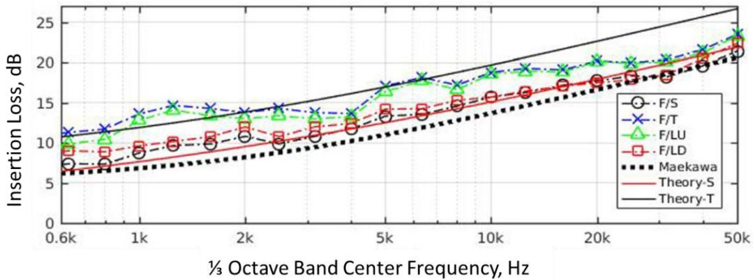
**Figure 19. Comparison of Experimental and Theoretical Results for S-Top, T-Top, L-Top (LU) and L-Top LD Barrier Configurations**
