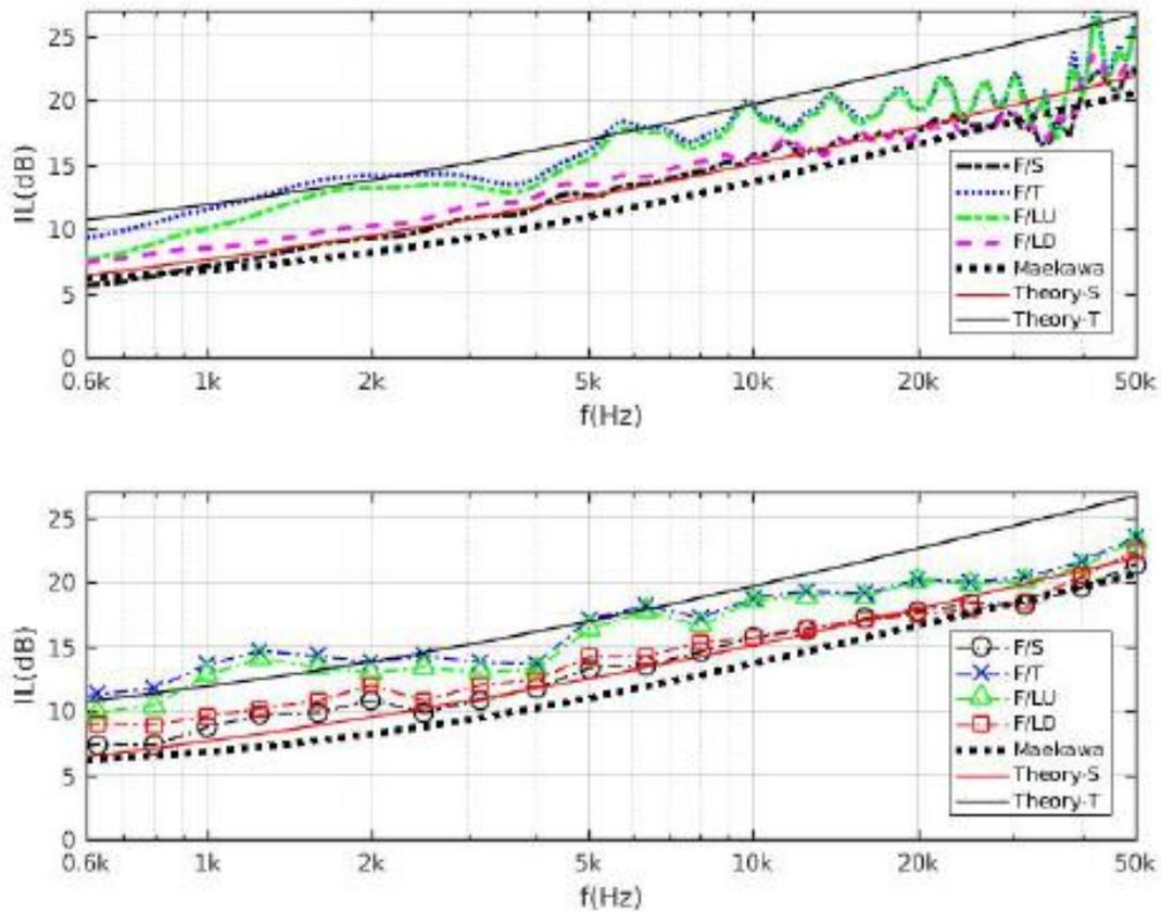
Figure 10: Insertion loss,  $IL$ , as a function of laboratory frequency  $f$  for the laterally homogeneous barriers including a thin screen (S), a T-shaped top (T) and L-shaped tops (LU and LD) relative to the free signal (F). Top - results from FFT computations. Bottom - 1/3rd octave filter calculations. The predictions from Maekawa's IL estimate for a thin screen and geometrical theory of diffraction results for a thin screen and T-top are also shown.
