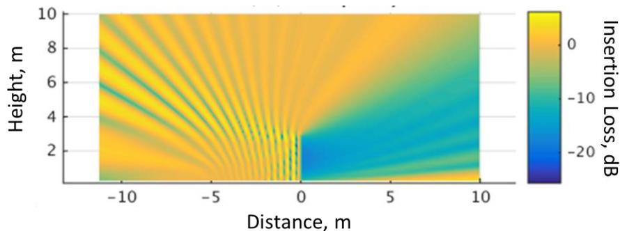
**Figure 27. Calculated insertion loss around a 3m sound wall for a source at distance -5m using OpenBEM**
