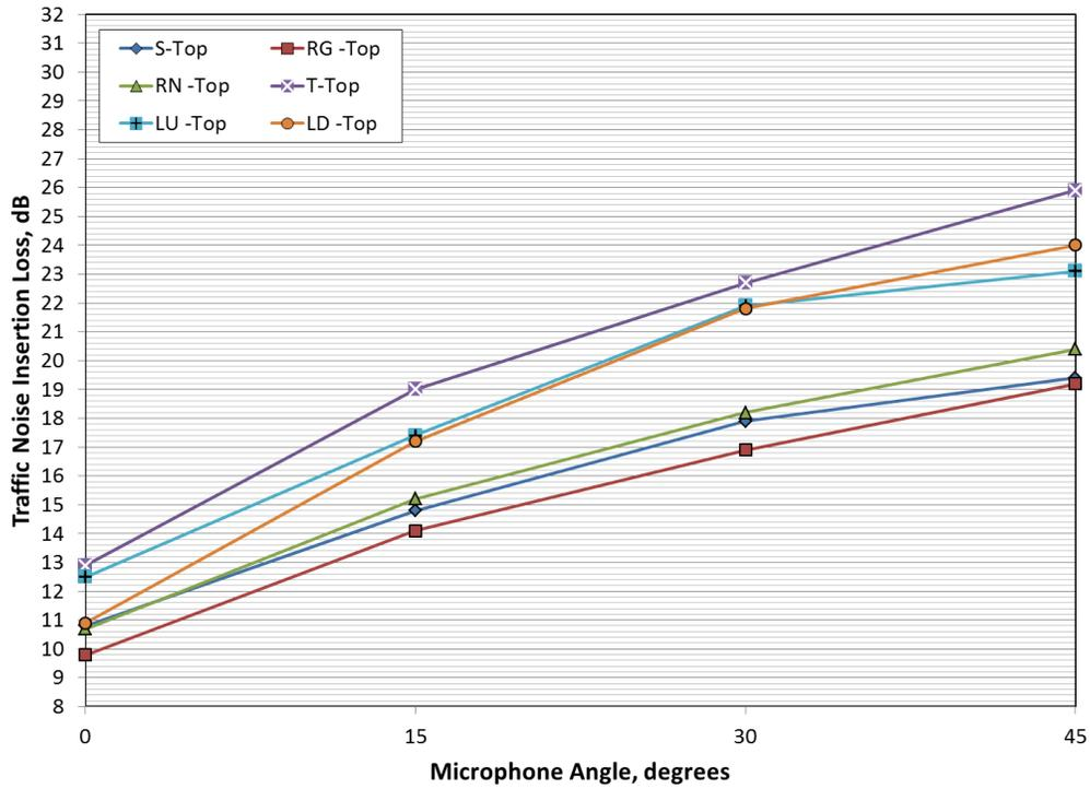
Figure 20. Traffic Noise Insertion Loss Based on Acoustic Scale Modeling Results for a Source Angle of 15° and a Full-Size R distance of 9.8ft (3m)
