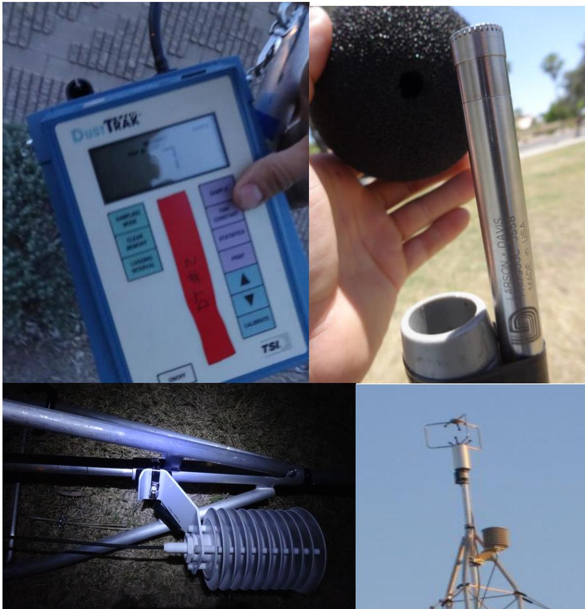
Figure 18. Images of various equipment: (top left) TSI DustTRAK; (top right) microphone; (bottom) detail showing mounting of 10 m sonic and “10 m” hygroclip which is at the top of the 3rd 10 ft tower section to reduce possible wake from the radiation shield (bottom left) on ground when disassembling (bottom right) on field tower during the observation period.
