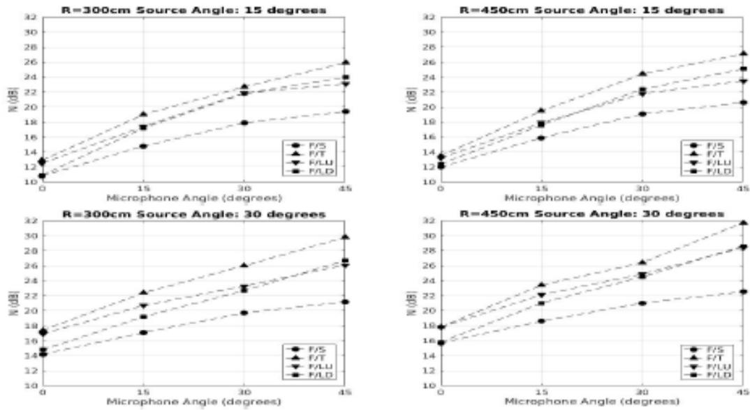
Figure 12: Directivity diagrams (relative to free F signal) for the single number insertion loss rating  $N$  as functions of microphone angle,  $\theta_M$ , for different source angles  $\theta_S$  and distances from barrier top  $R$ . Results for different barrier top geometries S, T, LU and LD are shown.
