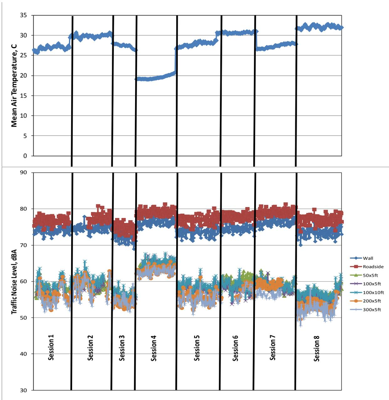
Figure 27: Measured Air Temperature and Sound Pressure Levels, All Sessions
