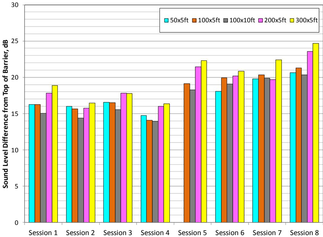
**Figure 24: Session Average Insertion Loss from Barrier Position**
