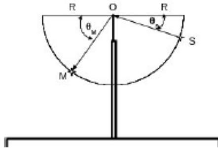
Figure 5: Schematic showing microphone, M, sound source, S, and angles,  $\theta_M$  and  $\theta_S$ , relative to the horizontal line passing through the origin, O, which coincides with the top of the barrier. The microphone and the sound source are at the same distance,  $R = 30$  or  $45$  cm, from the origin and the angles used are:  $\theta_S = 15^\circ, 30^\circ$ ,  $\theta_M = 0^\circ, 15^\circ, 30^\circ, 45^\circ$ .
