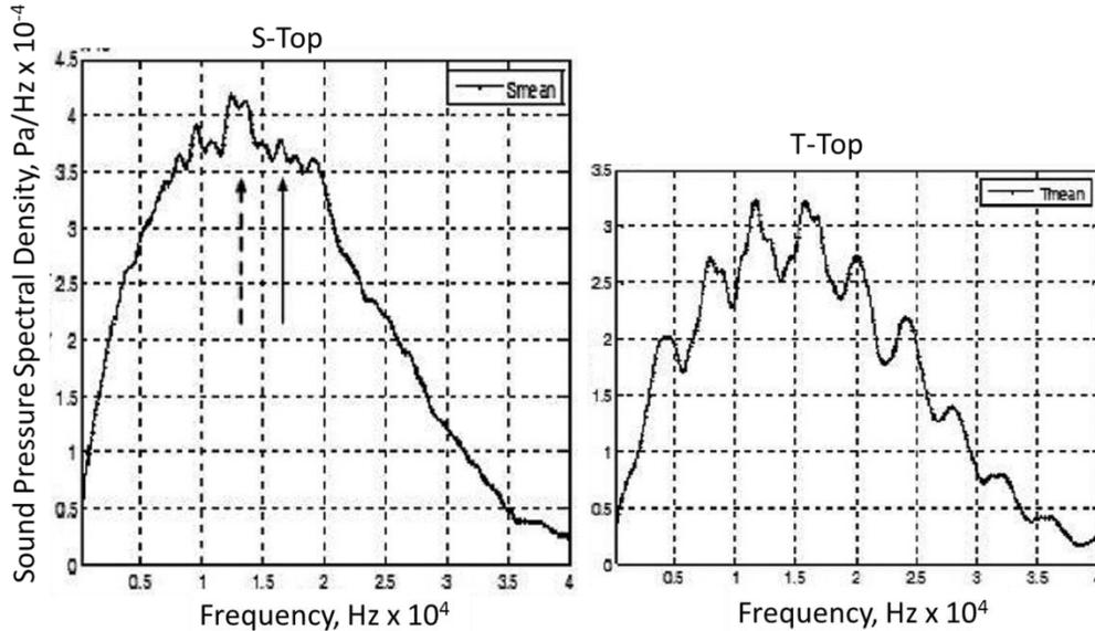
**Figure 16. Frequency Spectra for the Straight (S) Top and Tee (T) Top Barrier Configurations**
