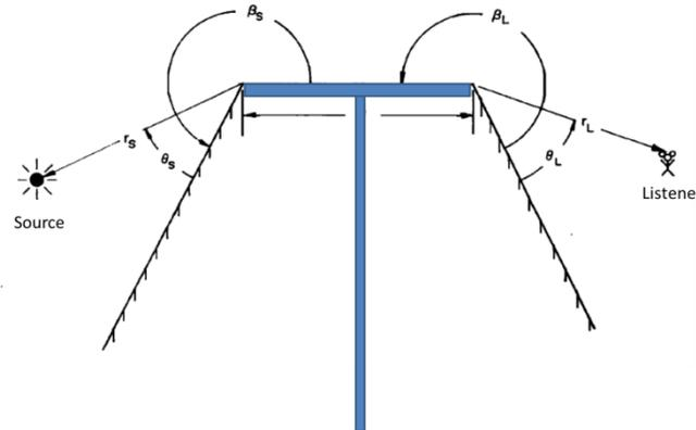
Figure 24. Representation of a T-Top barrier using wide barrier theory from Pierce
