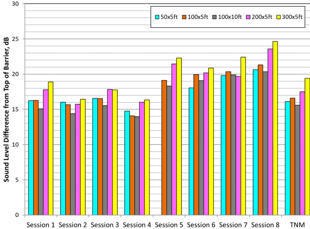
**Figure 9. Values for the Noise Level Differences between the Top of the Sound Wall Measurement Location and the Microphone Locations behind the Wall**
