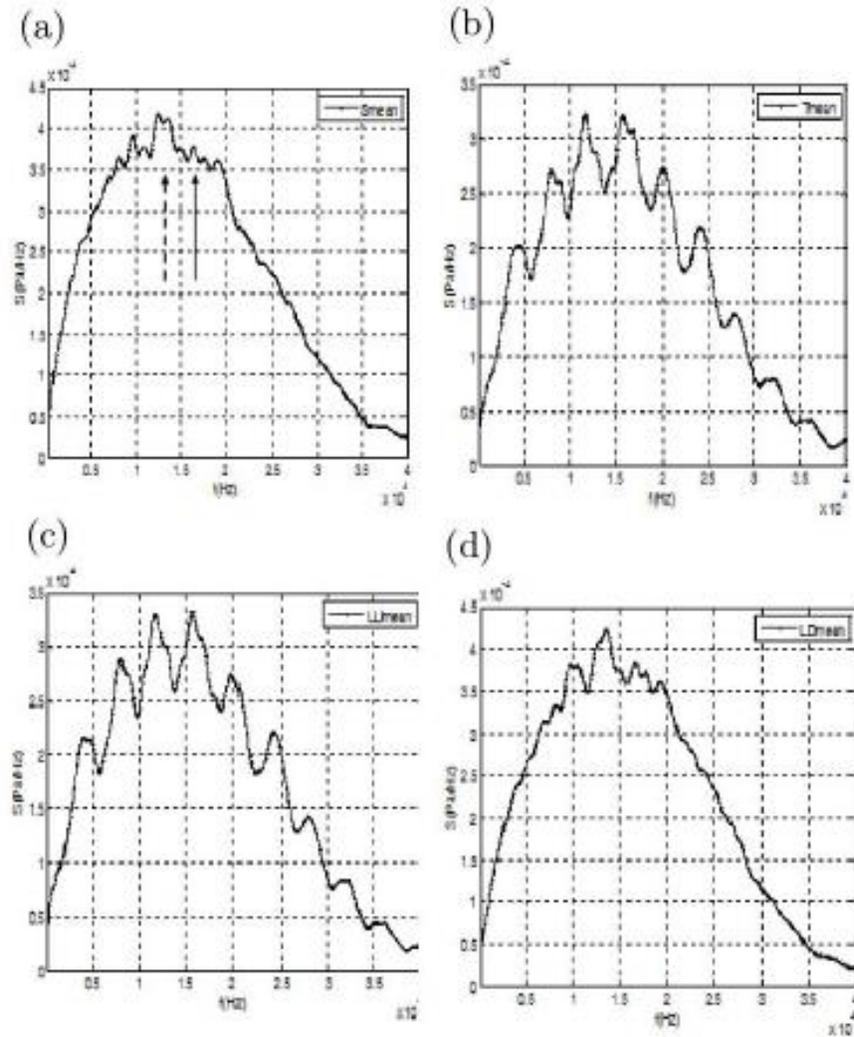
Figure 7: Spectrum density amplitudes for the mean diffracted pressure signal for the following homogeneous barrier tops: (a) thin vertical screen (S), (b) T-shaped top (T), (c) L-shaped (LU) top and (d) L-shaped (LD) top. The solid arrow shows the estimated characteristic frequency of the free signal and the dashed arrow shows the approximate position of the spectral maximum.
