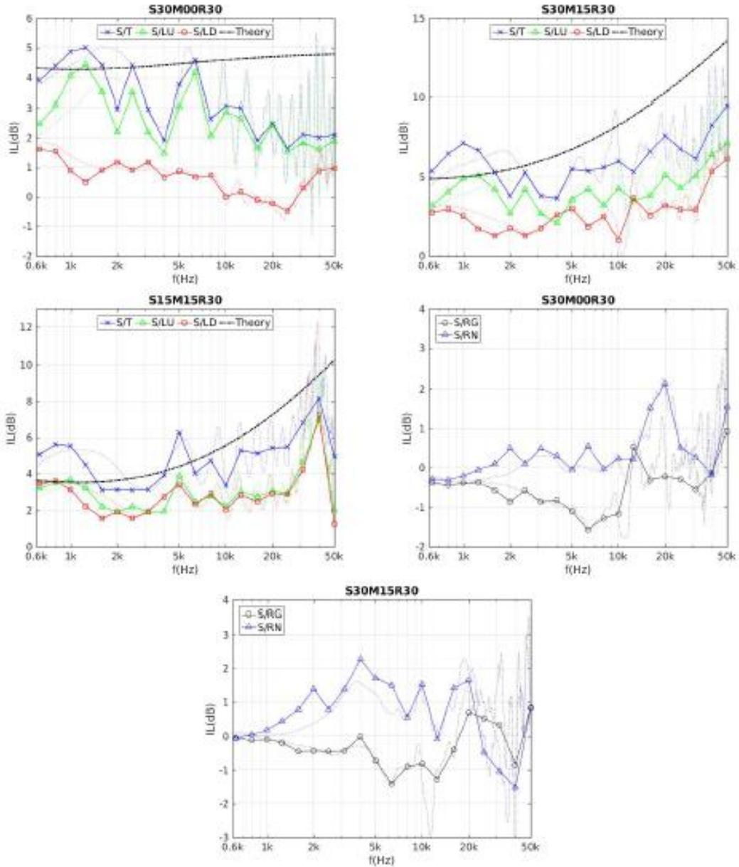
Figure 11: Insertion loss,  $IL$ , as a function of laboratory frequency  $f$  for the T-shaped top (T), the L-shaped tops (LU and LD) and the laterally heterogeneous tops (RG and RN) relative to the thin screen barrier (S) for different configurations of source and microphone positions. Faint lines show FFT results. Predictions from the geometrical theory of diffraction for the relative insertion loss of a T-top barrier relative to a thin screen are also shown.
