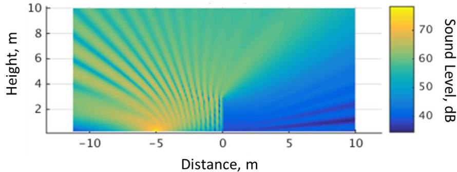
**Figure 26. Calculated sound field around a 3m sound wall for a source at distance -5m using OpenBEM**
