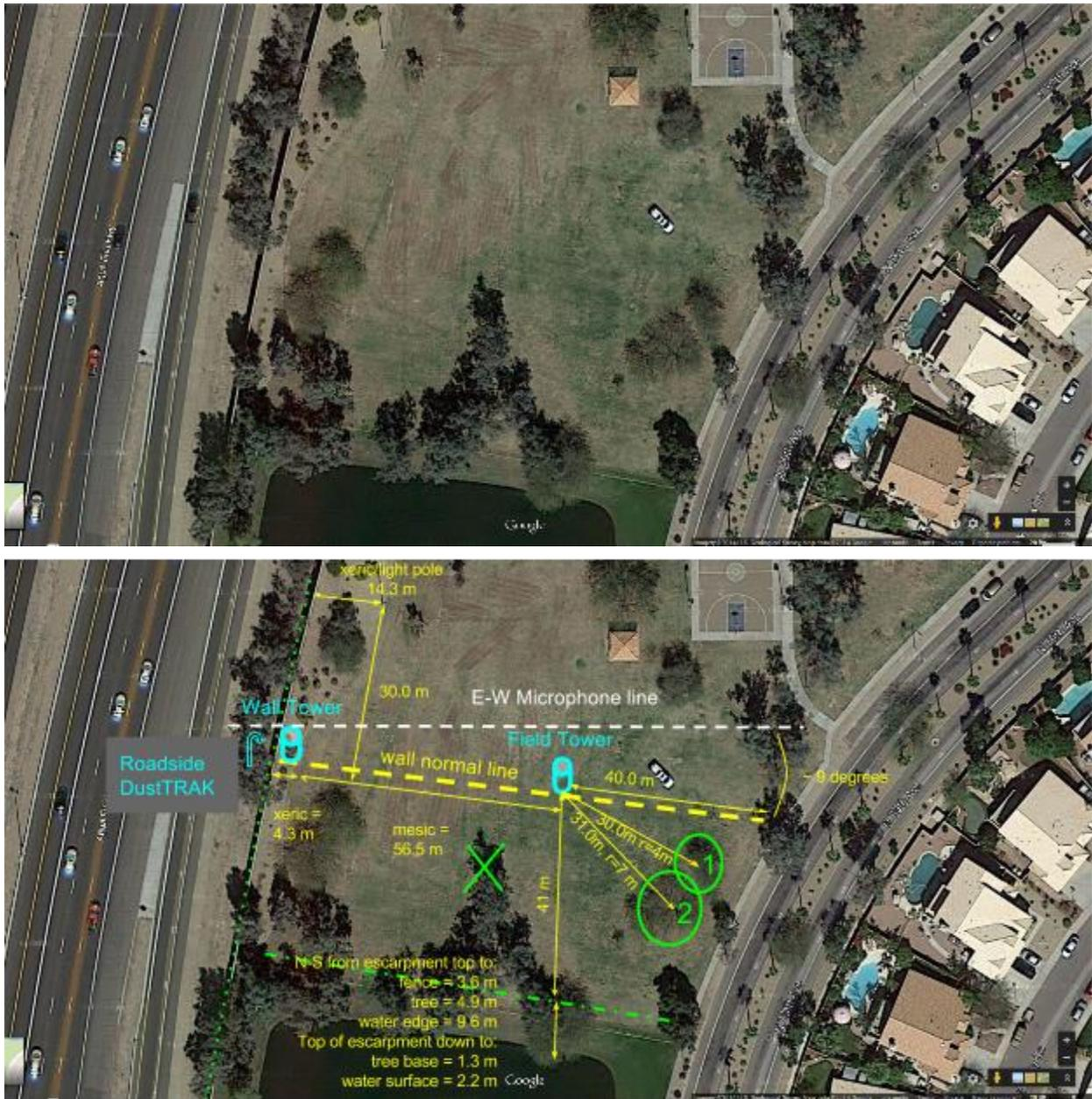
**Figure 2. Google Maps overview of Oasis Park (top) with schematic of setup measurement lines and distances for a few features (bottom) used during May 2012 experiment. See text for description.**
