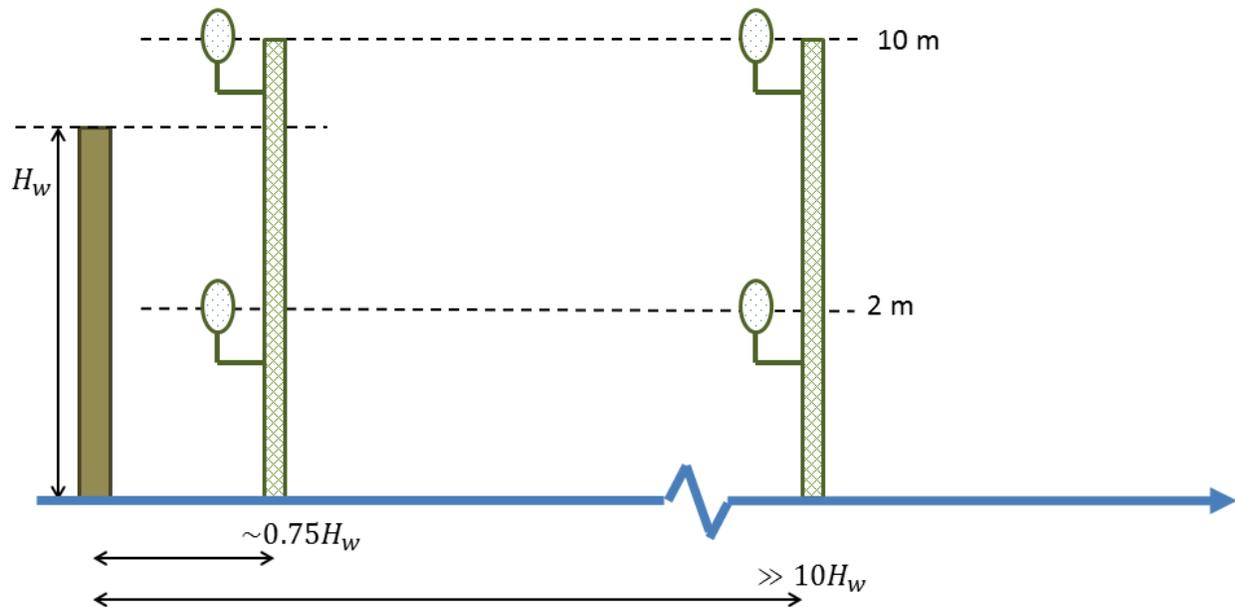
**Figure 1. Schematic of ADOT SPR-699 basic experimental setup for two 10-meter towers with 2 sonic anemometers each, at 2 and 10 meters above ground level. The tower separation and placement depend upon wall height ( $H_w$ ), measured from the wall position, which is also a fixed distance from the roadway.**
