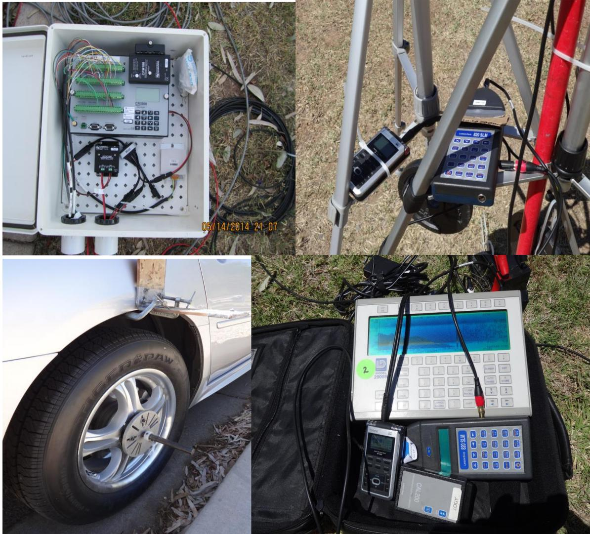
**Figure 17. Images of various equipment: (top left) wall tower data logger box; (top right) microphone equipment on field tripod; (bottom left) partial apparatus for mounting and taking On-Board Sound Intensity measurements; (bottom right) more acoustics equipment.**
