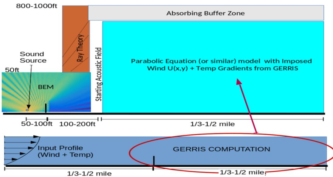
Figure 30. Numerical framework for computing the performance of different barrier designs for different meteorological conditions
