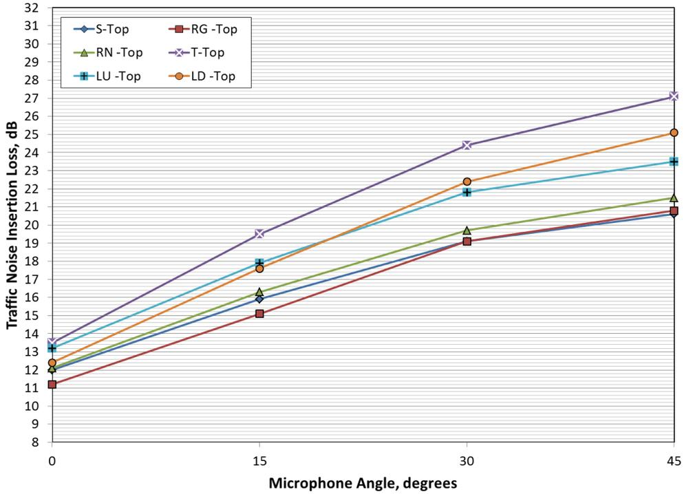
Figure 22. Traffic Noise Insertion Loss Based on Acoustic Scale Modeling Results for a Source Angle of 15° and a Full-Size R distance of 14.8ft (4.5m)
