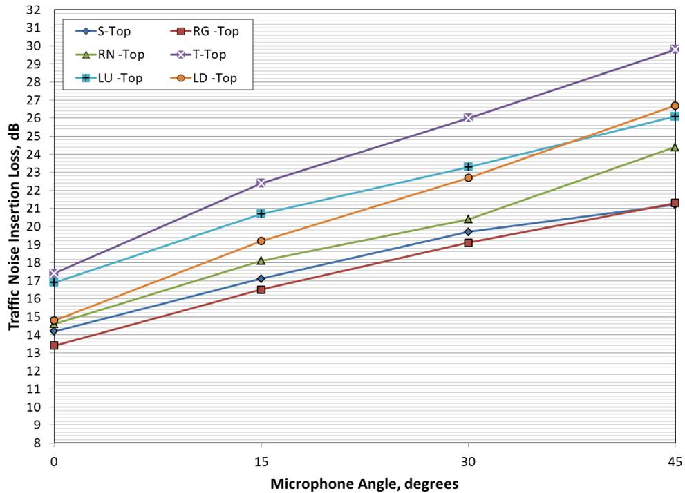
Figure 21. Traffic Noise Insertion Loss Based on Acoustic Scale Modeling Results for a Source Angle of 30° and a Full-Size R distance of 9.8ft (3m)
