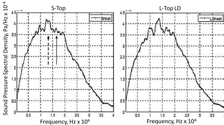
**Figure 17. Frequency Spectra for the Straight (S) Top and L-Top LD Barrier Configurations**
