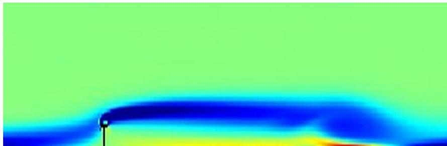
**Figure 28. Computation of mean vorticity around a T-top for wind from left to right using GERRIS CFD code**
