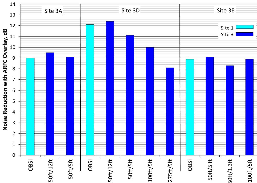
**Figure 7: Comparison of pre- and post-overlay noise reductions for Site 1 OBSI and Site 3 wayside measurements**
