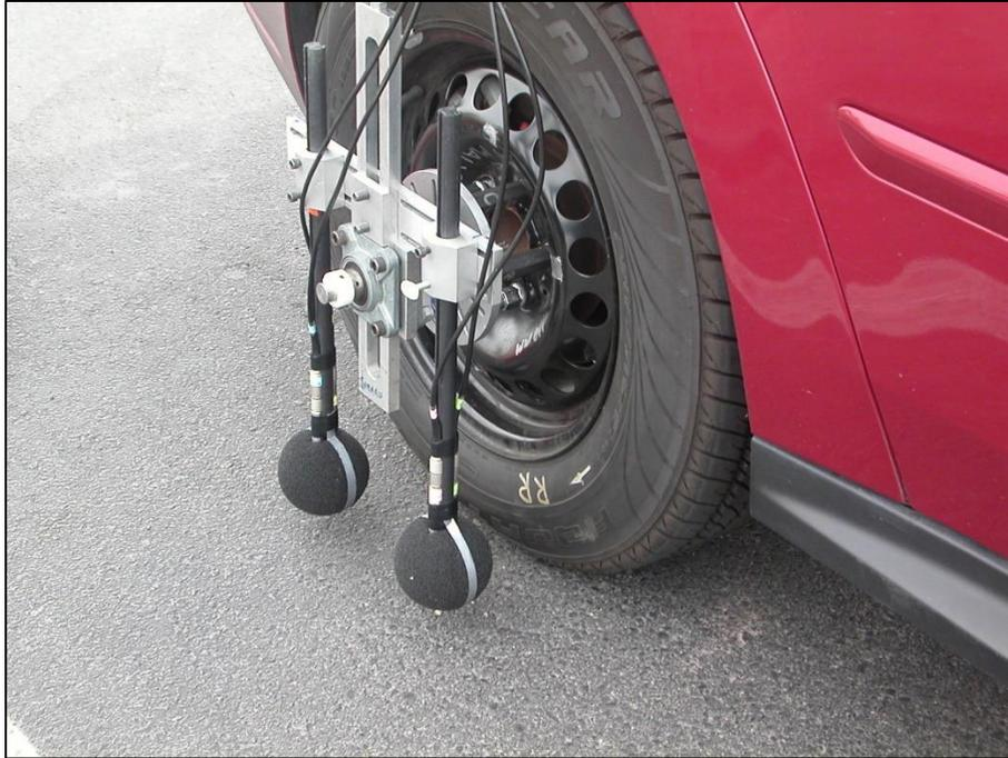
**Figure 5. OBSI Measurement Equipment Setup**
