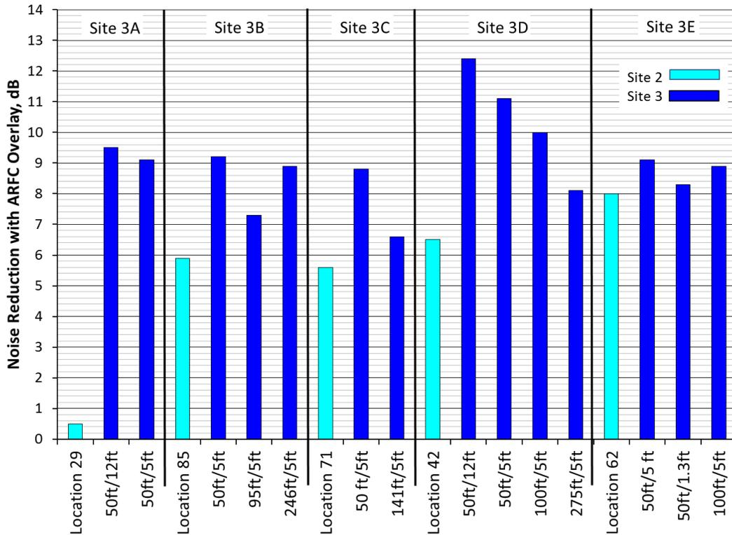
**Figure 6: Comparison of pre- and post-overlay noise reductions for Site 3 measurement locations and nearest Site 2 locations**
