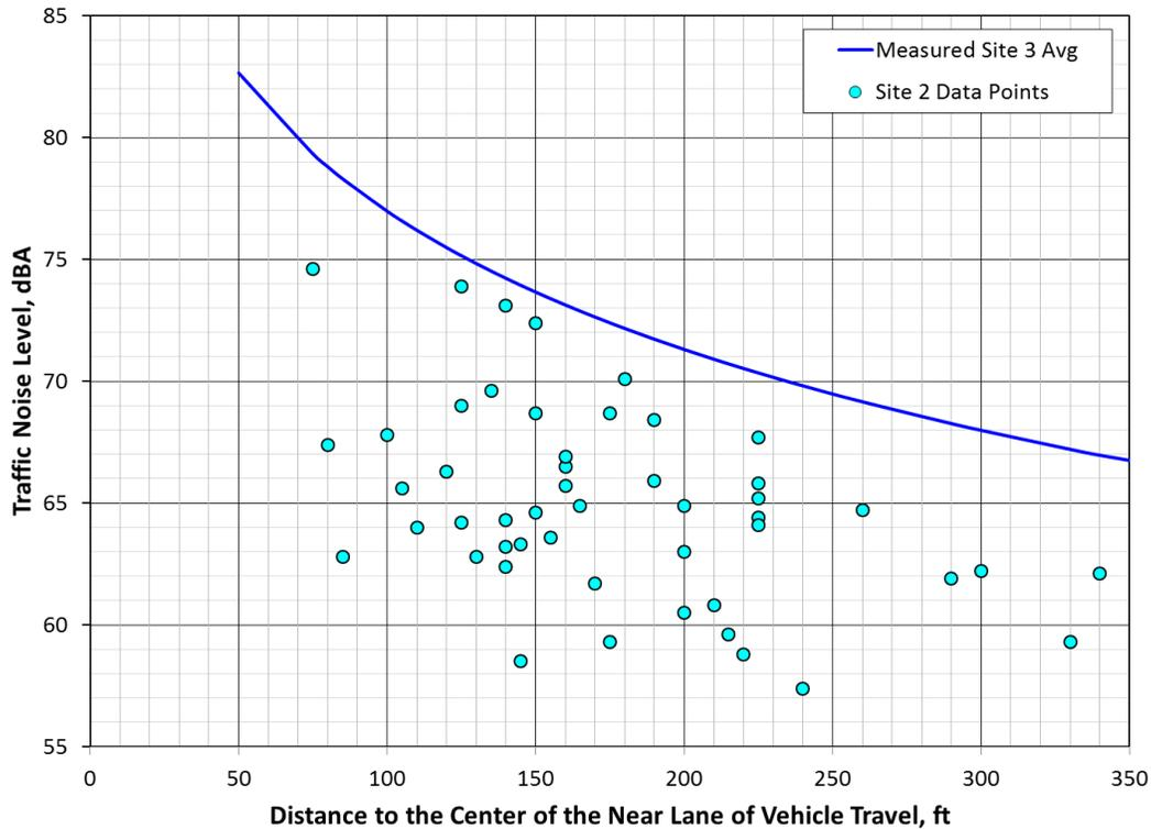
**Figure 15: Site 2 pre-overlay noise levels compared to Site 3 average pre-overlay levels as a function of distance from the roadway**
