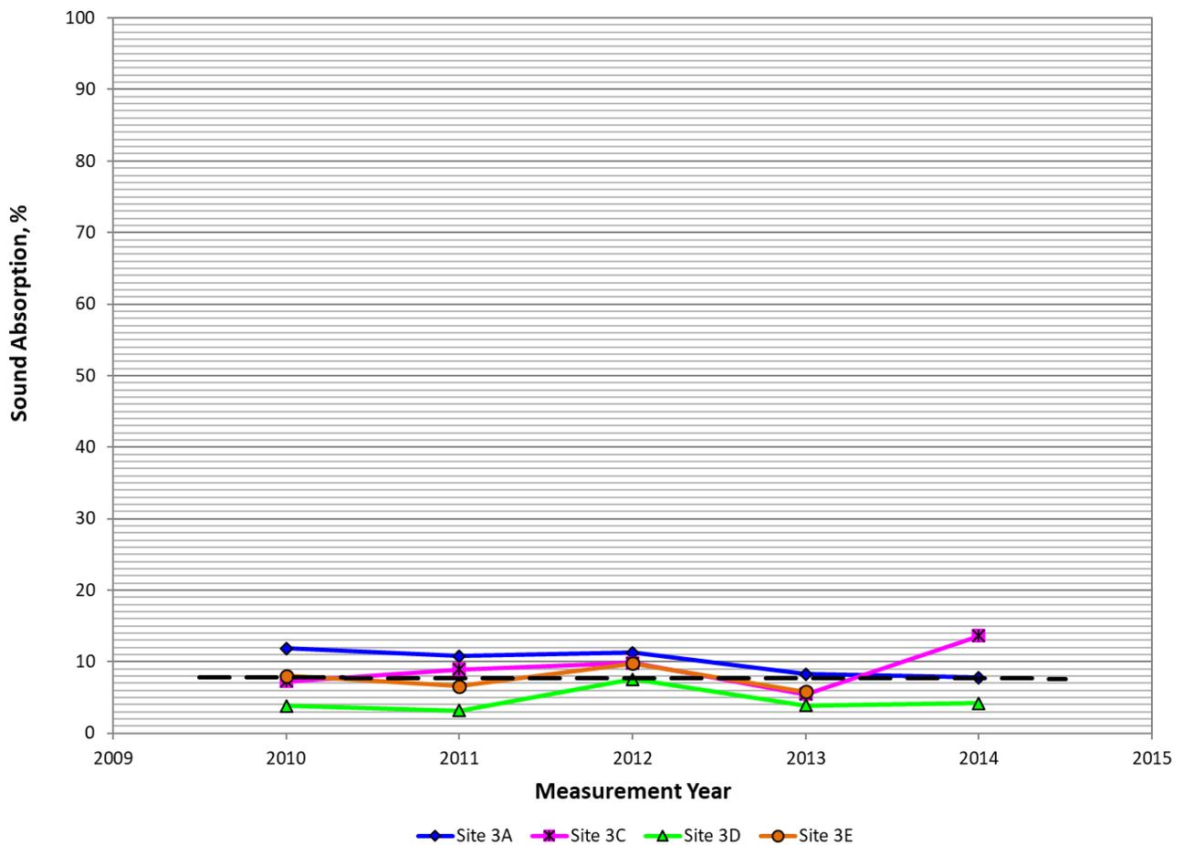
**Figure 32. Overall Average Sound Absorption Percentage for Type 3 Sites for Five Measurement Years**
