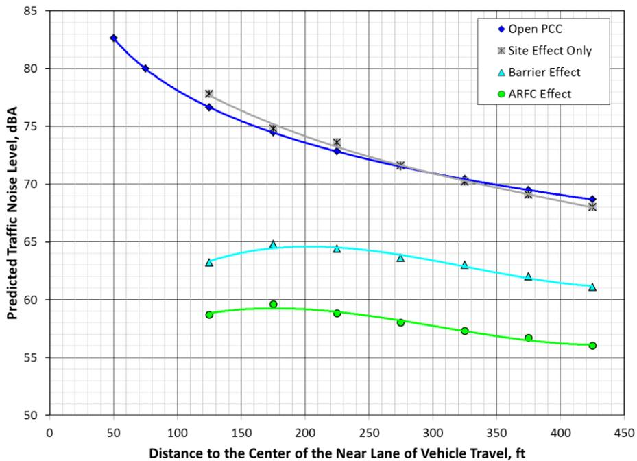
Figure 22: Example of TNM predictions for a flat roadway geometry (site effect), with an added 12 ft barrier 110 ft from the roadway (barrier effect), and with ARFC added (ARFC effect)
