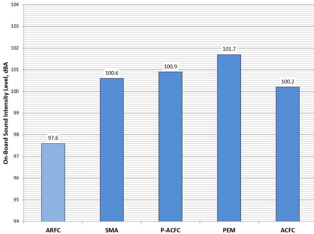
Figure 43. Average Overall Noise Levels for the Initial 2002 Casa Grande Measurement Period
