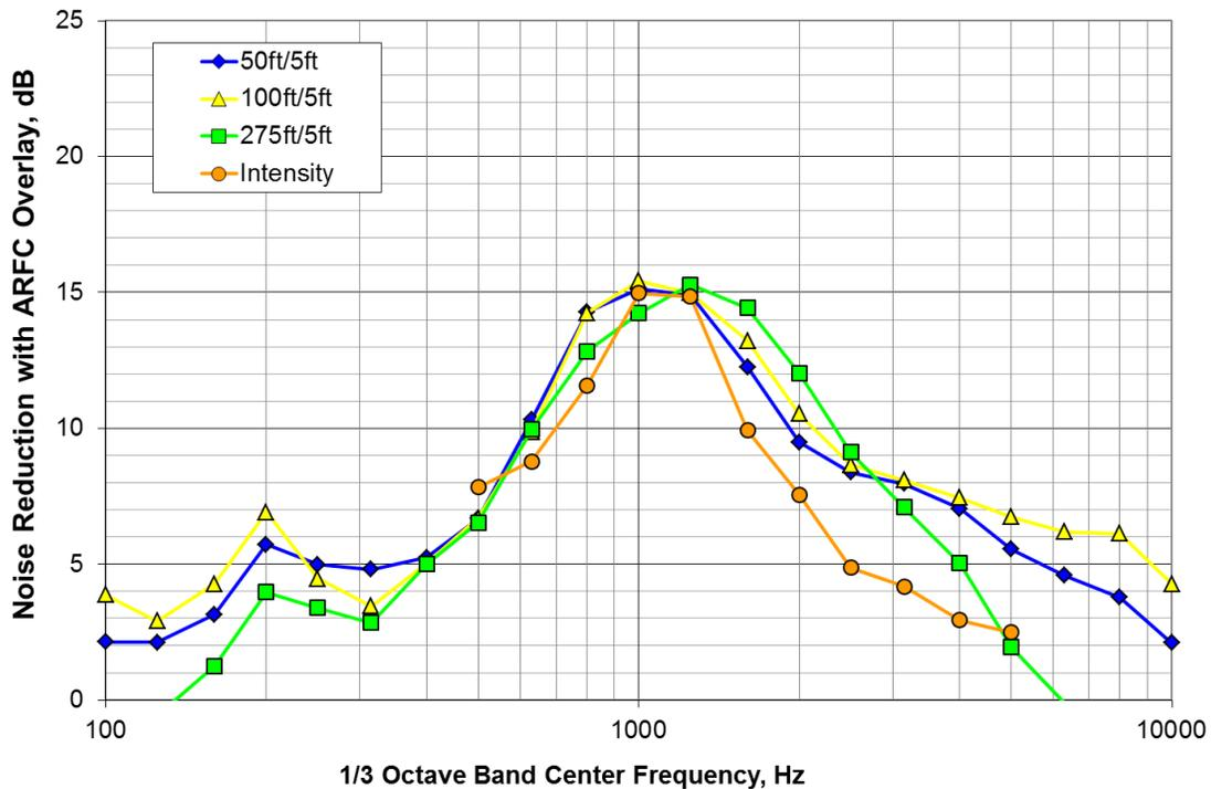
**Figure 8: Comparison of pre- and post-overlay 1/3 octave band noise reduction spectra for Site 1 OBSI and Site 3 wayside measurements**
