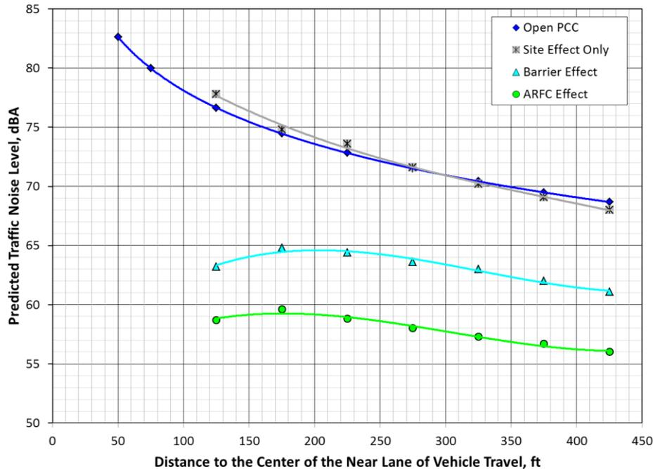
**Figure 23: Example of TNM predictions for a 4 ft elevated roadway (site effect), with an added 3 ft K-rail at the edge of the roadway (barrier effect), and with ARFC added (ARFC effect)**
