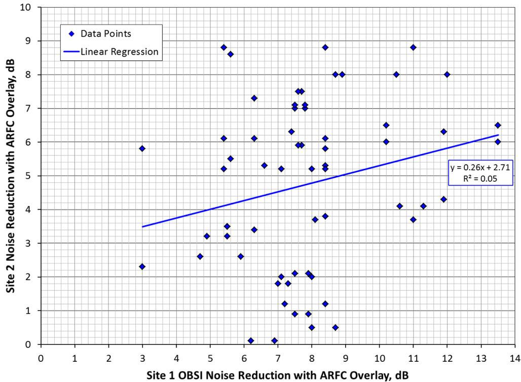
**Figure 5: Linear regression of Site 1 noise reductions versus Site 2 noise reductions**
