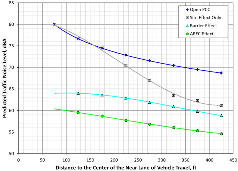
Figure 24: Example of TNM predictions for a roadway recessed 6 ft (site effect), with an added 12 ft barrier 100 ft from the roadway (barrier effect), and with ARFC added (ARFC effect)
