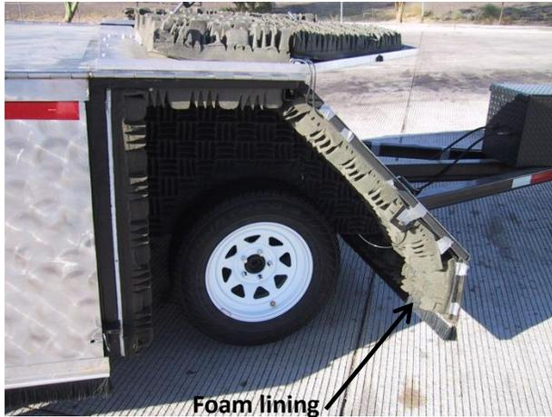
a) CPX Trailer Interior with Closable Panel Fully Opened
