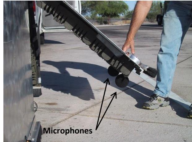
b) CPX Trailer Closable Panel with Microphones Installed
