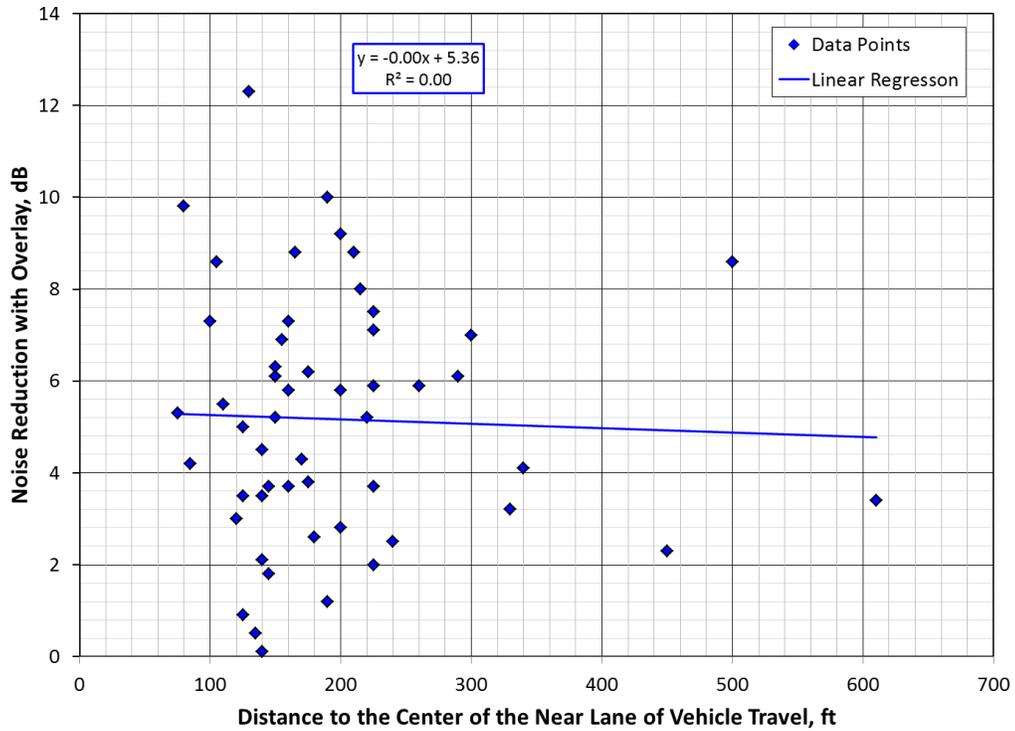
Figure 10: Linear regression of distance to the roadway for Site 2 locations versus noise reduction
