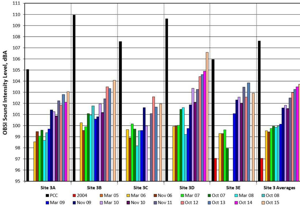
Figure 9. Overall OBSI Levels for Freeway Corridors Pre- and Post-ARFC Overlay
