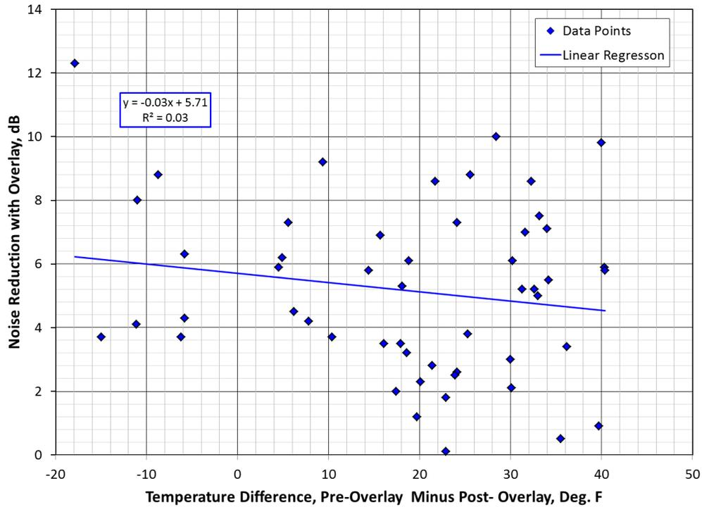
**Figure 13: Linear regression of pre- and post-overlay measurement temperature differences for Site 2 locations versus noise reduction**
