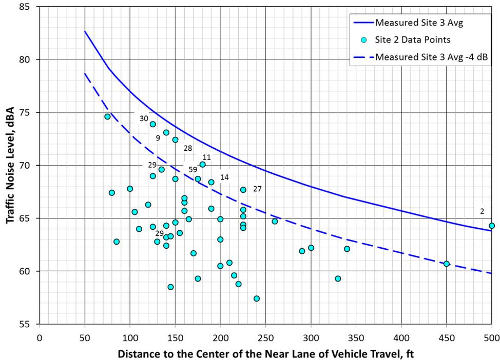
**Figure 29: Site 2 pre-overlay noise levels compared to the measured Site 3 averages and to the Site 3 averages offset 4 dB lower**
