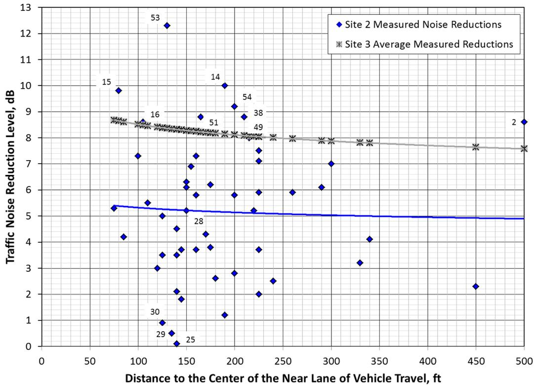
**Figure 27: Measured noise reductions for the Site 2 locations with logarithmic regression compared to the average noise reduction from the Site 3 measurements**
