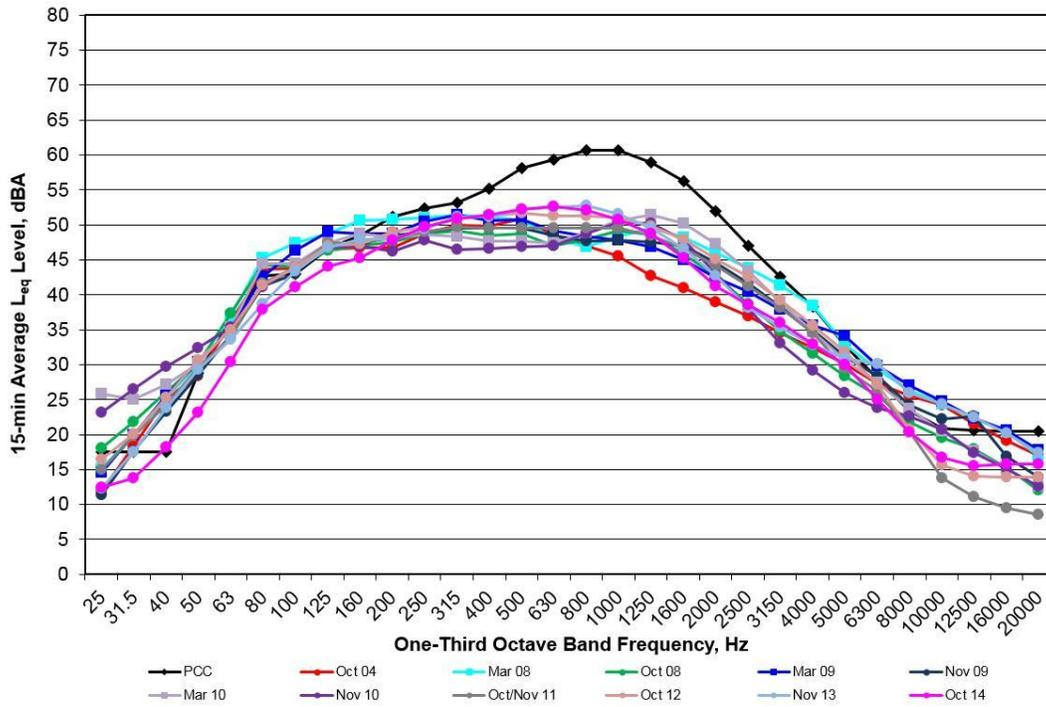
**Figure C22. One-Third Octave Band Spectra for Measured Noise Levels at Site 3D at the 250ft/5ft Microphone for PCC *Pre-Overlay* and *Post-Overlays* in 2004 and 2008 Through 2014**
