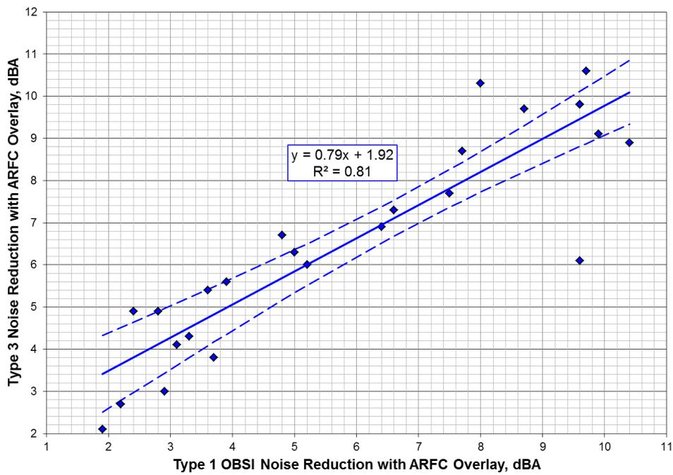
**Figure D7. Linear Regression of Type 3 Noise Reductions at 100 ft Versus Type 1 Noise Reductions for the Entire Project Duration**
