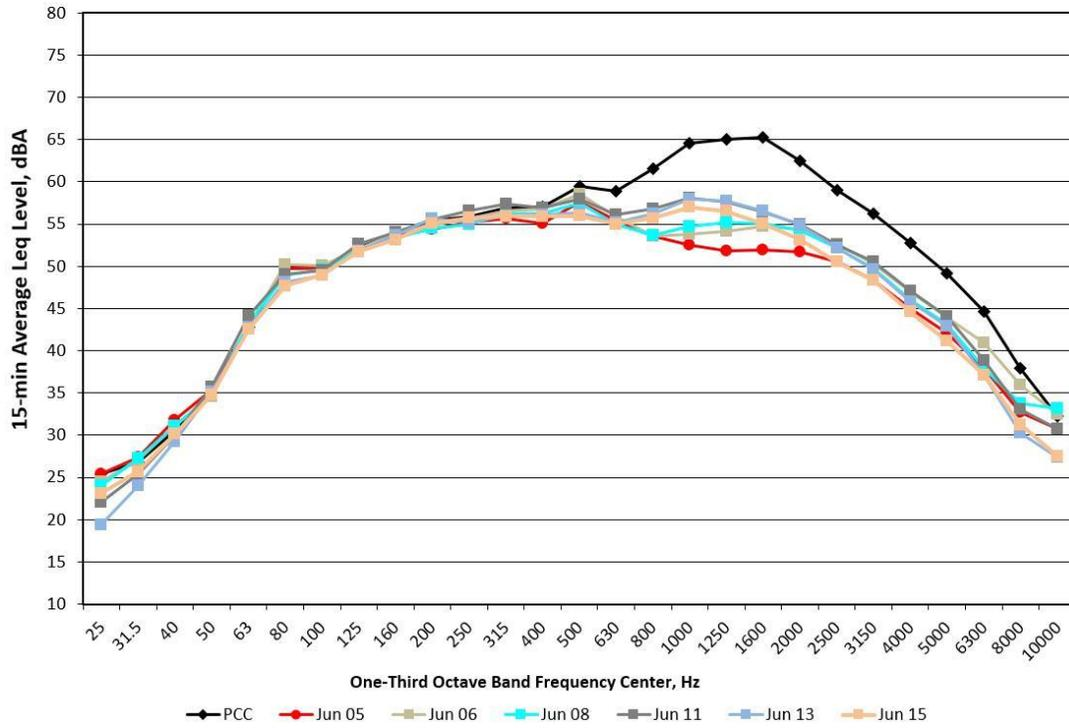
**Figure C15. One-Third Octave Band Spectra for Measured Noise Levels at Site 3C at the 141ft/5ft Microphone for PCC *Pre-Overlay* and *Post-Overlays* in 2005 Through 2015**
