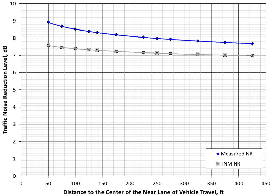
**Figure 20: Comparison of measured and predicted Site 3 wayside level noise reductions as a function of distance from the roadway**
