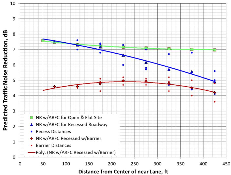
Figure 25: Incremental noise reduction for ARFC added to a flat site, a 6 ft recessed site, and a recessed site with a 12 ft barrier
