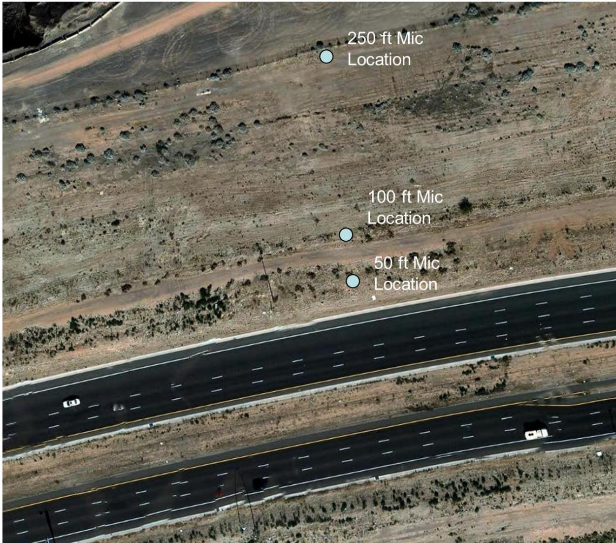
**Figure C16. Aerial Photograph of Site 3D on SR 202 with Microphone Positions Indicated**
