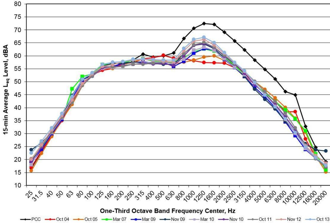
**Figure C27. One-Third Octave Band Spectra for Measured Noise Levels at Site 3E at the 100ft/5ft Microphone for PCC Pre-Overlay and Post-Overlays in 2004 and 2009 Through 2013**
