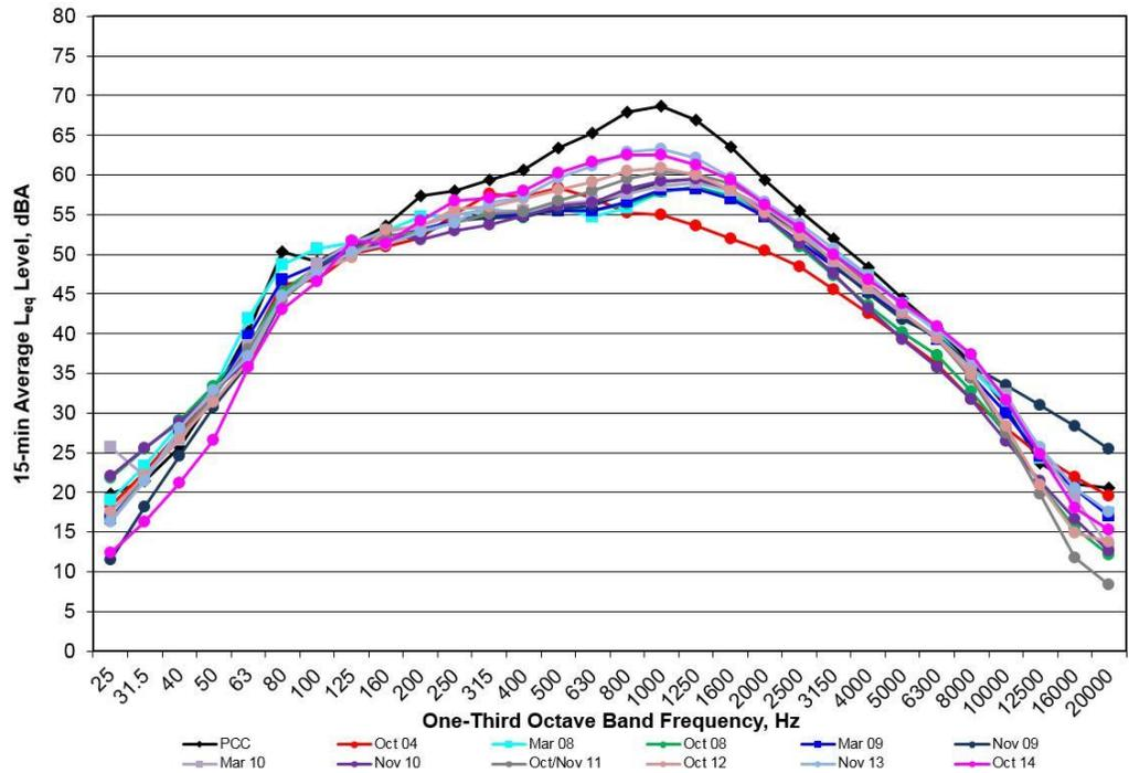
Figure C21. One-Third Octave Band Spectra for Measured Noise Levels at Site 3D at the 100ft/5ft Microphone for PCC Pre-Overlay and Post-Overlays in 2004 and 2008 Through 2014
