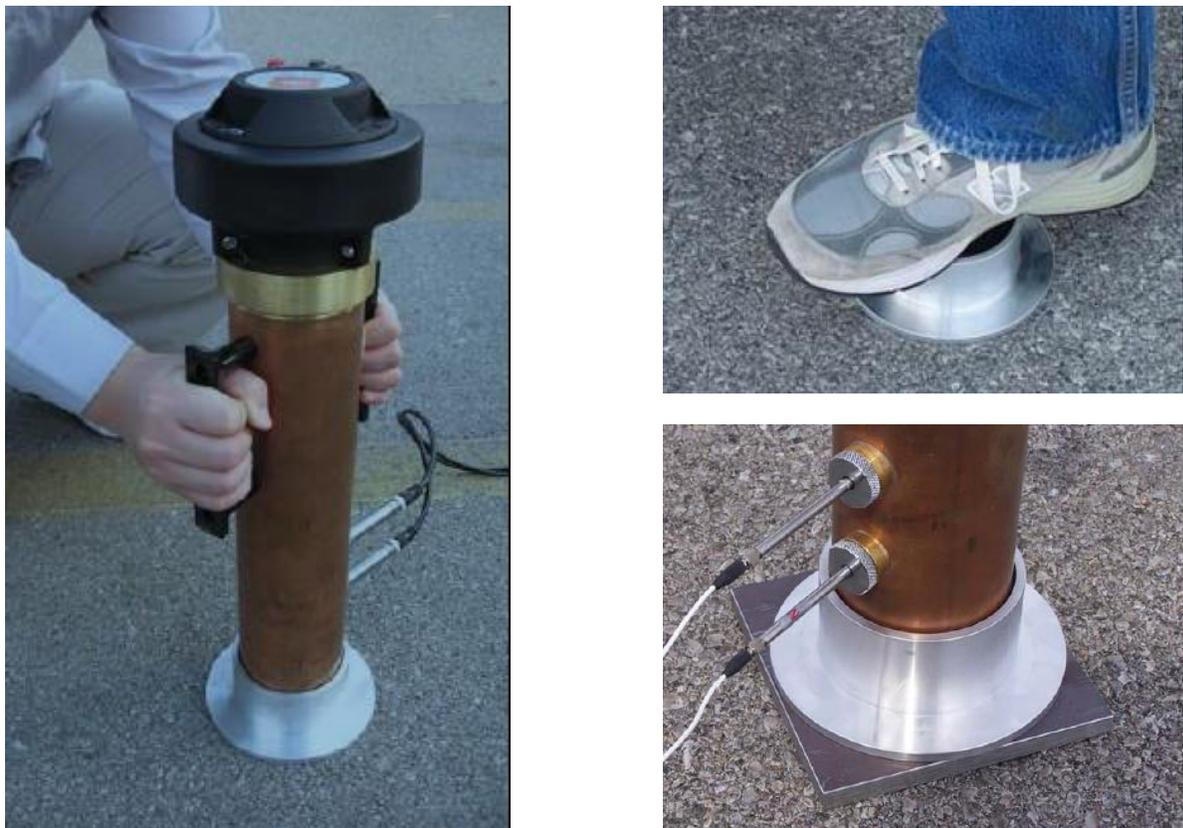
**Figure 31. Impedance Tube Installed on Pavement (Left), Sealing Ring Installed on the Pavement (Top Right), and Steel Plate Inserted Between Pavement and Impedance Tube (Lower Right) (Seybert and Martinus 2009)**
