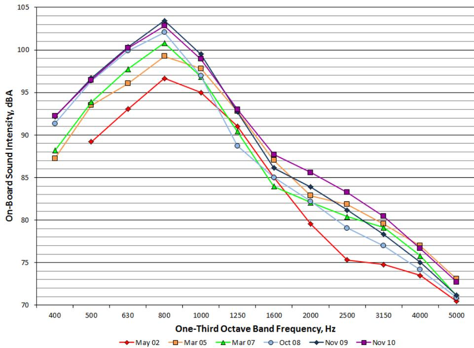
**Figure 49. One-Third Octave Band Spectra for the Casa Grande P-ACFC Section from May 2002 to November 2010**
