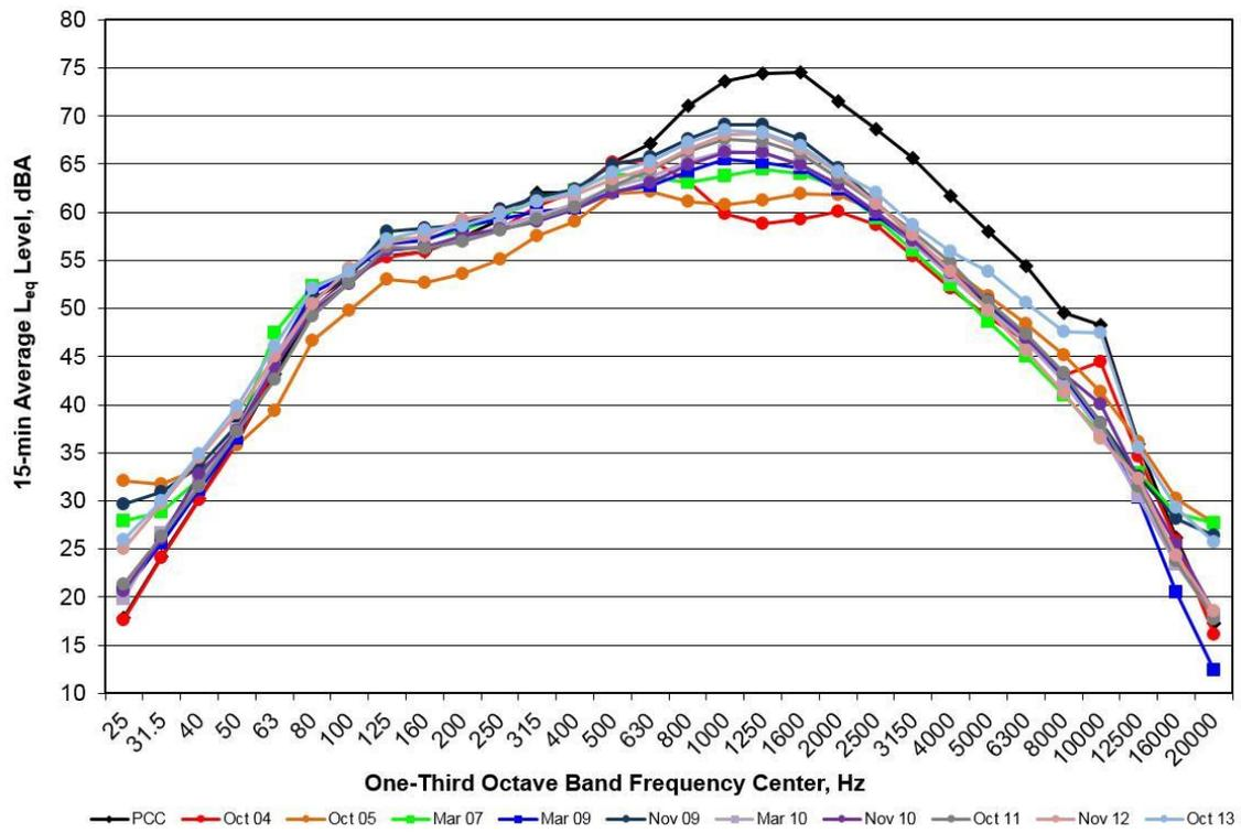
Figure C26. One-Third Octave Band Spectra for Measured Noise Levels at Site 3E at the 50ft/1.3ft Microphone for PCC Pre-Overlay and Post-Overlays in 2004 and 2009 Through 2013
