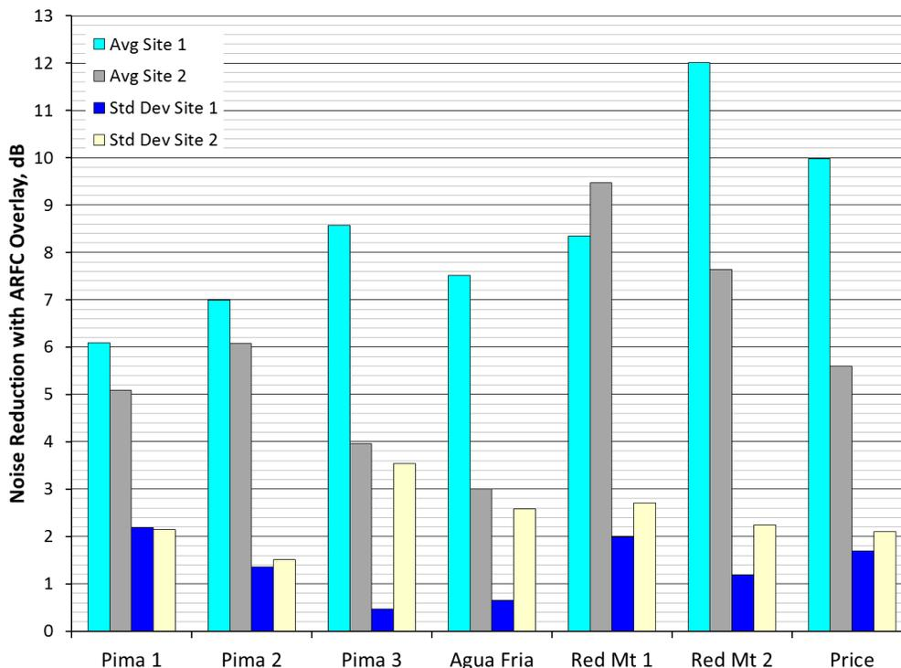
**Figure 4: Averages and standard deviations of Site 1 and 2 noise reductions for different freeway segments**
