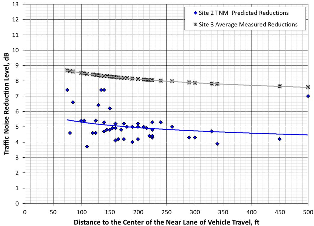
**Figure 26: Predicted noise reductions for the Site 2 locations with logarithmic regression compared to the average noise reduction from the Site 3 measurements**
