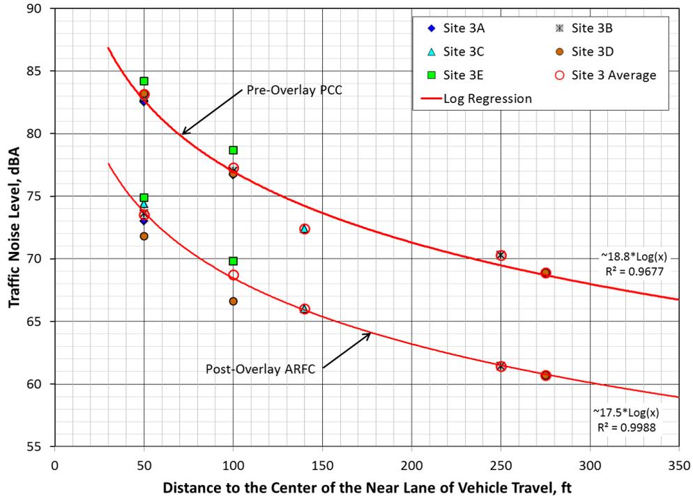
**Figure 14: Logarithmic regression of pre- and post-overlay wayside levels versus distance from the roadway for Site 3 measurement locations**
