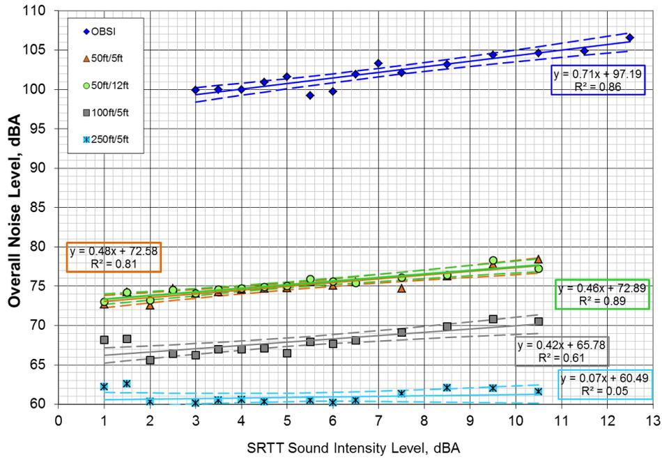
**Figure D4. Overall Levels Versus Age of Overlay for Type 1 and Type 3 Measurements at Site 3D with 95 Percent Confidence Limits of the Regression Line Indicated by Dashed Lines**
