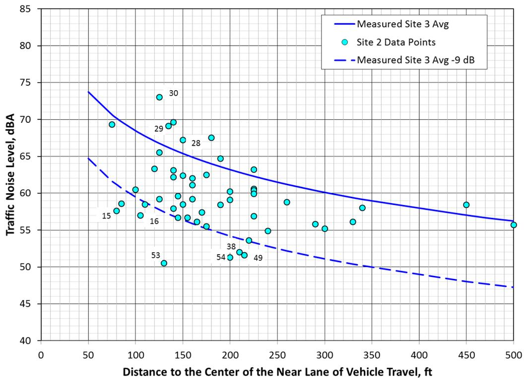
**Figure 28: Site 2 post-overlay noise levels compared to the measured Site 3 averages and to the Site 3 averages offset 9 dB lower**
