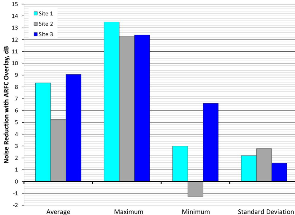
**Figure 2: Comparison of average, maximum, minimum, and standard deviation of noise reductions for Site 1, 2, and 3 measurements**
