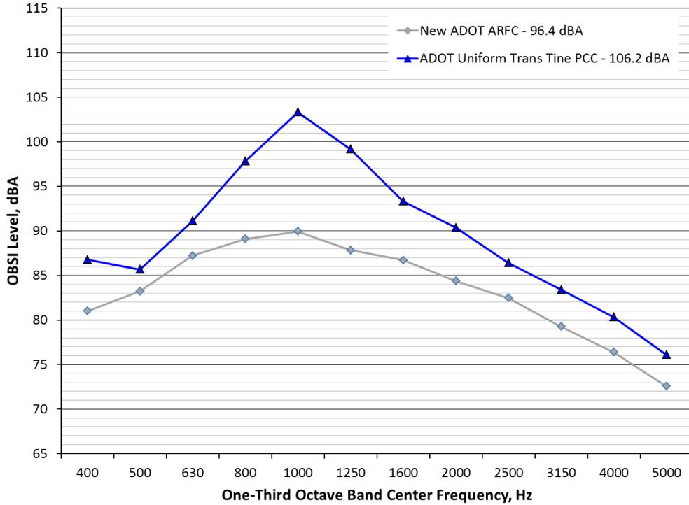
Figure 18: OBSI spectra representing pre-overlay uniform transversely timed PCC and post-overlay ARFC for use in the GLSS modified TNM
