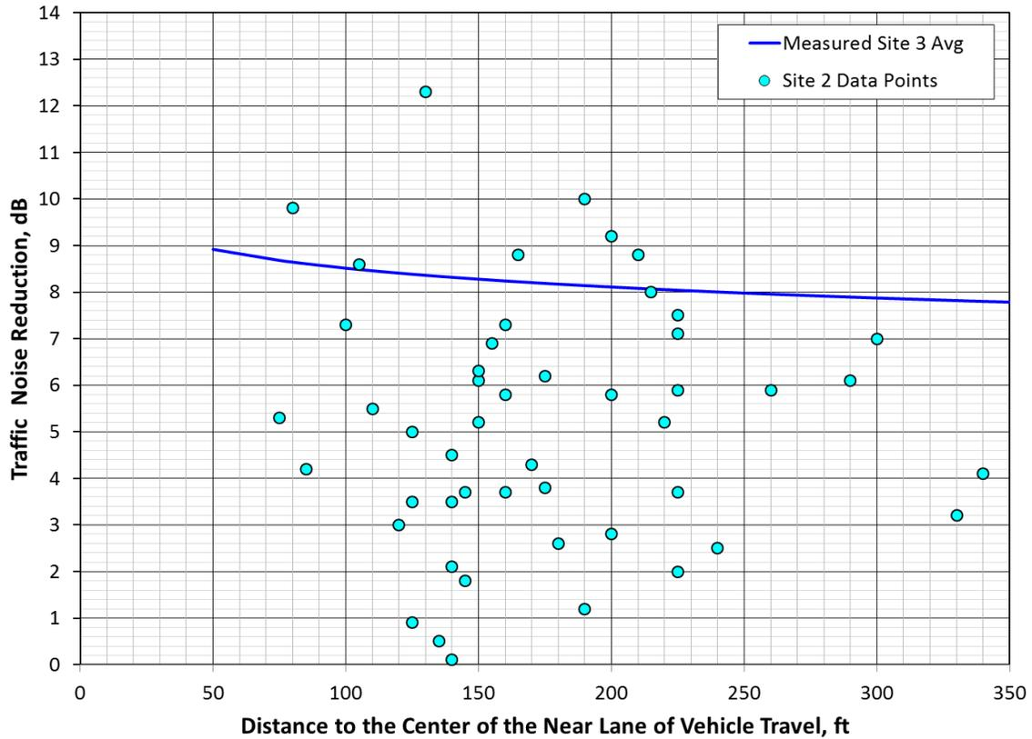
**Figure 17: Site 2 noise reductions compared to Site 3 average noise reductions as a function of distance from the roadway**
