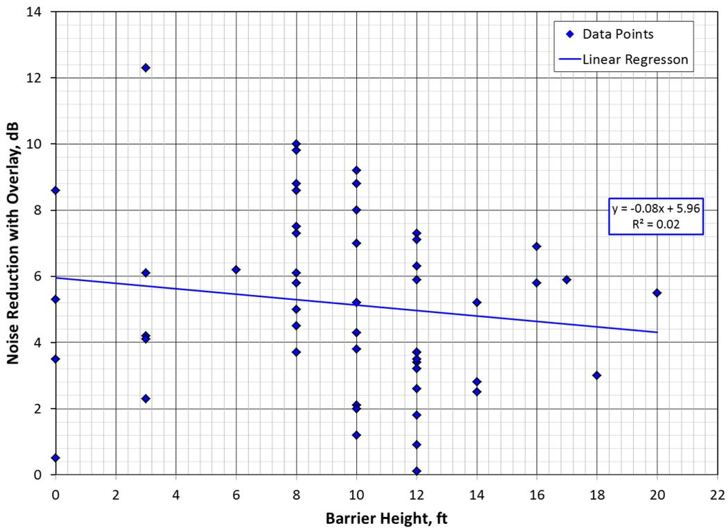
Figure 11: Linear regression of barrier height for Site 2 locations versus noise reduction
