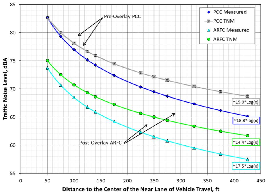
Figure 19: Comparison of measured and predicted Site 3 wayside levels pre- and post-overlay as a function of distance from the roadway
