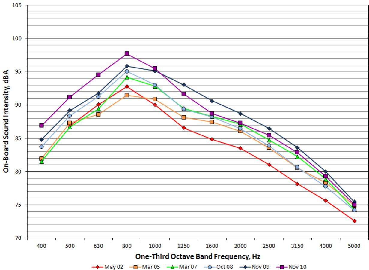
**Figure 47. One-Third Octave Band Spectra for the Casa Grande ARFC Section from May 2002 to November 2010**
