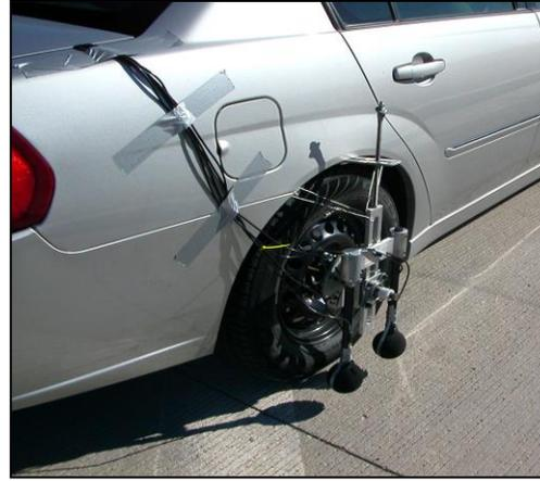
b) OBSI Dual-Probe Fixture Installed on Vehicle for Testing in November 2006
