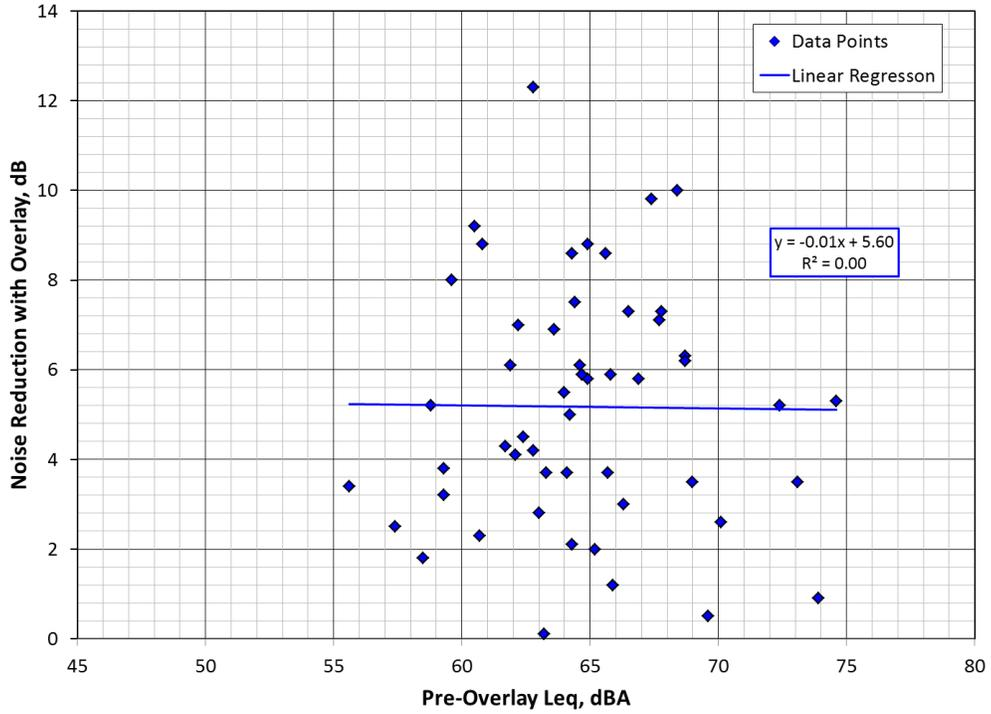
Figure 9: Linear regression Site 2 pre-overlay overall noise levels versus noise reduction
