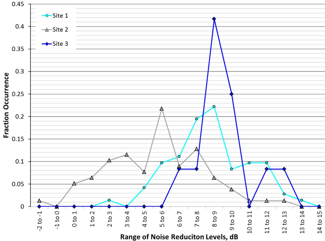
Figure 3: Fractional frequency of occurrence of noise reduction levels for Site 1, 2, and 3 results
