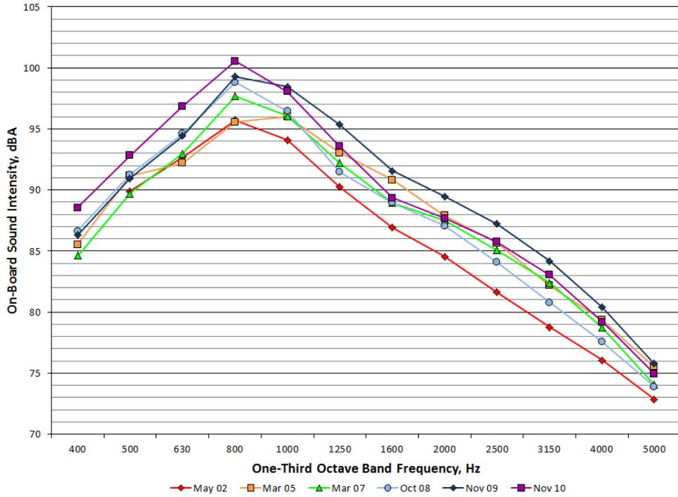
**Figure 48. One-Third Octave Band Spectra for the Casa Grande SMA Section from May 2002 to November 2010**
