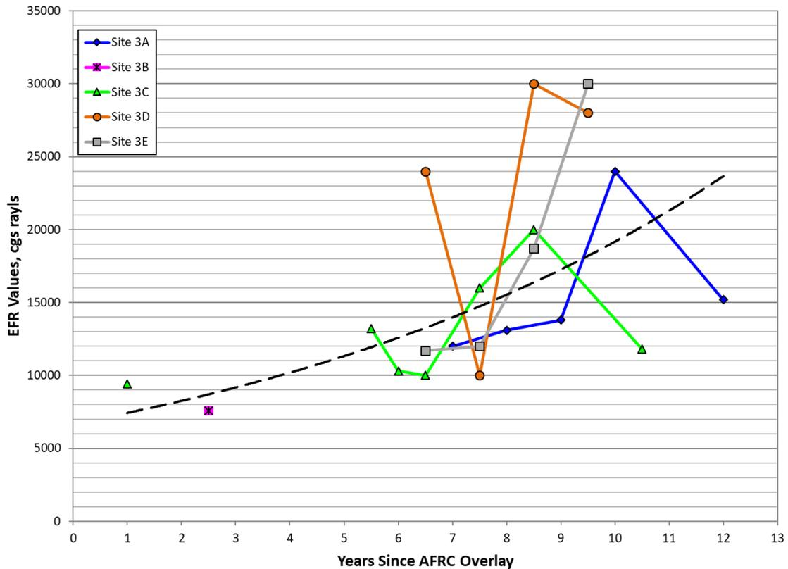
**Figure 30. EFR Values for Type 3 Sites Versus Pavement Age**
