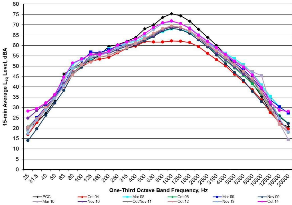
Figure C20. One-Third Octave Band Spectra for Measured Noise Levels at Site 3D at the 50ft/12ft Microphone for PCC Pre-Overlay and Post-Overlays in 2004 and 2008 Through 2014
