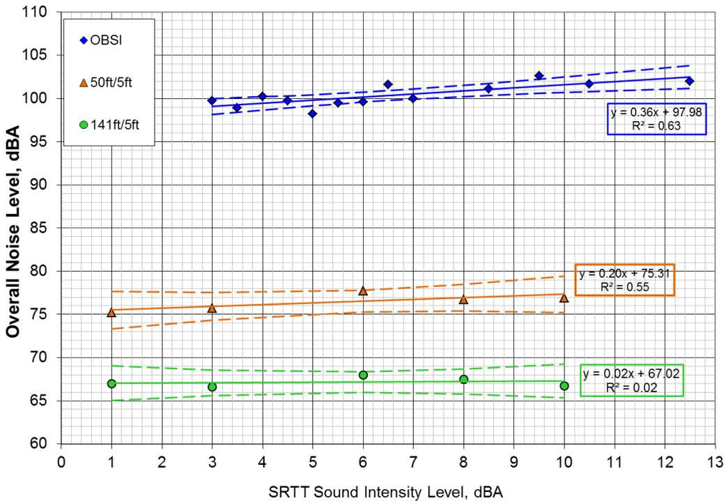
Figure D3. Overall Levels Versus Age of Overlay for Type 1 and Type 3 Measurements at Site 3C with 95 Percent Confidence Limits of the Regression Line Indicated by Dashed Lines
