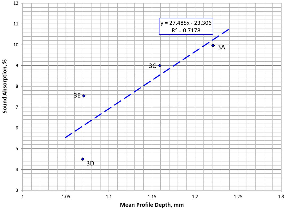
Figure 39. Sound Absorption and MPD Average Values for Sites 3A, 3C, 3D, and 3E
