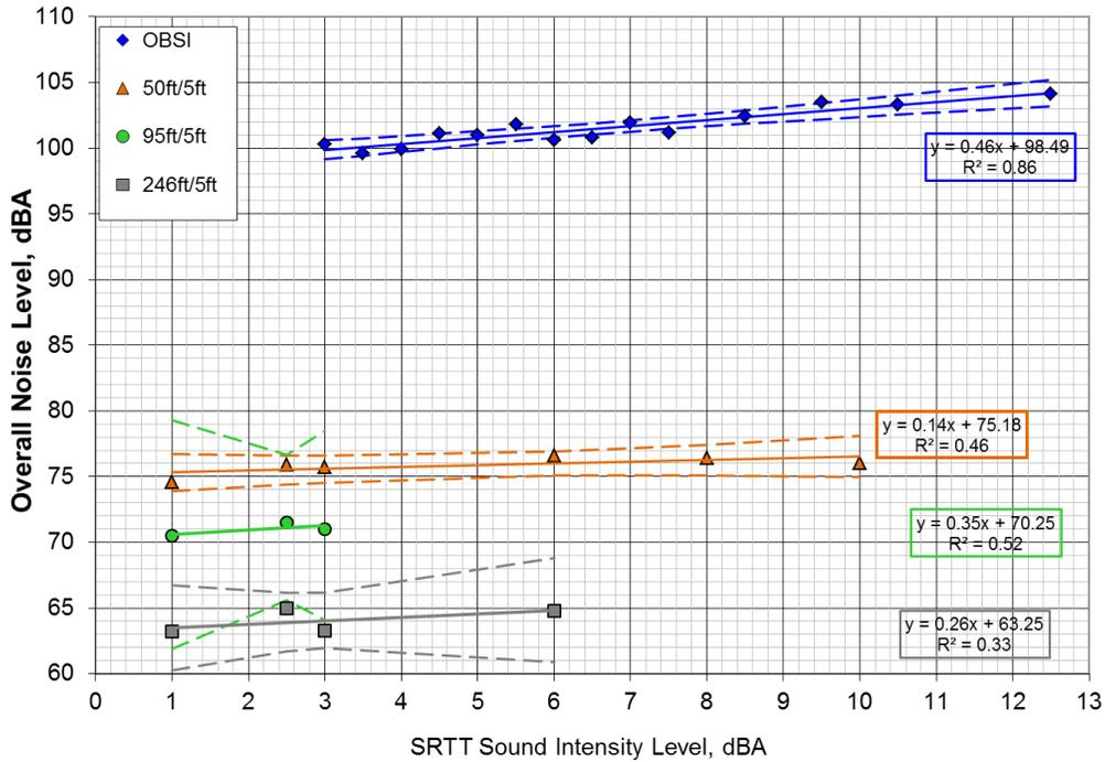
Figure D2. Overall Levels Versus Age of Overlay for Type 1 and Type 3 Measurements at Site 3B with 95 Percent Confidence Limits of the Regression Line Indicated by Dashed Lines
