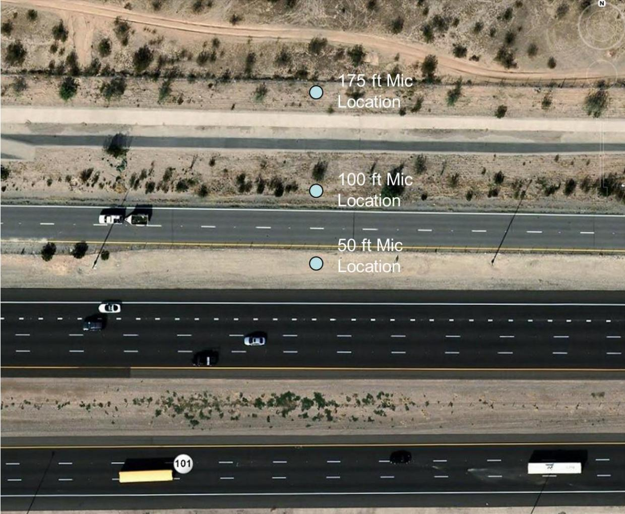
**Figure C1. Aerial Photograph of Site 3A on SR 101 with Microphone Positions Indicated**
