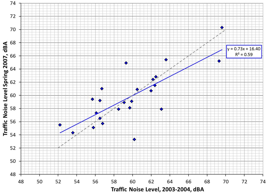
Figure 34: Post-overlay noise levels measured at same Site 2 locations in 2003-2004 and 2007
