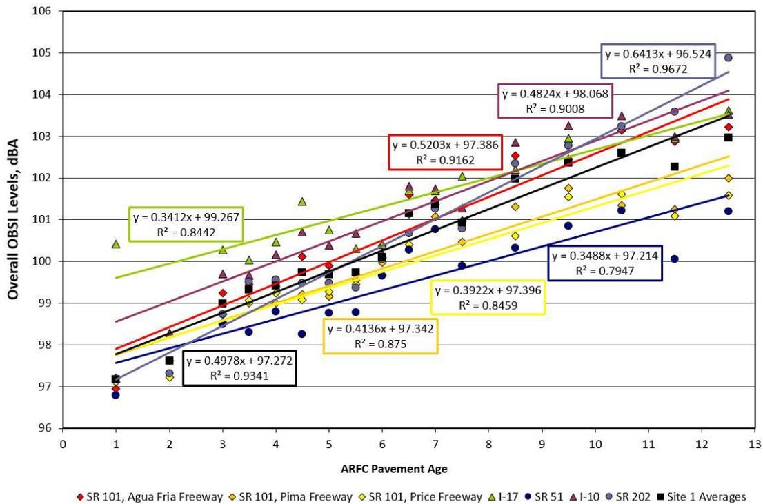
Figure 7. Overall OBSI Levels Versus Age, in Years, of ARFC Overlay
