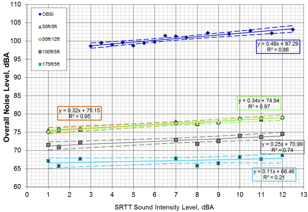
**Figure D1. Overall Levels Versus Age of Overlay for Type 1 and Type 3 Measurements at Site 3A with 95 Percent Confidence Limits of the Regression Line Indicated by Dashed Lines**
