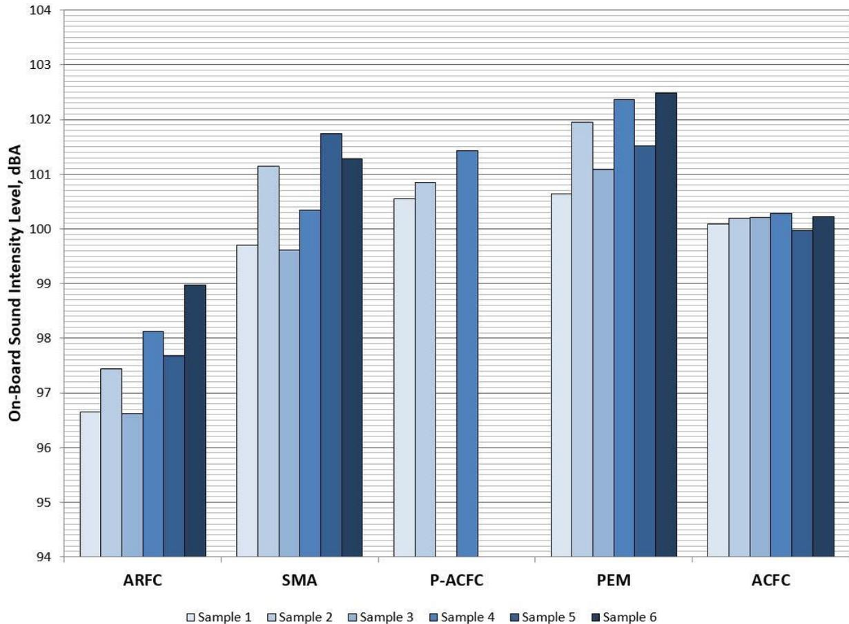
**Figure 42. Overall OBSI Noise Levels for the Initial 2002 Casa Grande Measurement Period**
