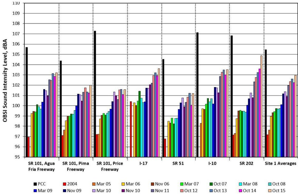
Figure 6. Milepost-Averaged OBSI Levels for Freeway Corridors Pre- and Post-ARFC Overlay
