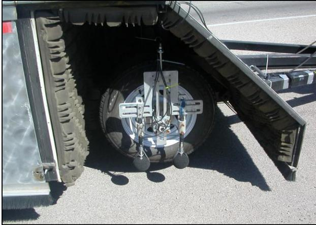
a) OBSI Dual-Probe Fixture Installed on ADOT CPX Trailer for Comparative Testing in March 2005
