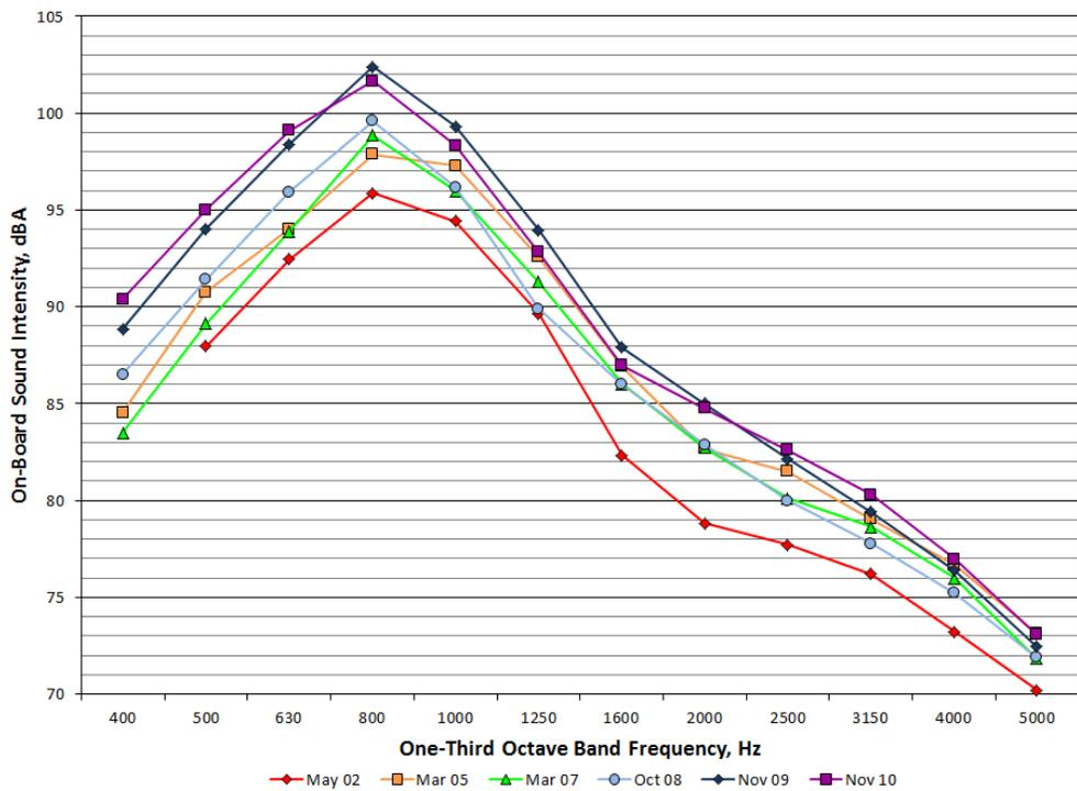
**Figure 51. One-Third Octave Band Spectra for the Casa Grande ACFC Section from May 2002 to November 2010**
