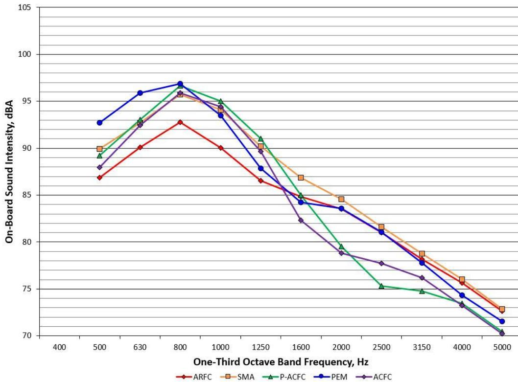
Figure 44. One-Third Octave Band Spectra for the Casa Grande Sections in May 2002
