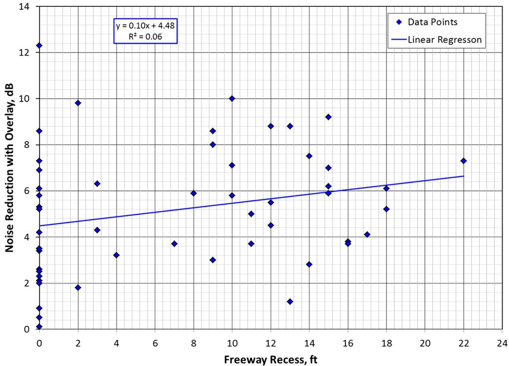
**Figure 12: Linear regression of the depth of roadway recesses for Site 2 locations versus noise reduction**
