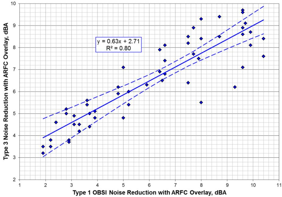
**Figure D6. Linear Regression of Type 3 Noise Reductions at 50 ft Versus Type 1 Noise Reductions for the Entire Project Duration**
