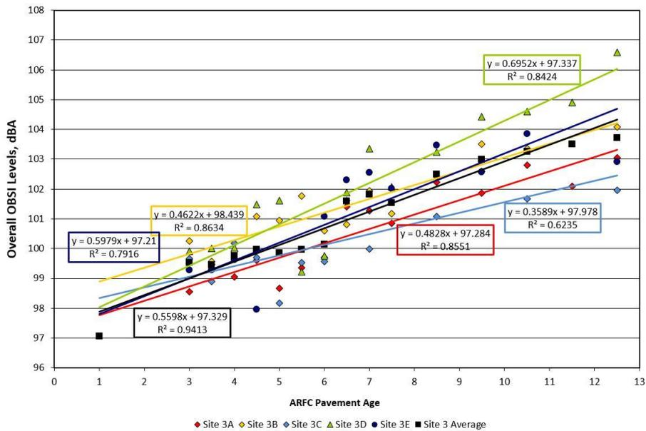
Figure 10. Overall OBSI Levels at Type 3 Sites Versus Age, in Years, of ARFC Overlay
