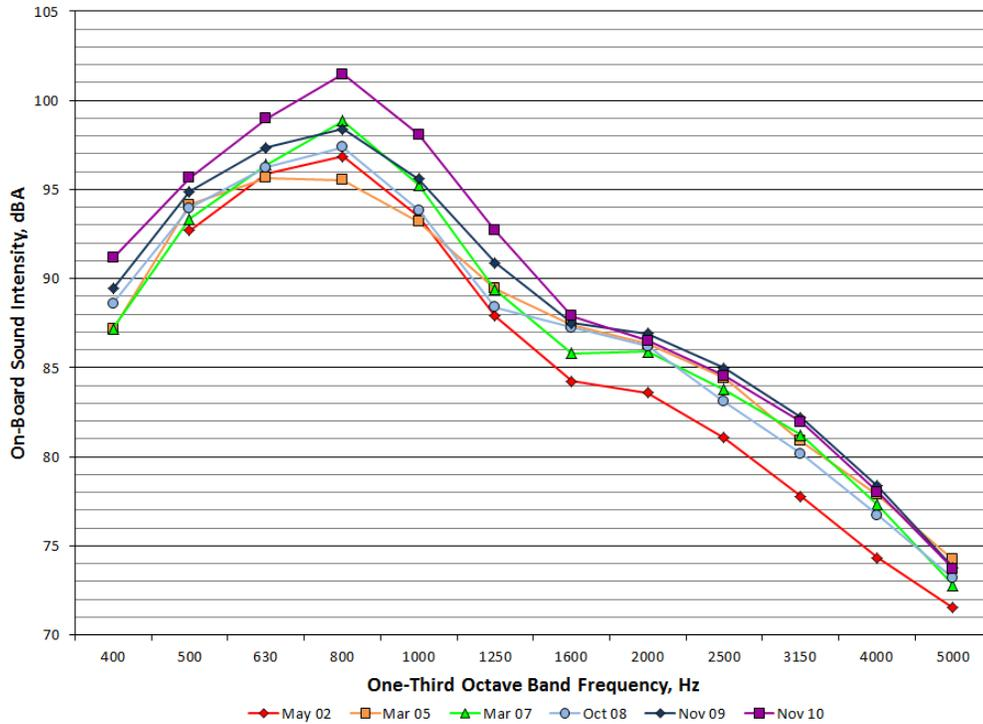
**Figure 50. One-Third Octave Band Spectra for the Casa Grande PEM Section from May 2002 to November 2010**
