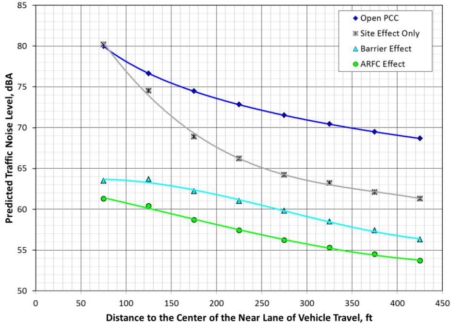
Figure 21: Example of TNM predictions for a roadway recessed 12 ft (site effect), with an added 12 ft barrier 70 ft from the roadway (barrier effect), and with ARFC added (ARFC effect)
