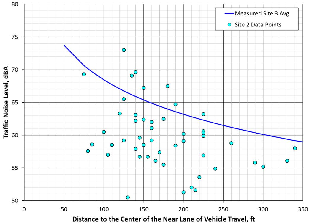
**Figure 16: Site 2 post-overlay noise levels compared to Site 3 average post-overlay levels as a function of distance from the roadway**
