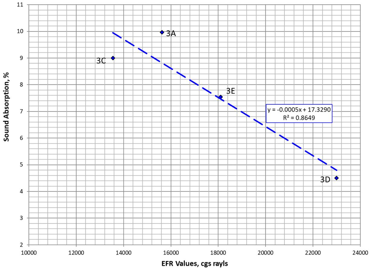
**Figure 38. Sound Absorption and EFR Average Values for Sites 3A, 3C, 3D, and 3E**
