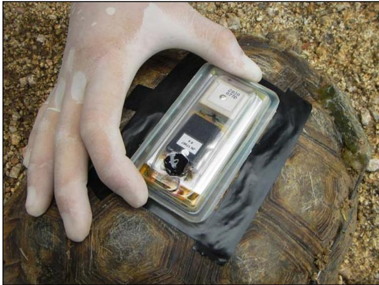
**Figure 12. Sirtrack MicroGPS Tracking Unit Being Applied to a Desert Tortoise in the US 93 Study.**
