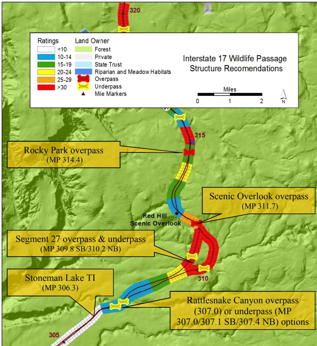
**Figure 33. Potential I-17 Passage Structures Evaluated South of the Red Hill Scenic Overlook between MP 306 and MP 312.**
