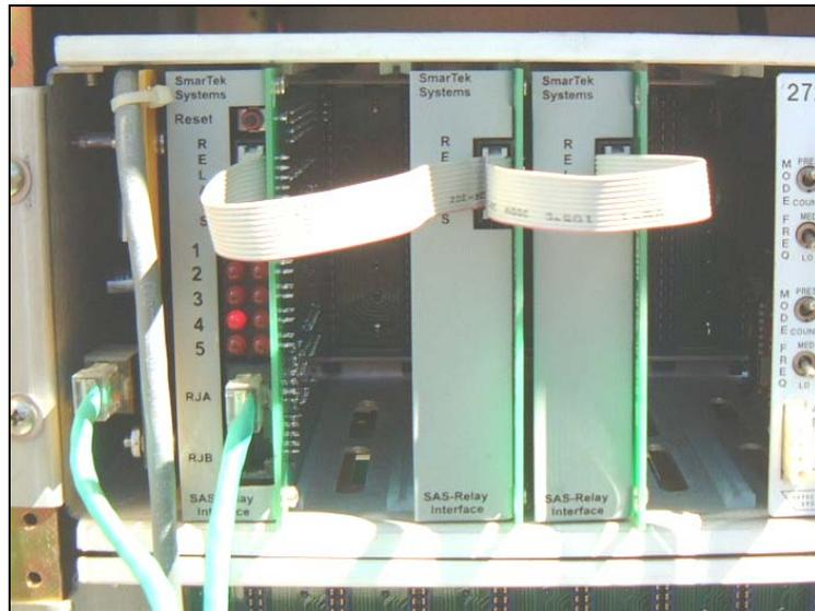
**Figure 3: SmarTek SAS-1 Contact-closure Cards**
