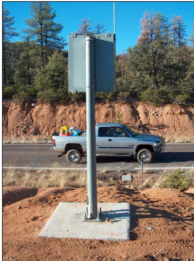
Figure 8.1. Permanent traffic counting station installed along the Little Green Valley section of State Route 260, Arizona, in December 2003. Traffic volume, speed and vehicle type are measured by induction loops cut into the pavement.
