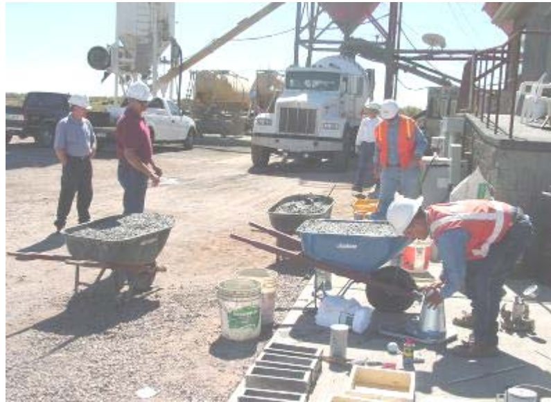
Figure 7. Testing HPC Trial Batches at the Ready Mix
