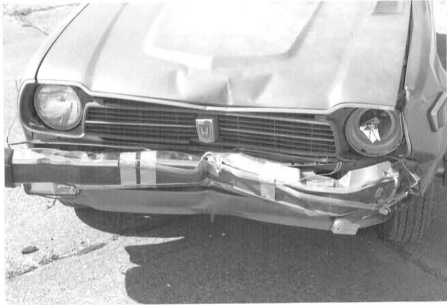
FIGURE 7.21. VEHICLE DAMAGE FOLLOWING TEST 7024-27.
