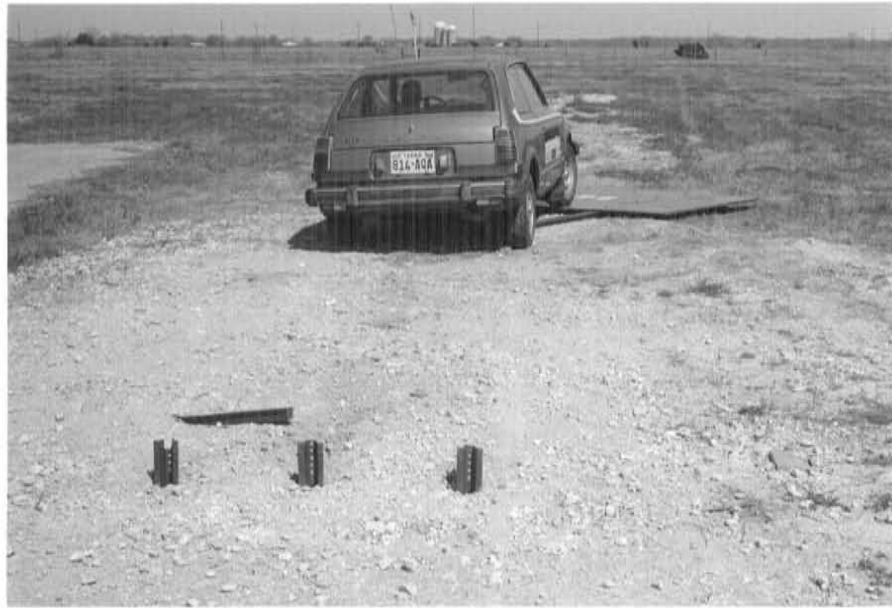
FIGURE 7.14. VEHICLE RESTING POSITION FOLLOWING TEST 7024-24.
