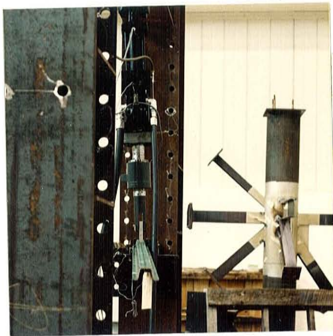
FIGURE 5.11. PHOTOGRAPH OF 18 INCH LATERAL TIP DEFLECTION MEASURED DURING A FACE TO FACE TEST IN THE NON-CRITICAL CONFIGURATION.
