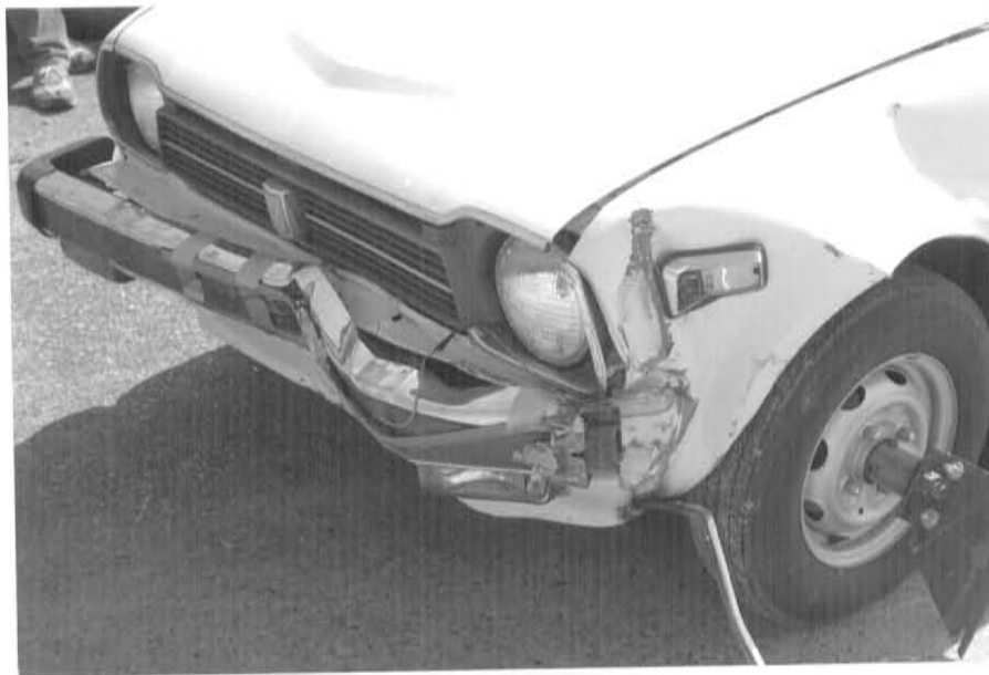
FIGURE 7.5. VEHICLE DAMAGE FOLLOWING TEST 7024-24.
